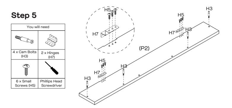
Attach 4 x Cam Bolts (H3) to Top Panel (P2) by tightening with the Phillips Head Screwdriver. Attach 2 x Hinges (H7) to Top Panel (P2) with 6 x Small Screws (H5) by tightening with the Phillips Head Screwdriver.
