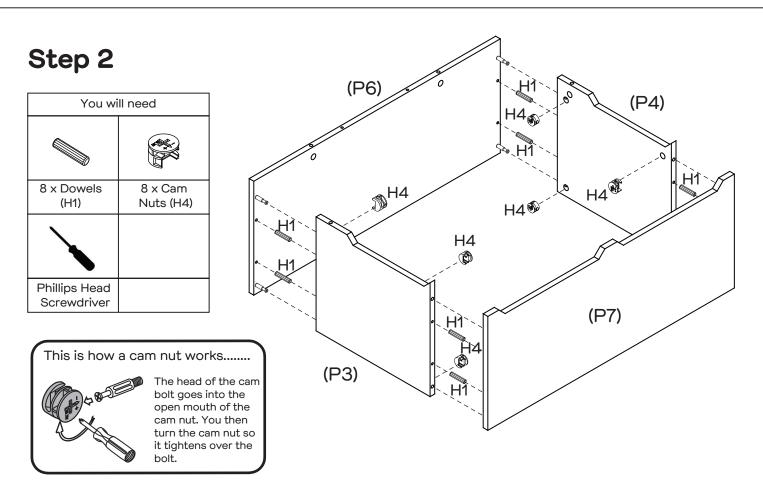
Insert 8 x Cam Nuts (H4) and 8 x Dowels (H1) into Left & Right Side Panels (P3 & P4) as shown. Rotate the cam nuts so the arrows point towards the incoming cam bolts. Attach Front Panel (P7) and Back Panel (P6) to Left & Right Side Panels (P3 & P4) by tightening all cam nuts with the Phillips Head Screwdriver.
