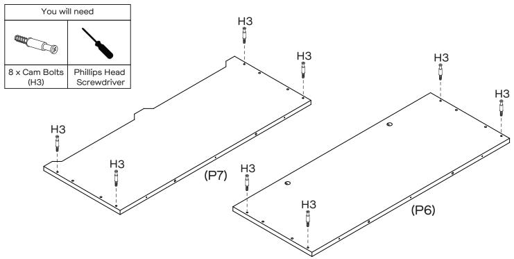
Attach 8 x Cam Bolts (H3) to Front Panel (P7) and Back Panel (P6) by tightening with the Phillips Head Screwdriver.
