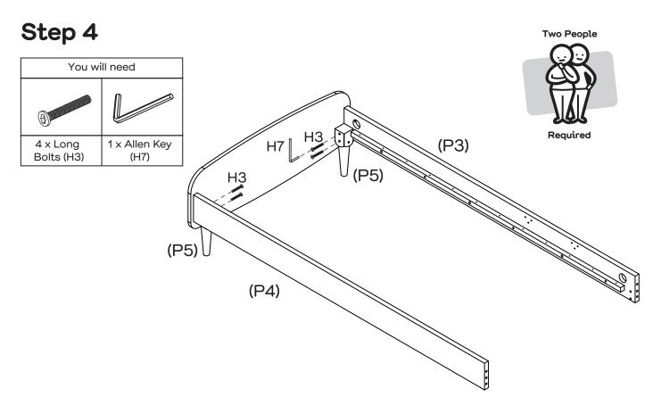
Attach 2 x Legs (P5) to the Left and Right Side Rails (P3 & P4) with 4 x Long Bolts (H3) by tightening at 80 percent with an Allen Key (H7), keep a little loose on this step.
