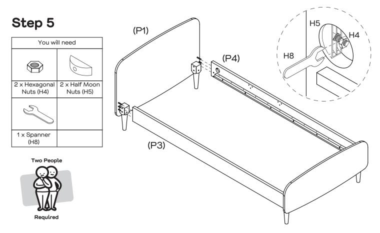
Attach the Headboard (P1) to the Left and Right Side Rails (P3 & P4) with 2 x Half Moon Nuts (H5), and 2 x Hexagonal Nuts (H4) using a Spanner (H8).
