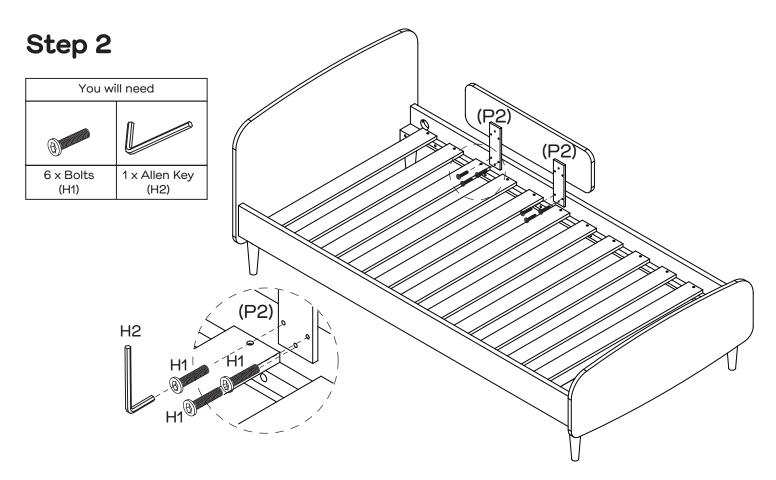
Attach 2  $\times$  Brackets (P2) to either the Right Side Rail (P4) or Left Side Rail (P3) of Pod Bed Single with 6  $\times$  Bolts (H1) by tightening with 1  $\times$  Allen Key (H2).
