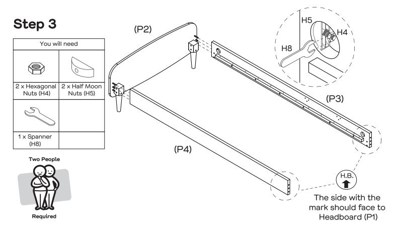
Attach the Footboard (P2) to the Left Side Rail (P3) with 1 x Half Moon Nut (H5) and 1 x Hexagonal Nut (H4) using a Spanner (H8) as shown. Repeat this process for the Right Side Rail (P4).
