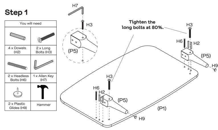
Attach 2 x Plastic Glides (H9) to Legs (P5) with the Hammer. Insert  $4 \times 1$  Dowels (H2) into the Headboard (P1). Attach 2 x Headless Bolts (H6) into the Headboard (P1) by rotating clockwise. Attach 2 x Legs (P5) to the Headboard (P1) with 2 x Long Bolts (H3) by tightening at 80 percent with an Allen Key (H7), keep a little loose on this step.
