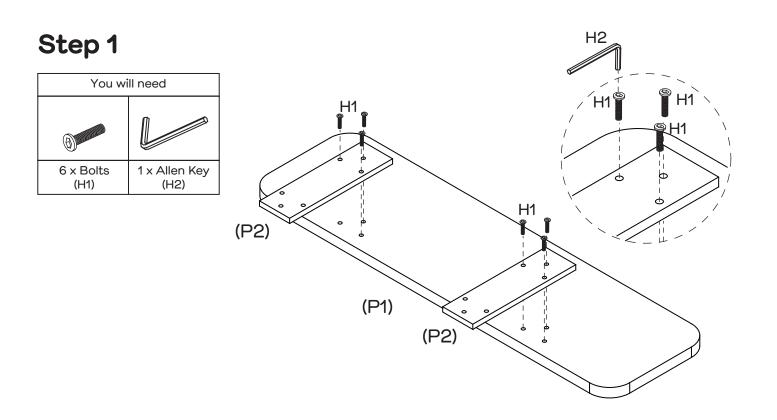
Attach 2 x Brackets (P2) to Panel (P1) with 6 x Bolts (H1) by tightening with 1 x Allen Key (H2).
