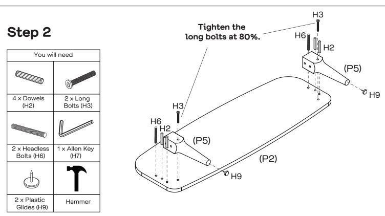
Attach 2 x Plastic Glides (H9) to Legs (P5) with the Hammer. Insert 4 x Dowels (H2) into the Footboard (P2). Attach 2 x Headless Bolts (H6) into the Footboard (P2) by rotating clockwise. Attach 2 x Legs (P5) to the Footboard (P2) with 2 x Long Bolts (H3) by tightening at 80 percent with an Allen Key (H7), keep a little loose on this step.
