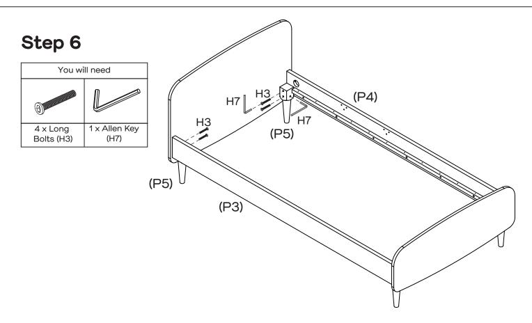
Attach 2 x Legs (P5) to the Left and Right Side Rails (P3 & P4) with 4 x Long Bolts (H3) by tightening with an Allen Key (H7). Make sure the inner space of the bed is square. Ensure to fully tighten all bolts (H3) for attaching legs (P5) with the Allen Key (H7).
