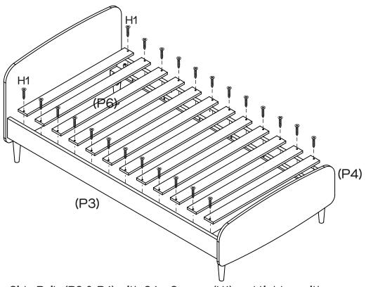
Attach 12  $\times$  Slats (P6) to the Side Rails (P3 & P4) with 24  $\times$  Screws (H1) and tighten with a Phillips head screwdriver.
