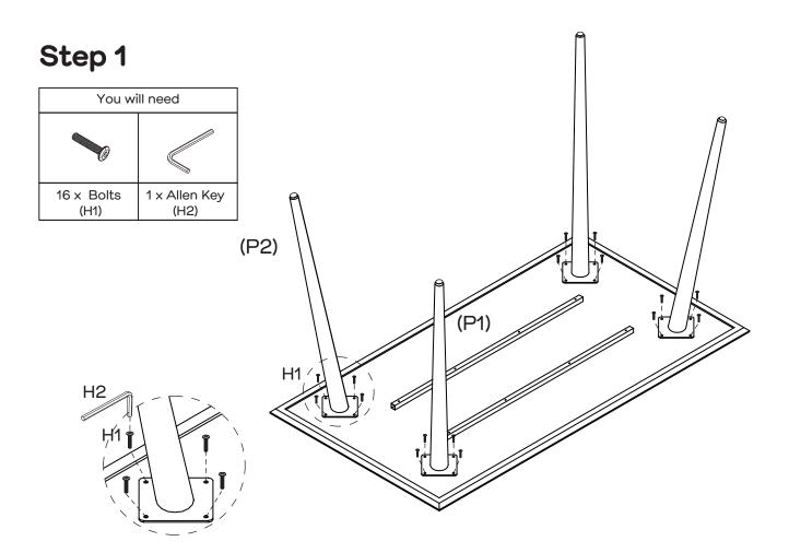
Attach 4 x Legs (P2) to Top Panel (P1) and secure with 16 x Bolts (H1). Tighten with an Allen Key (H2).
