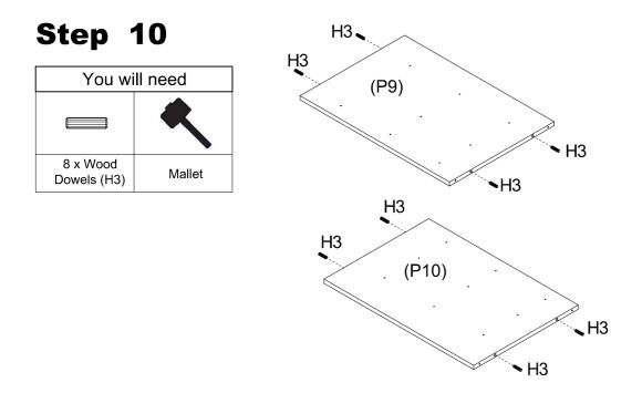
Insert 8 x Wood Dowels (H3) into Divider Panels (P9) and (P10).
