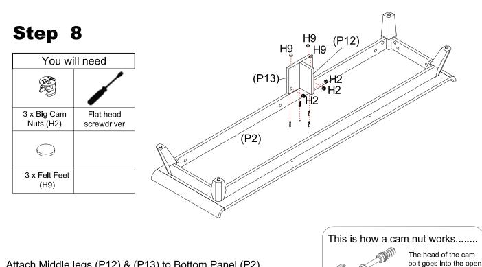
Attach Middle legs (P12) & (P13) to Bottom Panel (P2). Insert 3 x Big Cam Nuts (H2) into Middle Legs (P12) & (P13). Rotate the cam nuts so the arrows pointing towards the incoming cam bolts and turn clockwise to lock. Attached 3 x Felt Feet (H9) to Middle Legs (P12) & (P13).
