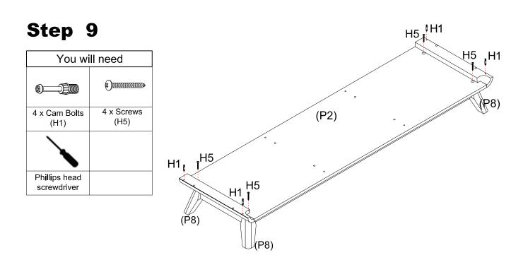
Screw 4 x Cam Bolts (H1) into Bottom Panel (P2) as shown. Use 4 x Screws (H5) through Bottom Panel (P2) to connect Legs (P8).
