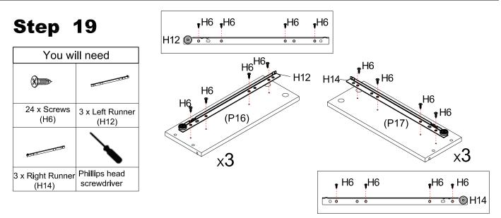
Attach each one Left Runner (H12) to Left Drawer Sides (P16) with 4 x Screws (H6). Repeat two times for all Left Drawer Sides (P16).
