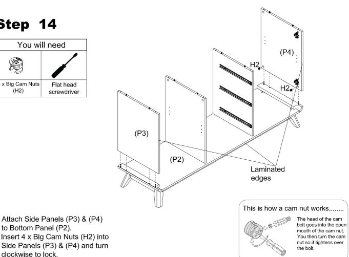
Make sure the laminated edges of Bottom Panel (P2), Side Panels (P3) and (P4) are facing the same direction.
