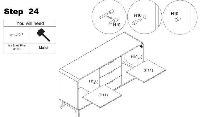
Insert 8 x Shelf Pins (H10) into desired holes in panels. Use a mallet to gently tap them into place if needed. Put Shelf Panels (P11) onto Shelf Pins (H10).
