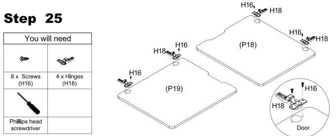
Insert 4 x Hinges (H18) into Doors (P18) and (P19). Attach with 8 x Screws (H16).
