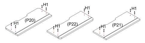
Screw each 4 x Cam Bolts (H1) into Drawer Fronts (P20) (P21) (P22) using a Phillips head screwdriver.
