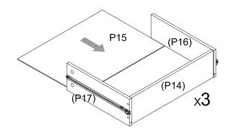
Slide each Drawer Base (P15) into the groove in the Drawer Panels (P17), (P16) and (P14). Repeat two times for all Drawer Bases (P15).
