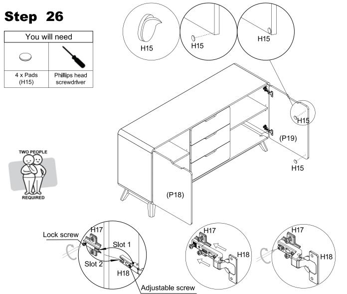
Attach doors onto cabinet as shown. Slide Hinge (H18) onto Hinge Base (H17), until each adjustable screw is in slot 1 and the lock screw is in the slot 2, then tighten lock screw. Attach 4 x Pads (H13) onto Doors (P15) and (P16).
