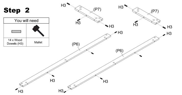
Insert each 3 x Wood Dowels (H3) into Short Rail (P7) and each 4 x Wood Dowels (H3) into Long Rail (P6).
