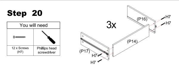
Attach each Drawer Side Panels (P16) and (P17) to each Drawer Back (P14) with 4 x Screws (H7). Repeat two times for all drawer panels.
