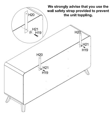
Use Screw (H19) to connect Wall Strap (H20) on Top Panel (P1).
