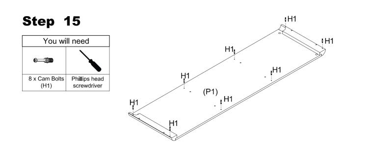
Screw 8 x Cam Bolts (H1) into Top Panel (P1) as shown.
