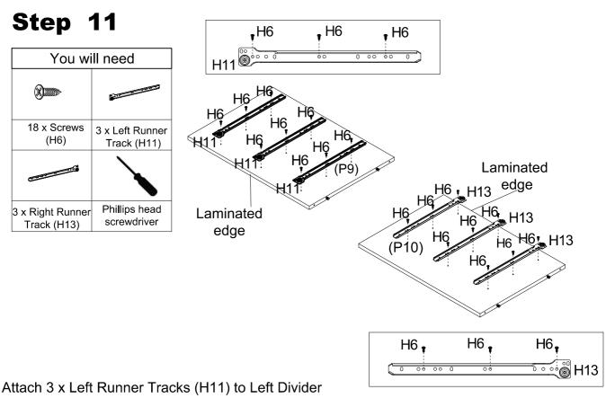
Attach 3 x Left Runner Tracks (H11) to Left Divider Panel (P9) with 9 x Screws (H6). Attach 3 x Right Runner Tracks (H13) to Right Divider Panel (P4) with 9 x Screws (H6).
