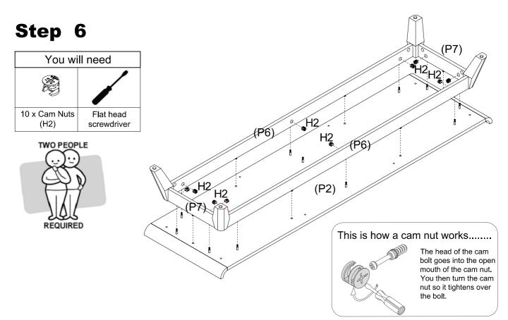
Attach Short Rail (P7) and Long Rail (P6) to Bottom Panel (P2).
