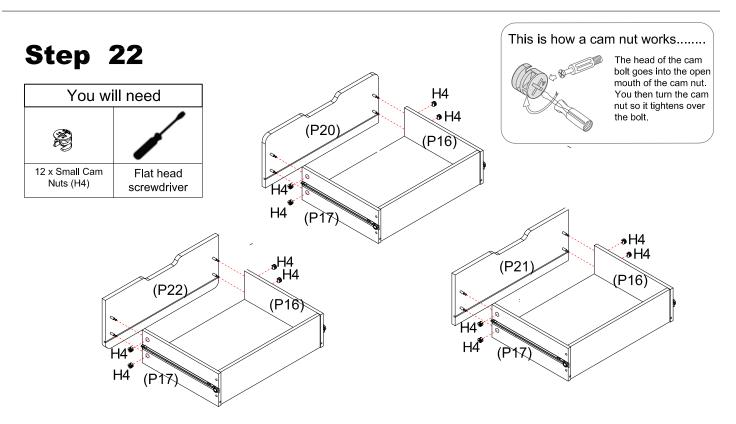
Attach Drawer Front (P20) to Drawer Sides (P17) & (P16). Insert 4 x Small Cam Nuts (H4) into Drawer Sides (P17) & (P16).Rotate the cam nuts so the arrows point towards the incoming cam bolt and turn clockwise to lock. Repeat for other Drawer Fronts (P21) & (P22).
