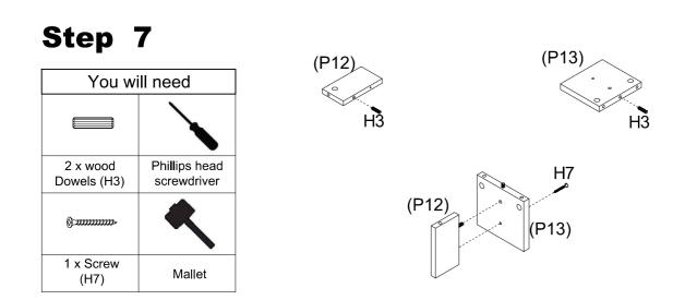
Insert 2 x Wood Dowels (H3) into Small Middle Leg (P12) and Big Middle Leg (P13). Attach Small Middle Leg (P12) to Big Middle Leg (P13) with 1 x screw (H7).
