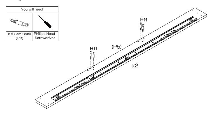
Attach 8 x Cam Bolts (H11) to Side Panels (P5) by tightening with the Phillips Head Screwdriver.
