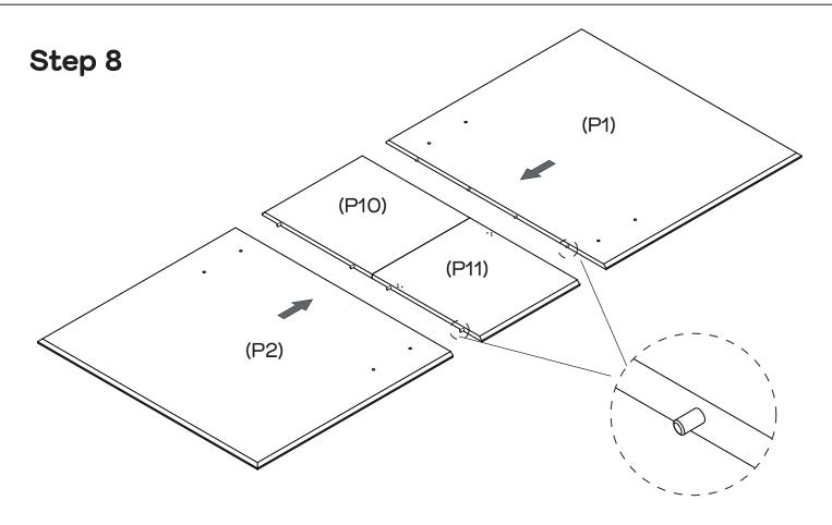
Lay table tops down on a soft surface to not scratch the finish. Attach Top Panel (P1&P2) and Scab (P10&P11) together.
