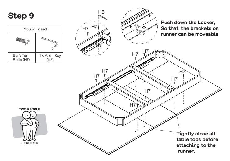
Push down the lockeron runner. Attach runner to Top Panels (P1&P2) with 8 x Small Bolts (H7) by tightening with the 1 x Allen Key (H5). Well align eight Bolts (H7) before fully tighten.
