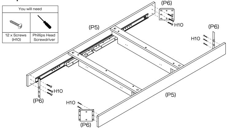
Attach Blocks (P6x4) to Side Panels (P5x2) with 12 x Screws (H10) by tightening with the Phillips Head Screwdriver.
