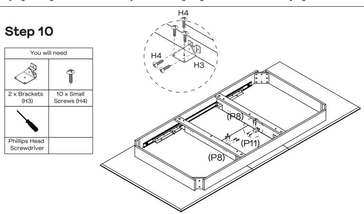
Attach 2 x Brackets (H3) to Scab (P11) and Rails (P8x2) with 10 x Small Screws (H4) by tightening with the Phillips Head Screwdriver.
