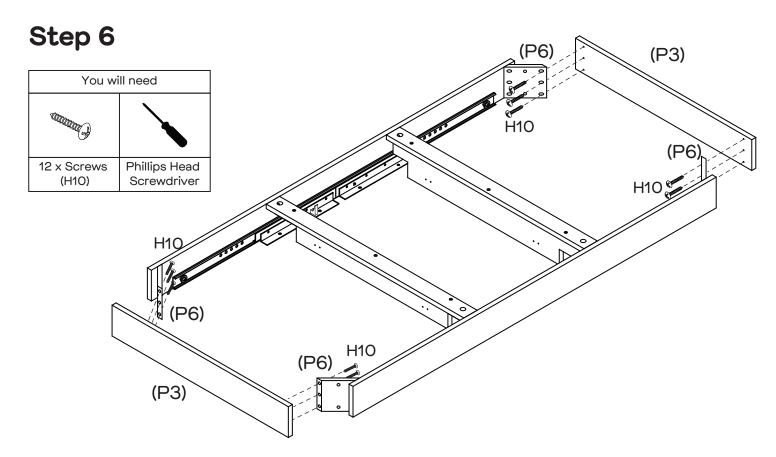
Attach Rails (P3x2) to Blocks (P6x4) with 12  $\times$  Screws (H10) by tightening with the Phillips Head Screwdriver.
