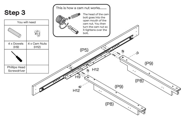
Insert 4 x Dowels (H9) into Side Panel (P5). Insert 4 x Cam Nuts (H12) into the holes of Rails (P8x2 & P9x2). Rotate the cam nuts so the arrow points towards the incoming cam bolts. Attach Rails (P8x2 & P9x2) to Side Panel (P5) by tightening the Cam Nuts (H12) with the Phillips Head Screwdriver.
