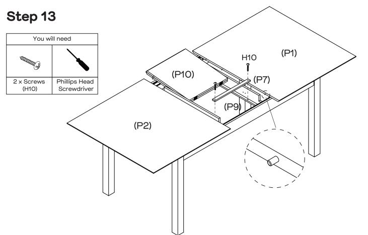
Attach Rails (P7) to Rails (P9x2) with  $2 \times \text{Screws}$  (H10) by tightening with the Phillips Head Screwdriver.
