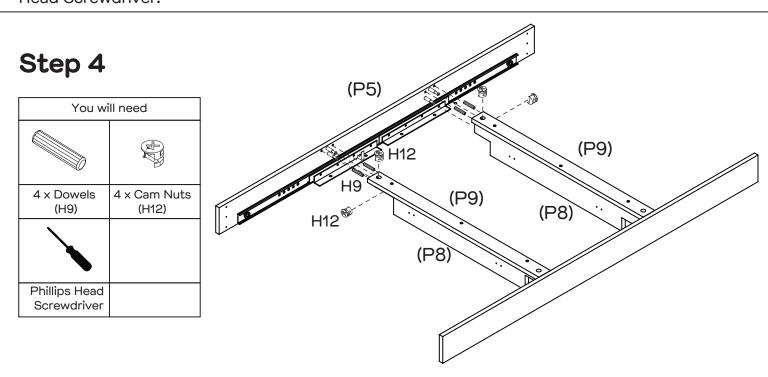
Insert 4 x Dowels (H9) into Side Panel (P5). Insert 4 x Cam Nuts (H12) into the holes of Rails (P8x2 & P9x2). Rotate the cam nuts so the arrow points towards the incoming cam bolts. Attach Rails (P8x2 & P9x2) to Side Panel (P5) by tightening the Cam Nuts (H12) with the Phillips Head Screwdriver.
