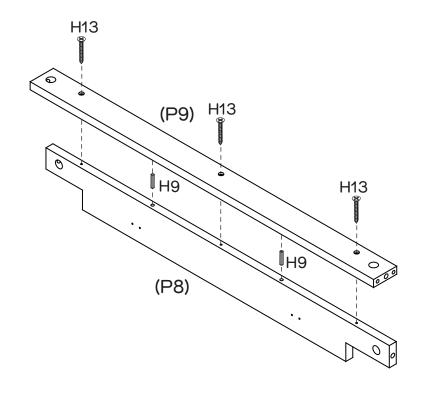
Attach Rails (P9x2) to Rails (P8x2) with 4 x Dowels (H9) and secure with 6 x Screws (H13). Tightening with the Phillips Head Screwdriver.
