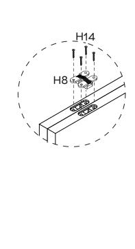
Attach 2 x Barckets (H8) to Scab (P10&P11) with 8 x Screws (H14) by tightening with the Phillips Head Screwdriver.
