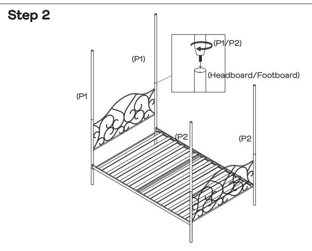
Screw in, by rotating clockwise 2 x short posts (P1) into the cornerposts of the headboard until secure.
