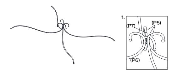
Assemble the canopy, beginning with canopy top (P6) with the thread bolt facing upwards. Place 3 x canopy top (P5) onto the thread bolt and secure them together by screwing the centre finial (P7) onto the top of the thread by turning in a clockwise direction.
