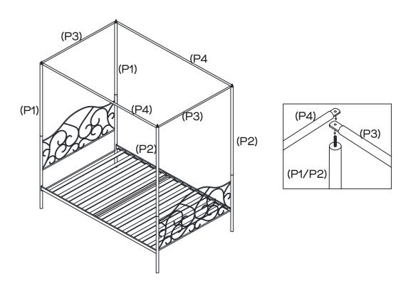
Place a short cross bar (P3) across each end of the bed, aligning the holes to the bolts on the cornerposts (P1 & P2).
