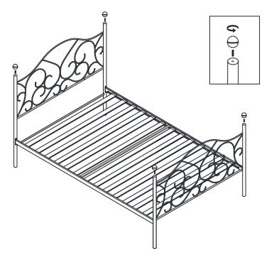
Begin with an assembled Giselle Single Bed (sold separately). Remove the 4 x finials (P8) and the 4 x headless bolts (H1) from the corner posts by unscrewing in an anti-clockwise direction and set aside.
