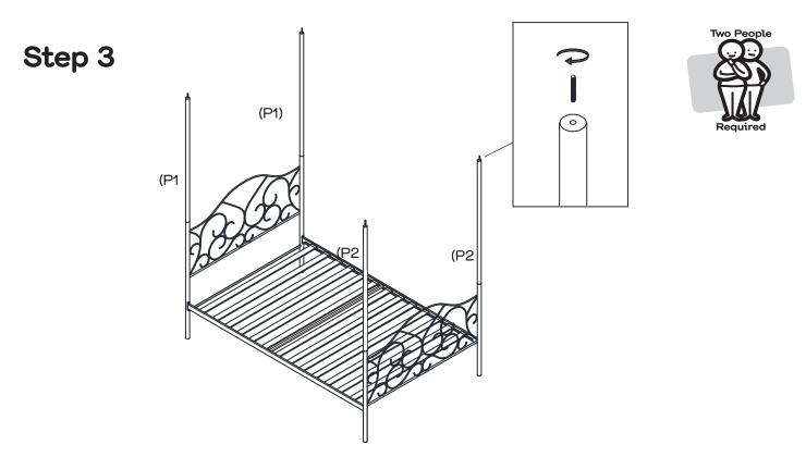
Screw in a headless bolt (H1) into the top of each of the 4 cornerposts by rotating clockwise.
