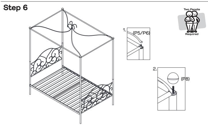
Carefully place the pre-assembled canopy top onto the exposed headless bolts on the cornerposts (P1 & P2).
