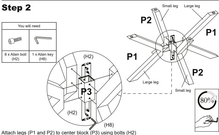
Attach legs (P1 and P2) to center block (P3) using bolts (H2) and Allen key (H8).Make sure large legs (P1) and small legs (P2) are in correct sequence before tightning bolts. Be aware to only tighten bolts 80%, you will fully tighten these in step 4.
