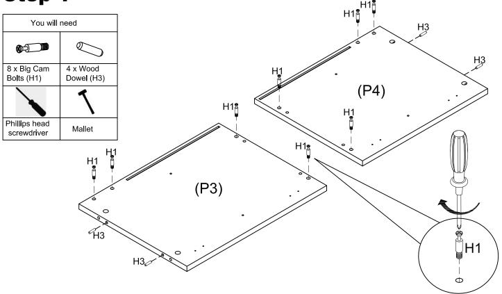
Using a mallet if needed, Insert 4 x Dowel (H3) onto the Left Side Panel (P3) and Right Side Panel (P4). Screw 8 x Big Cam Bolt (H1) onto the Left Side Panel (P3) and Right Side Panel (P4).
