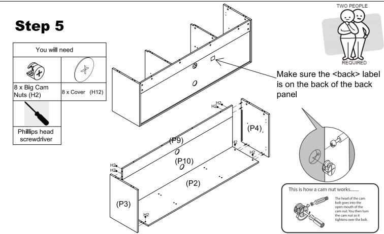
Position the Side Panel (P3,P4) to the Bottom Panel (P2) and Back Rail (P9) and Back Panel (P10). Insert the 8 x Big Cam Nuts (H2) to the Bottom Panel (P2) and Back Rail (P9) make sure the opening on nuts is facing incoming cam bolt,turn clockwise to lock. Insert the 8 x Covers (H12) onto the Big Cam Nuts (H2).
