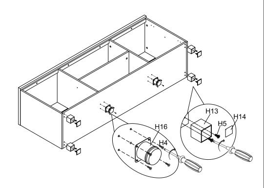
Attach 4 x Leg (H13) to Bottom Panel by using 8 x Bolt (H5), then insert 4 x Leg Cap (H14) onto Leg (H13).attach 2 x Leg (H16) to Bottom Panel by using 8 x Small Screw (H4).
