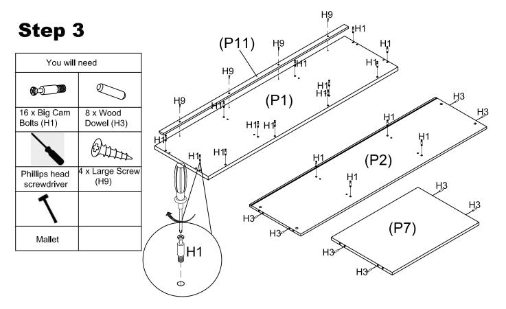
Using a mallet if needed, Insert 8 x Dowel (H3) onto the Bottom Panel (P2) and Middle Shelf Panel (P7).
