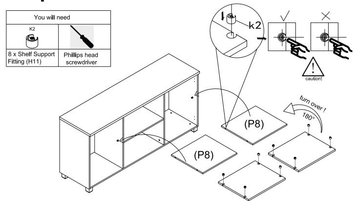
Insert 8 x Shelf Support Fitting (H11-K2) onto the Shelf Panel (P8) make sure the opening on Shelf Support Fitting is facing to the panel edge.turn the panel down then position to the Shelf Support Fitting (H11-K1).
