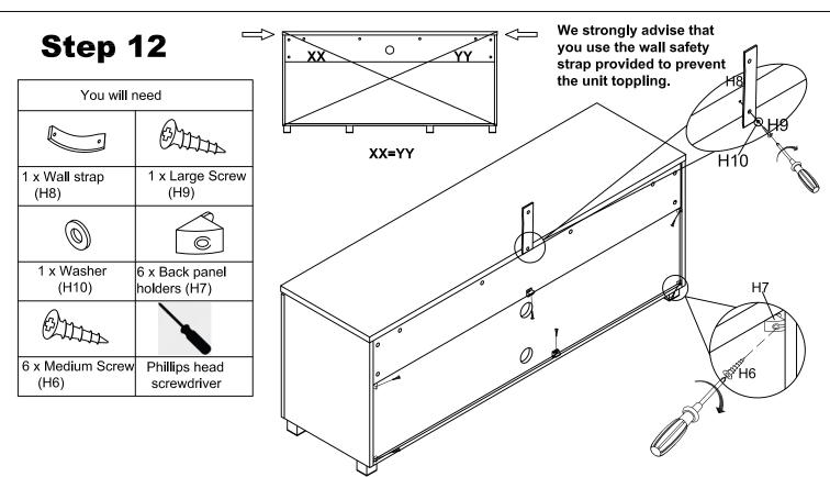
If necessary, gently adjust the Top Panel (P1) sideway in either direction untill XX and YY are equal Slide 6 x Back Panel holders (H7) into the grooves as shown. Insert 6 x Medium Screw (H6) to fix them into place. Tighten the Screw (H6) with a Phillips Head Screwdriver Tighten the Wall Strap (H8) to the Top Panel (P1) with Large Screw (H9) and Washer (H10).
