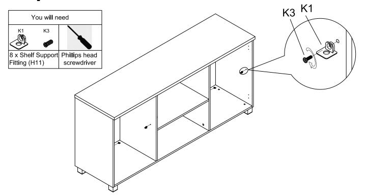
Insert 8 x Shelf Support Fitting (H11-K1) onto the Left Side Panel (P3) and Right Side Panel (P4) and Middle Side Panel (P5,P6) by using 8 x Shelf Support Fitting (H16-K3).
