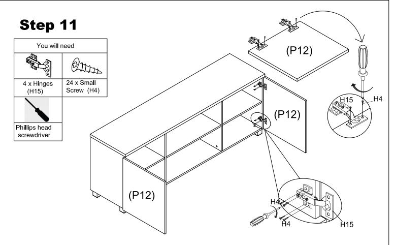
Attach 4 x Hinges (H15) onto the Door Panel (P12) by using 8 x Small Screw (H4) then attach the Hinges (H15) onto the Side Panel (P3,P4) by using 16 x Small Screw (H4).
