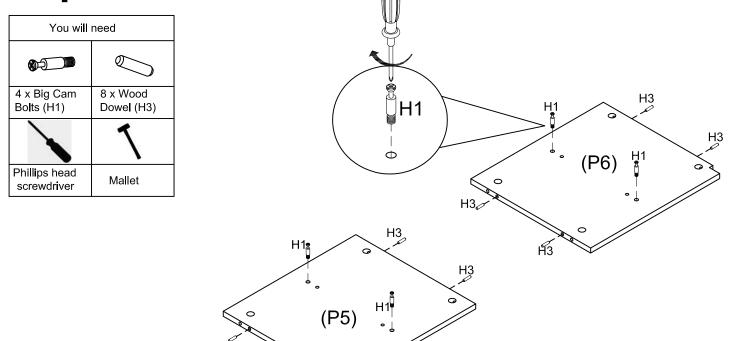
Using a mallet if needed, Insert 8 x Dowel (H3) onto the Middle Side Panel (P5,P6). Screw 4 x Big Cam Bolt (H1) onto the Middle Side Panel (P5,P6).
