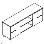
**STEP 13.3** Adjust the flush between door panel and side panel
