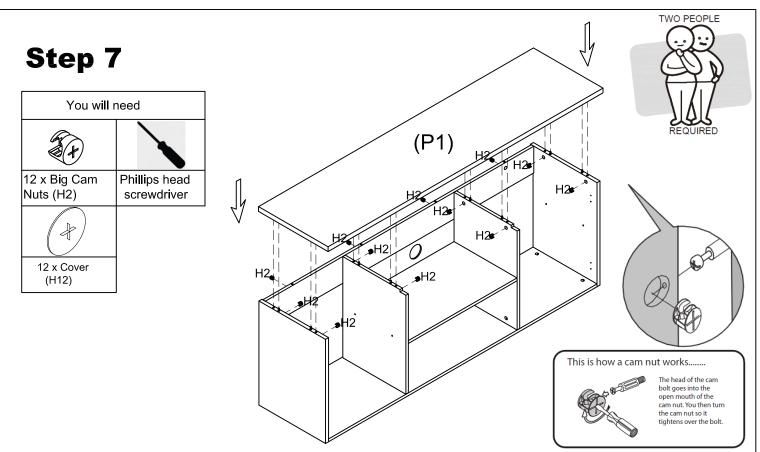
Position the Top Panel (P1) to the Left Side Panel (P3) and Right Side Panel (P4) and Middle Side Panel (P5,P6) and Back Rail (P9).
