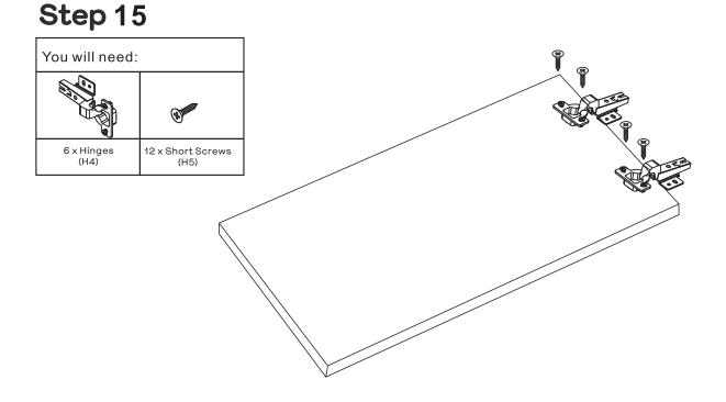
Using 4 x Short Screws(H5) to connect 2 x Hingers(H4) to Right Door(P13) Adjust the door then tighten all screws with a Phillips Head Screwdriver. Repeat previous step for Anther Right Door(P13) and Left Door(P12)
