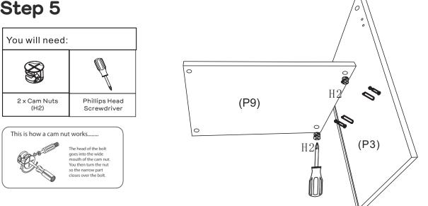
Insert 2 x Cam Nuts(H2) into Short Shelf(P9) as shown.Rotate the cam nuts so the arrows point towards the incoming cam bolts. Attach Short Shelf(P9) to Right Panel(P3) by tightening the cam nuts(H2)
