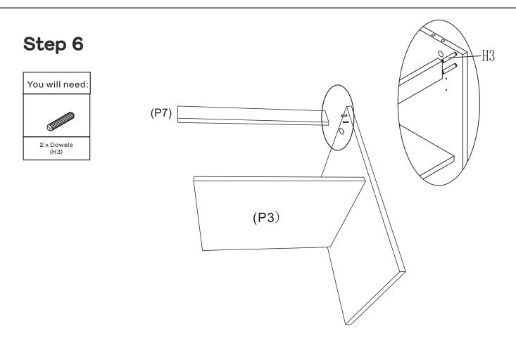
Insert 2 x Dowels(H3)into Right Panel(P3) and connect Short Support(P7) to Right Panel(P3).
