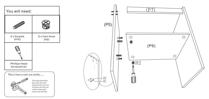
Insert 2 x Dowels(H15) into Middle Panel(P5) Insert 2 x Cam Nuts(H2) into Short Shelf(P9) as shown. Rotate the cam nuts so the arrows point towards the incoming cam bolts. Attach Short Shelf(P9) to Middle Panel(P5) by tightening the Cam Nuts(H2) with the Phillips Head Screwdriver
