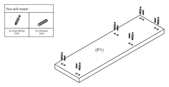
Insert 6 x Dowels(H3) into Unit Top(P1) and secure 6 x Cam Bolts(H1) into Unit Top(P1) by tightening with the Phillips Head Screwdriver.
