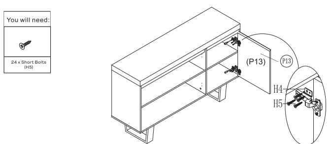
Using 8 x Short Screws(H5) to connect Right Door(P13) to Buffet by tightening with a Phillips head screwdriver. Repeat previous step for Right Door(P13) and Left Door(P12)
