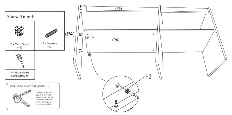
Insert 2 x Dowels(H3) into Left Panel(P4) to connect with Long Support(P6). Insert 4 x Cam Nuts(H2) into Long Shelf(P8) as shown. Rotate the cam nuts so the arrows point towards the incoming cam bolts. Attach Long Shelf(P8) to Left Panel(P4) by tightening the Cam Nuts(H2)
