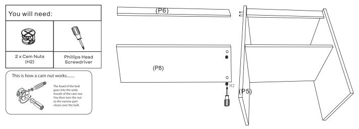
Connect Long Support(P6) to Middle Panel(P5) by Dowels(H15). Insert 2 x Cam Nuts(H2) into Long Shelf(P8) as shown. Rotate the cam nuts so the arrows point towards the incoming cam bolts. Attach Long Shelf(P8) to Middle Panel(P5) by tightening the Cam Nuts(H2) with the Phillips Head Screwdriver
