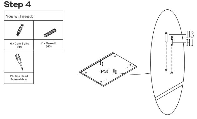
Insert 2 x Dowels(H3) into Middle Right Panel(P3) and secure 2 x Cam Bolts(H1) to Middle Right Panel(P3) by tightening with the Phillips Head Screwdriver. Repeat previous step for Left Panel (P4) and Middle Panel(P5).
