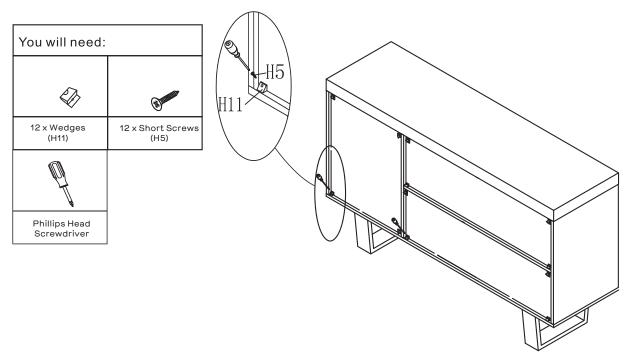
Insert 12 x Wedges(H11) into all corners of the back of the assembled unit as shown. Secure Wedges(H1) by tightening 12 x Short Screws(H5) with the Phillips Head Screwdriver.
