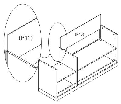
Turn over the Buffet Slide another Long Back Panel(P10) and Short Back Panel(P11)into the groove.
