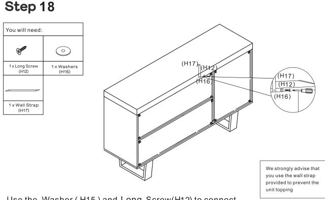
Use the Washer (H15) and Long Screw(H12) to connect the Wall Strap (H16) to the top Shelf (P1) using the Phillips head Screwdriver.
