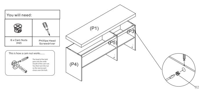
Insert 6 x Cam Nuts(H2) into Panel(P3&P4&P5) as shown.Rotate the cam nuts so the arrows point towards the incoming cam bolts. Attach Top(P1) to Panel(P3&P4&P5) by tightening the Cam Nuts(H2) with the Phillips Head Screwdriver
