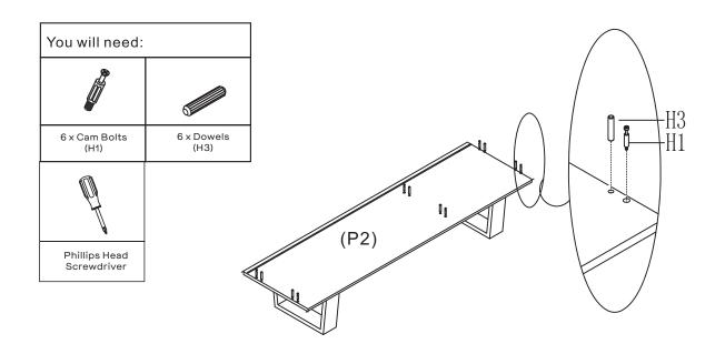
Insert 6 x Dowels(H3) into Unit Bottom(P2) and secure 6 x Cam Bolts(H1) to Unit Bottom(P2) by tightening with the Phillips Head Screwdriver.
