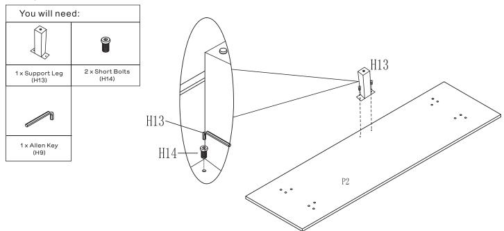
Using 2 x Short Bolts(H4) secure the Support Leg(H13) to the Unit Bottom(P2) by tightening with Allen Key(H9).
