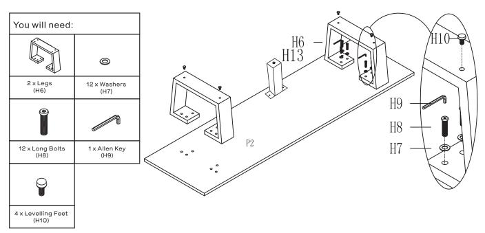
Using 6 x Washers(H7) and 6 x Long Bolts(H8) secure the Table Leg(H6) to the Unit Bottom(P2) by tightening with Allen Key(H9) Repeat the previous step to attach the second Table Leg(H6). Screw in 4 x Levelling Feet(H10) to the bottom of the Table Legs(H6) Ensure the Levelling Feet are screwed in firmly.If your flooring surface is uneven adjust the Levelling Feet accordingly.
