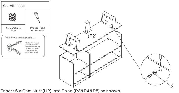
Rotate the cam nuts so the arrows point towards the incoming cam bolts. Attach Bottom(P2) to Panel(P3&P4&P5) by tightening the Cam Nuts(H2) with the Phillips Head Screwdriver
