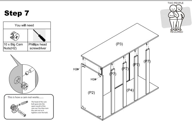
Place Left Side (P3) on to position ,insert 10 x Big Cam Nut (H2) into the holes on Panel (P2,P5,P6,P7) make sure the opening on cam nut face incoming cam bolts, turn clockwise to lock.
