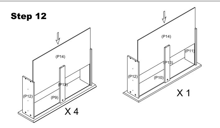
Insert the Drawer Base Panel (P14) into the grooves of the Drawer Front (P9,P10), Drawer Left Side (P11) and Drawer Right Side (P12)
