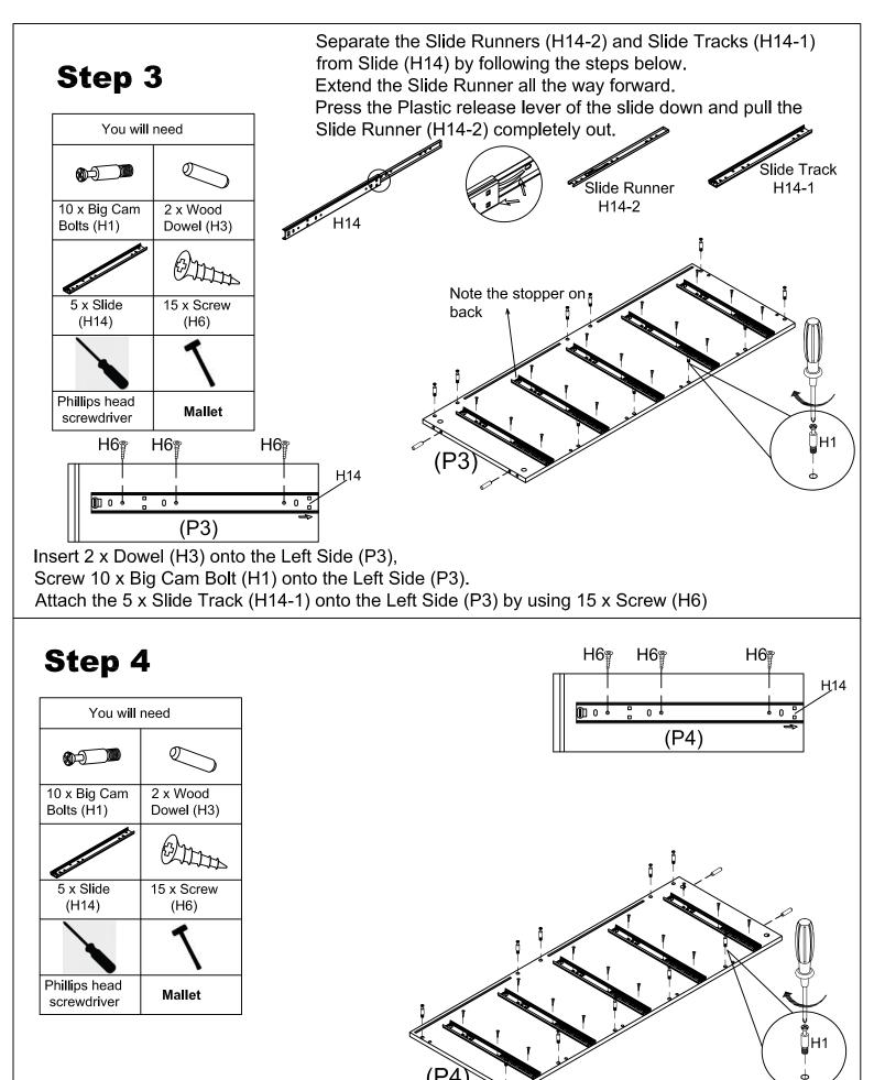
Insert 2 x Dowel (H3) onto the Right Side (P4), Screw 10 x Big Cam Bolt (H1) onto the Right Side (P4). Attach the 5 x Slide Track (H14-1) onto the Right Side (P4) by using 15 x Screw (H6)
