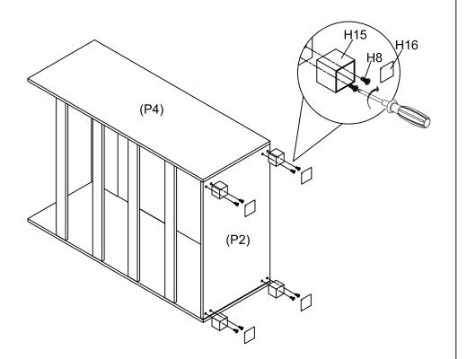
Attach 4 x Leg (H15) to Bottom of Base Panel by using 8xBolt (H8), then insert Plastic Cap (H16) onto Leg (H15)
