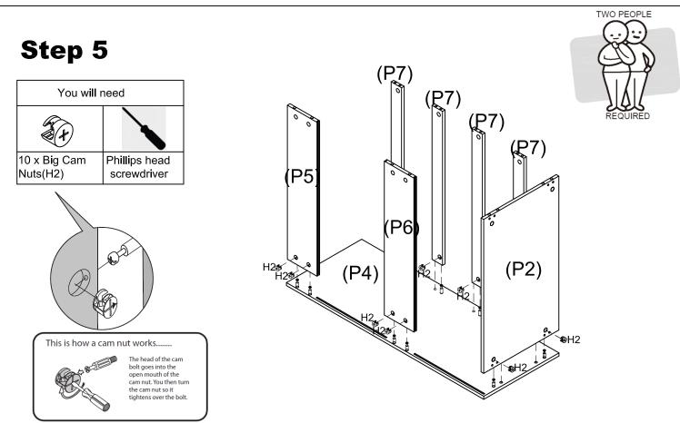
Position the Base Panel (P2) and Back Panel (P5,P6) and 4 x Front Rail (P7) onto the Right Side (P4),
