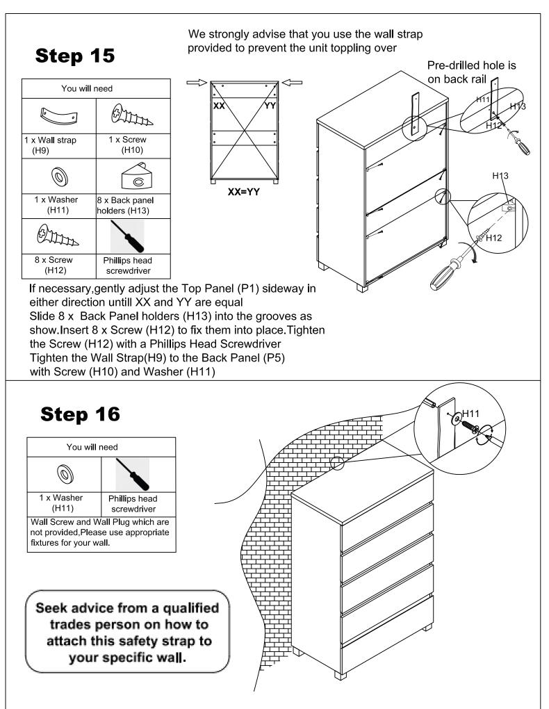
Move the Tall boy to the final position, and attached the wall strap to the wall securely. Make sure it is firmly attached and snug fit.
