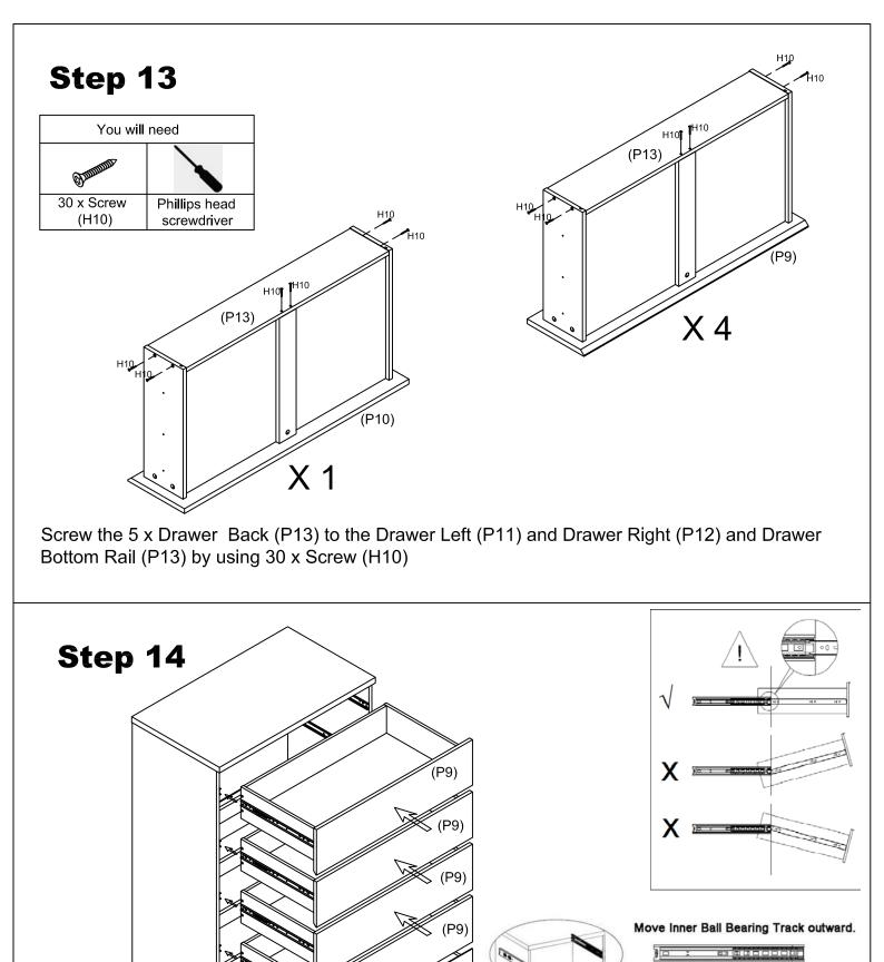
Position Drawer box so that Slide Runner (H14-2) aligns with Side Track (H14-1) as shown.
