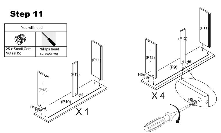
Position the 5 x Drawer Left Side (P11) and 5 x Drawer Right Side (P12) and 5 x Drawer Bottom Rail (P13) to the Drawer Front (P9,P10),insert 25 x Small Cam Nut (H5) into the holes on Panel (P11,P12,P13) as show, make sure the opening on cam nut is facing incoming cam bolts, turn clockwise to lock.
