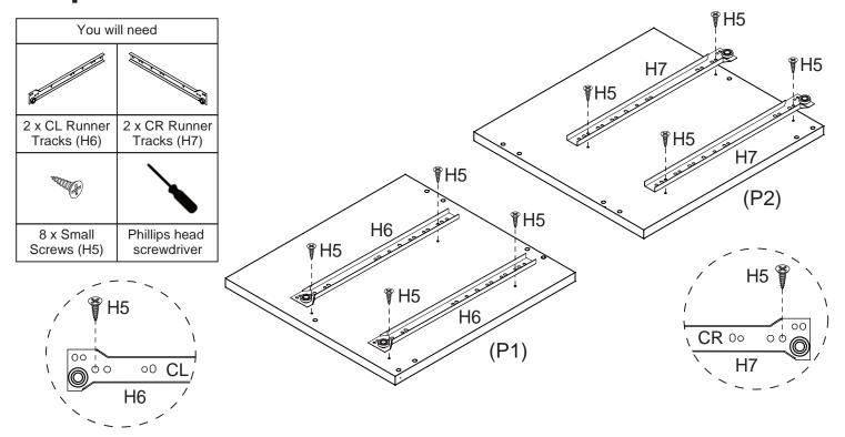
Attach 2 x CL Runner Tracks (H6) to Left Side Panel (P1) with 4 x Small Screws (H5). Attach 2 x CR Runner Tracks (H7) to Right Side Panel (P2) with 4 x Small Screws (H5).
