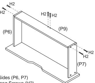
Attach Drawer Back (P9) to Drawer Sides (P6, P7) and Drawer Support (P10) with 6 x Long Screws (H2),
