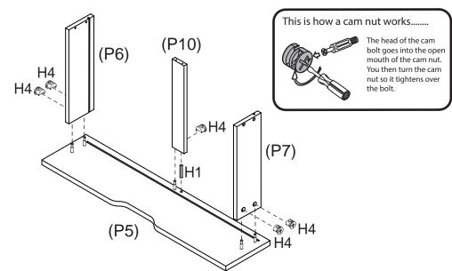
Insert 1 x Dowel (H1) into Drawer Front (P5) as shown.
