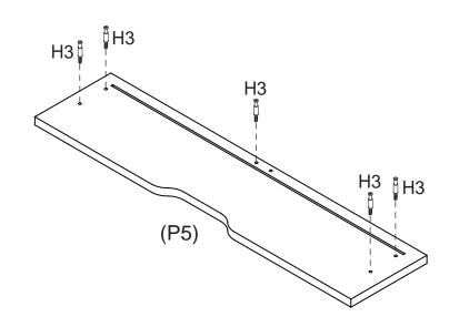
Screw 5 x Small Cam Bolts (H3) into Drawer Front (P5) with a Phillips head screwdriver. www.fantasticfurniture.com.au
