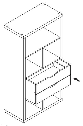
Put the insert cabinet into the bookcase, make sure the drawer front of insert cabinet is flush with the edge of shelf.
