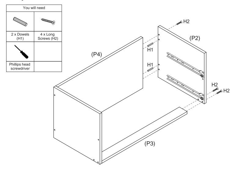
Insert 2 x Dowels (H1) into the holes of Back Panel (P4) as shown. Attach Right Side Panel (P2) to Back Panel (P4) and Rail (P3) with 4 x Long Screws (H2). Tighten the screws with a Phillips head screwdriver.
