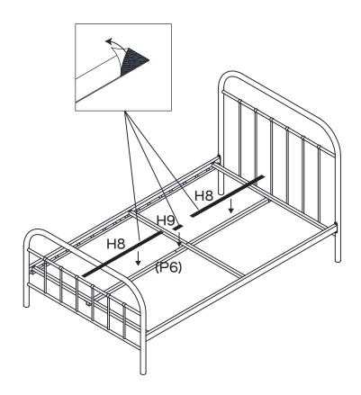
Peel off the adhesive strip protective paper and apply downward pressure on the centre rail with the strip until fully applied.
