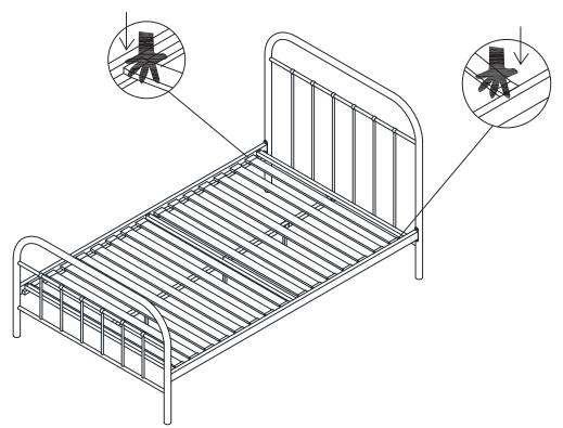
Lower the slat (P9) with the end connectors (P8) to the side rails (P3). Ensure the plastic slat caps are in place over the side rail holes and apply downward pressure until the plastic slat caps are fully inserted into the rails. Repeat for every bed slat until finished.
