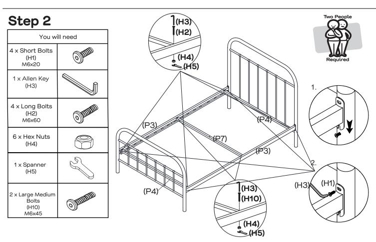
Attach the 2 x side rails (P3) to the headboard (P1) and footboard (P2).
