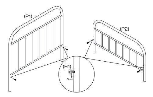
Insert  $4 \times 8$  short bolts (H1) into the bottom holes of the headboard (P1) and footboard (P2) using the allen key (H3). Do not fully tighten the bolts and leave a gap of 5mm as shown.
