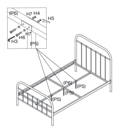
Attach the 3 x support legs (P5) to the centre rail (P6) with 6 x medium bolts (H6) 12 x metal washers and 6 x hex nuts (H4).
