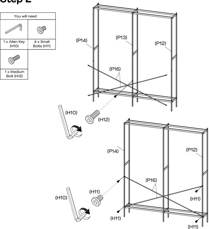
Attach Support Bars (P16x2) to the Middle Side Frame (P13) with 1x Medium Bolt (H12) by tightening with the Allen Key (H10) as shown.
