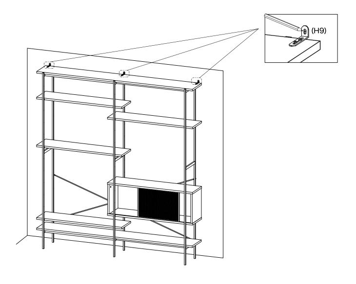
Connect the 3  $\times$  Wall Brackets (H9) to the wall. Make sure it is firmly attached and a snug fit.
