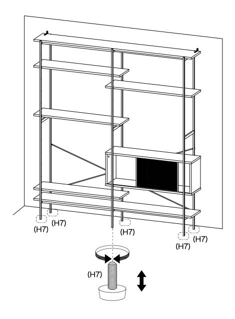
If the floor is uneven, adjust the 6 x Adjustable Feet (H7) to balance the Bookcase if needed.
