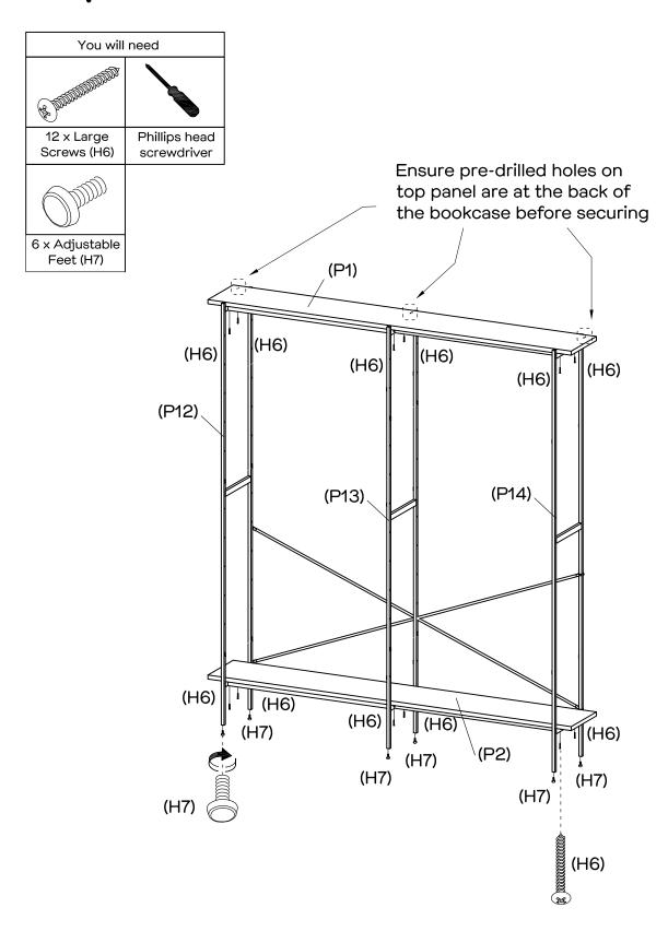
Attach the Top Panel (P1) and Base Panel (P2) to Right Frame (P14), Middle Frame (P13) and Left Frame (P12) with 12 x Large Screws (H6) using Phillips head screwdriver.
