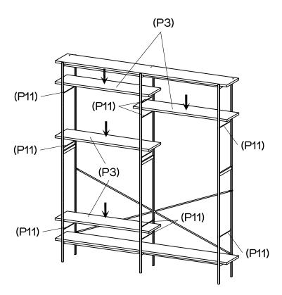
Place the Shelves (P3x4) into position by resting on the Shelf Supports (P11x10) as shown. Ensure that the grooves on the bottom of the shelves slot into the shelf supports and each shelf is firmly secure.
