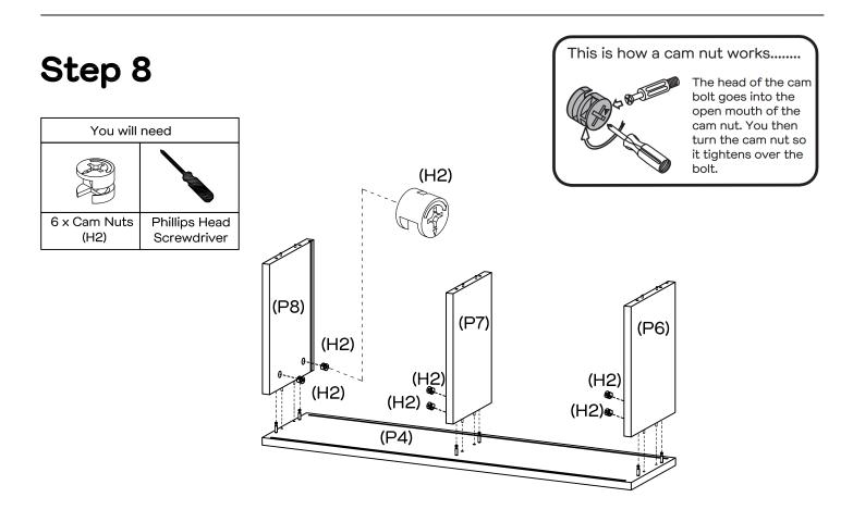
Insert 6 x Cam Nuts (H2) into Cupboard Left, Middle & Right Side Panels (P6, P7 & P8) as shown. Rotate the Cam Nuts so the arrows point towards the incoming Cam Bolts. Attach Cupboard Left, Middle & Right Side Panels (P6, P7 & P8) to Cupbard Top Panel (P4) by tightening the Cam Nuts with the Phillips Head Screwdriver.
