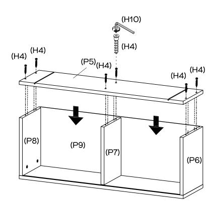
Slot Cupboard Back Panel (P9) into the grooves of Cupboard Top Panel (P4) and Left & Right Side Panels (P6 & P8) as shown. Attach Cupboard Base Panel (P5) to Cupboard Left, Middle & Right Side Panels (P6, P7 & P8) with 6 x Connecting Screws (H4) by tightening with the Allen Key (H10).
