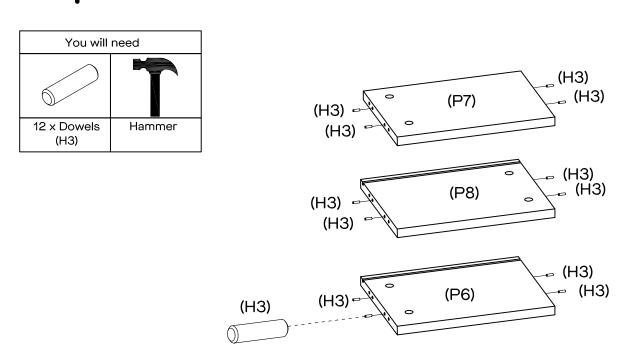
Insert 12 x Dowels (H3) into Cupboard Left, Middle & Right Side Panels (P6, P7 & P8) as shown by gently tapping in with the Hammer if needed.
