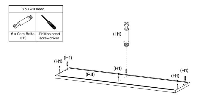
Attach 6 x Cam Bolts (H1) to Cupboard Top Panel (P4) as shown using Phillips head screwdriver.
