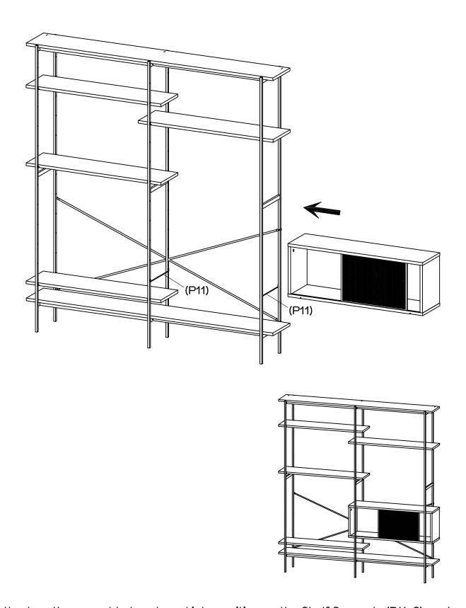
Gently place the assembled cupboard into position on the Shelf Supports (P11x2) as shown. Ensure that the grooves on the bottom of the cupbard slot into the shelf supports and the cupboard is firmly secure.
