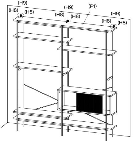
Attach 3  $\times$  Wall Brackets (H9) to Top Panel (P1) with 6  $\times$  Small Screws (H8) as show using Phillips head screwdriver.
