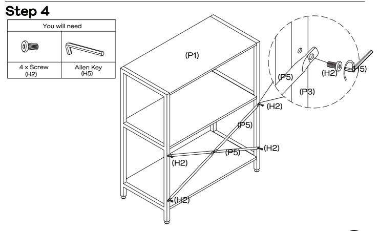
Attach Back Supports (P5x2) to Left & Right Side Frames (P3&P4) as shown with  $4 \times$ Screws (H2) by tightening with the Allen Key (H5).
