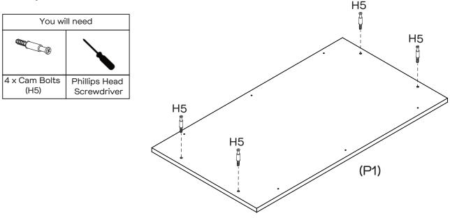
Attach 4 x Cam Bolts (H5) to Top Panel (P1) by tightening with the Phillips Head Screwdriver.
