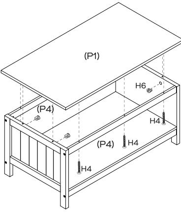
Insert 4 x Cam Nuts (H6) into Side Panels (P2x2) as shown. Rotate the cam nuts so the arrow points towards the incoming cam bolts. Attach Rails (P4x2) and Side Panels (P2x2) to Top Panel (P1) with 6 x Long Screws (H4) by tightening with the Phillips Head Screwdriver.
