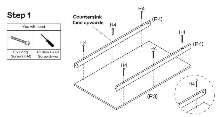
Attach Rails (P4x2) to Bottom Panel (P3) with 6 x Screws (H4) by tightening with the Phillips Head Screwdriver.
