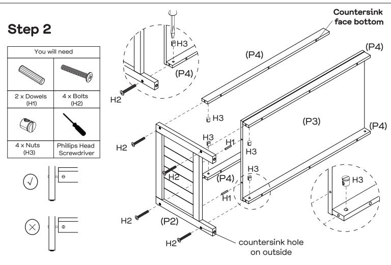
Insert 2 x Dowels (H1) into Bottom Panel (P3). Push 4 x Bolts (H2) through Side Panel (P2) and insert 4 x Nuts (H3) into Rails (P4x4). Rotate the nuts so the opening point towards the incoming bolts. Attach Rails (P4x4) to Side Panel (P2) by tightening all nuts with the Phillips Head Screwdriver.
