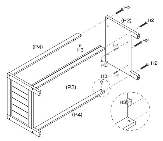
Insert 2 x Dowels (H1) into Bottom Panel (P3). Push 4 x Bolts (H2) through Side Panel (P2) and insert 4 x Nuts (H3) into Rails (P4x4). Rotate the nuts so the opening point towards the incoming bolts. Attach Rails (P4x4) to Side Panel (P2) by tightening all nuts with the Phillips Head Screwdriver.
