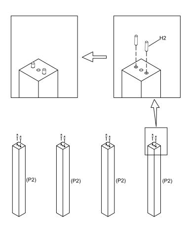
Using a Mallet if needed, Insert 8 x Wood Dowels (H2) to the hole on Leg (P2) as shown.
