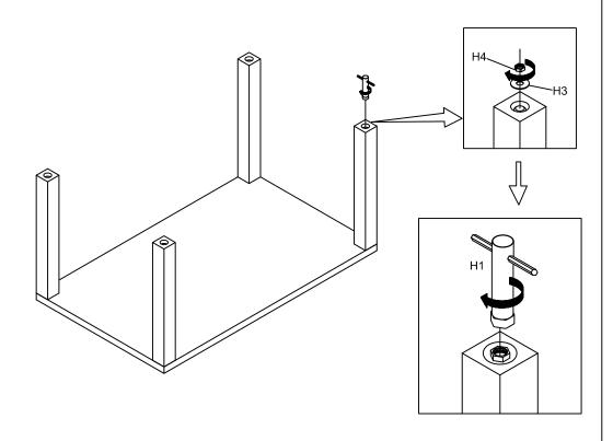
Insert 4 x Washer (H3) and 4 x Hexagonal Nuts (H4) as shown. Using the Spanner (H1) to tighten the Hexagonal Nuts to the Long Bolt.
