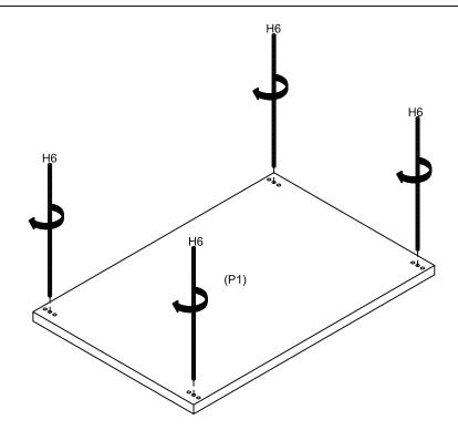
Lay table top down on a soft surface as to not scratch the finish. Insert 4 x Long Bolt (H6) to the Top Panel (P1) as shown.
