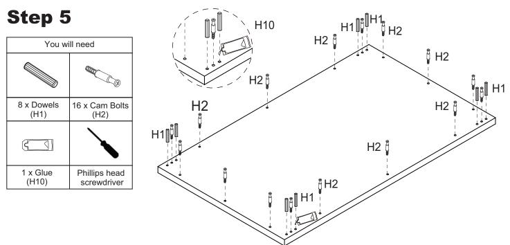
Squeeze Glue (H10) into dowel holes in Top Panel (P1) and insert 8 x Dowels (H1). Screw 16 x Cam Bolts (H2) into Top Panel (P1) with a Phillips head screwdriver.
