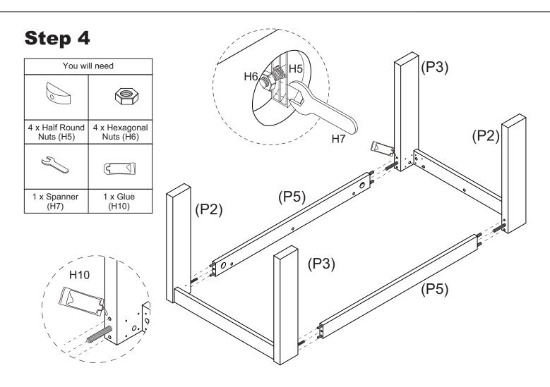
Squeeze Glue (H10) into dowel holes in Legs (P2, P3). Attach Long Apron (P5) to Legs (P2, P3) with 4 x Half Round Nuts (H5) and 4 x Hexagonal Nuts (H6) using Spanner (H7).
