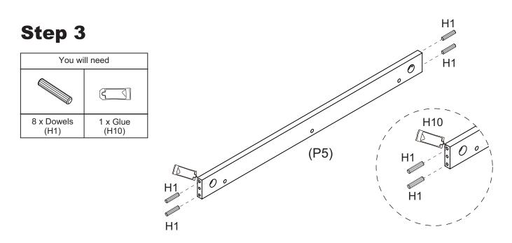
Squeeze Glue (H10) into dowel holes in Long Apron (P5) and insert 4 x Dowels. **Repeat Step 3 for another Long Apron (P5).**
