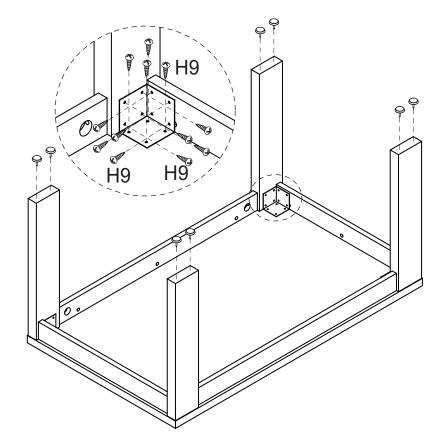
Attach 4 x Corner Fitting (H8) to the dinning table with 48 x Screws (H9) as shown. Tighten Screws using a Phillips head screwdriver. Hammer 8 x Plastic Glides (H11) into end of each leg (P2, P3)
