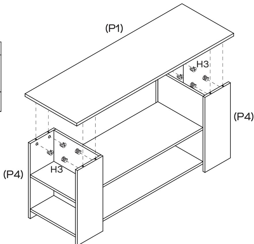
Insert 8 x Cam Nuts (H3) into the holes of Side Panels (P3, P4). Rotate the cam nuts so the arrows point towards the incoming cam bolts. Attach Top Panel (P1) and tighten the cam nuts using a Flat head screwdriver.
