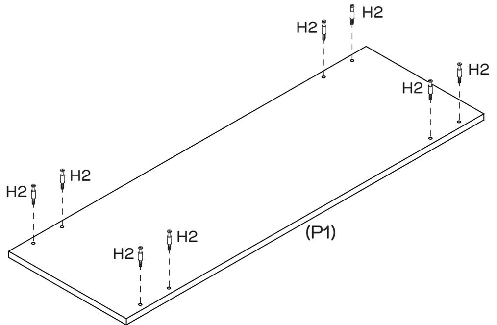
Attach 8 x Cam Bolts (H2) into Top Panel (P1). Tighten Cam Bolts using a Phillips head screwdriver.
