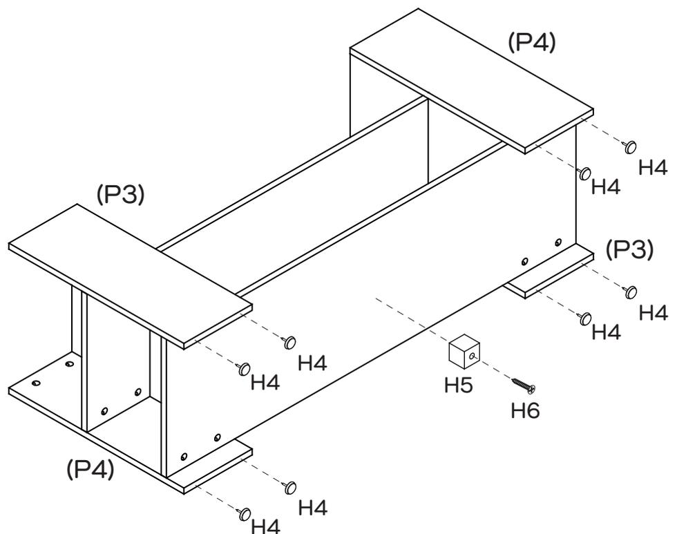
Hammer 8 x Plastic Glides (H4) on to end of Shelf Panels (P3, P4). Attach 1 x Support Leg (H5) to the bottom of Shelf Panel (P2) with 1 x Screw (H6).
