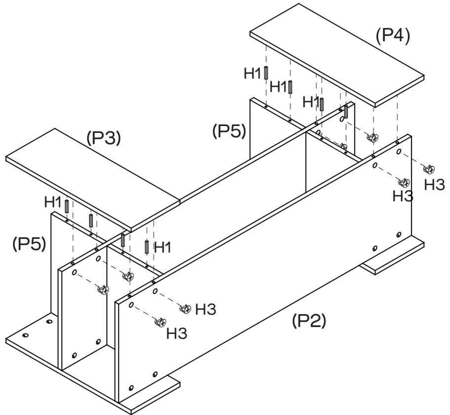
Insert 4 x Cam Nuts (H3) into the holes of Shelf Panel (P2) as shown. Rotate the cam nuts so the arrows point towards the incoming cam bolts. Attach Side Panels (P3, P4) to Shelf Panel (P2), then tighten the cam nuts using a Flat head screwdriver.
