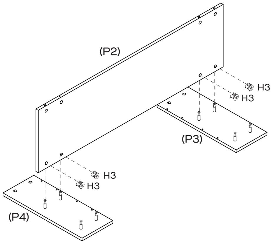
Insert 4 x Cam Nuts (H3) into the holes of Shelf Panel (P2) as shown. Rotate the cam nuts so the arrows point towards the incoming cam bolts. Attach Side Panels (P3, P4) to Shelf Panel (P2), then tighten the cam nuts using a Phillips head screwdriver.
