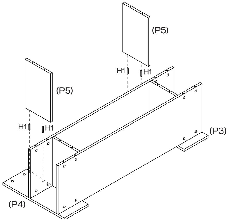
Insert 4 x Dowels (H1) into Side Panels (P3, P4). Put Dividers (P5) to the place as shown.
