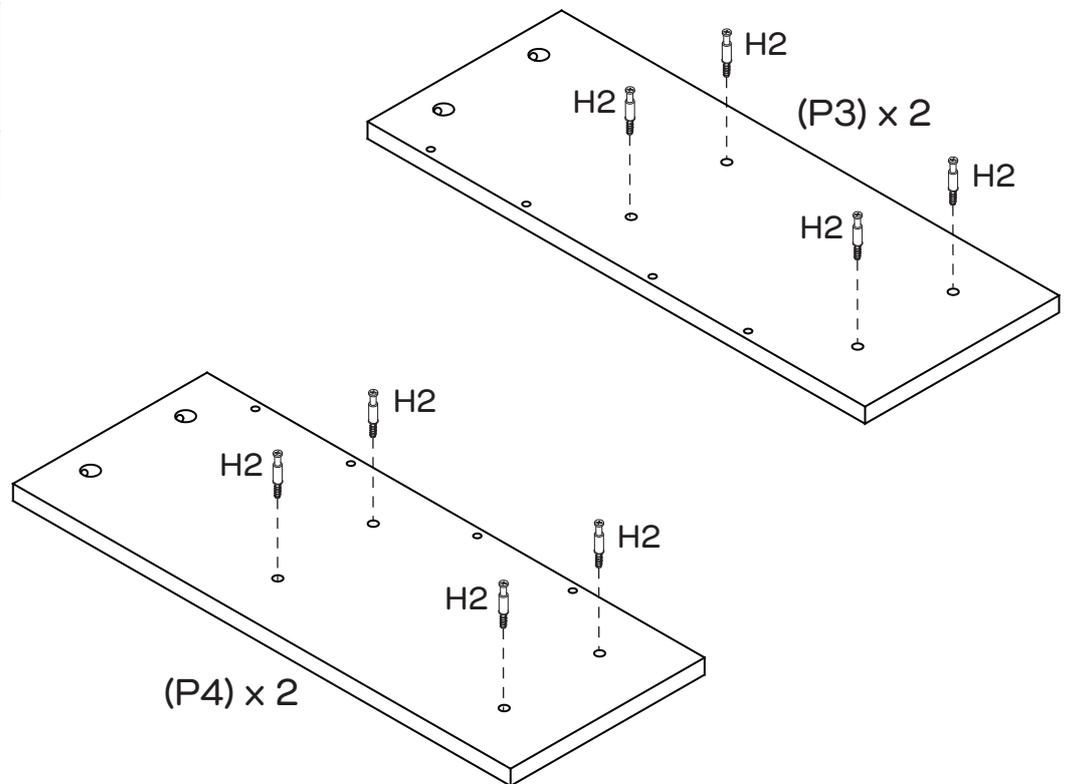
Attach 8 x Cam Bolts (H2) into Left Side Panel (P3) and Right Side Panel (P4) using a Phillips head screwdriver.
