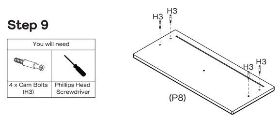
Attach  $4 \times \text{Cam}$  Bolts (H3) to Drawer Front Panel (P8) by tightening with the Phillips Head Screwdriver.
