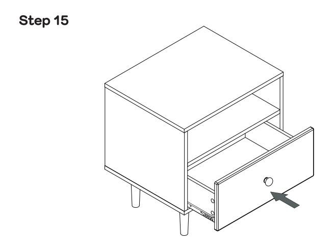
Insert the assembled drawer into the corresponding compartment as shown. Ensure the drawer slide easily along the rails.
