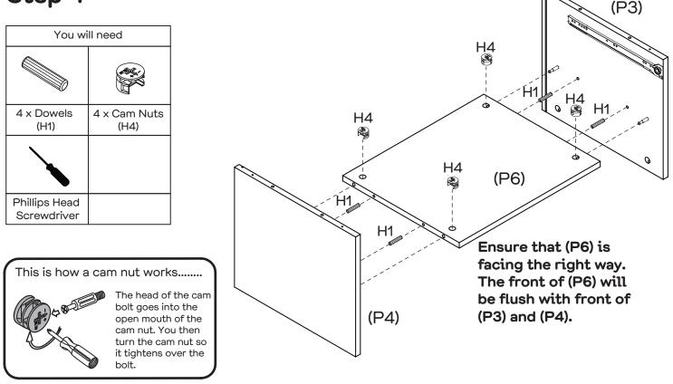
Insert 4 x Cam Nuts (H4) and 4 x Dowels (H1) into Shelf Panel (P6) as shown. Rotate the cam nuts so the arrows point towards the incoming cam bolts. Attach Left & Right Side Panels (P3 & P4) to Shelf Panel (P6) by tightening all cam nuts with the Phillips Head Screwdriver.
