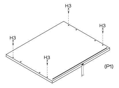
Attach 4 x Cam Bolts (H3) to Top Panel (P1) by tightening with the Phillips Head Screwdriver.
