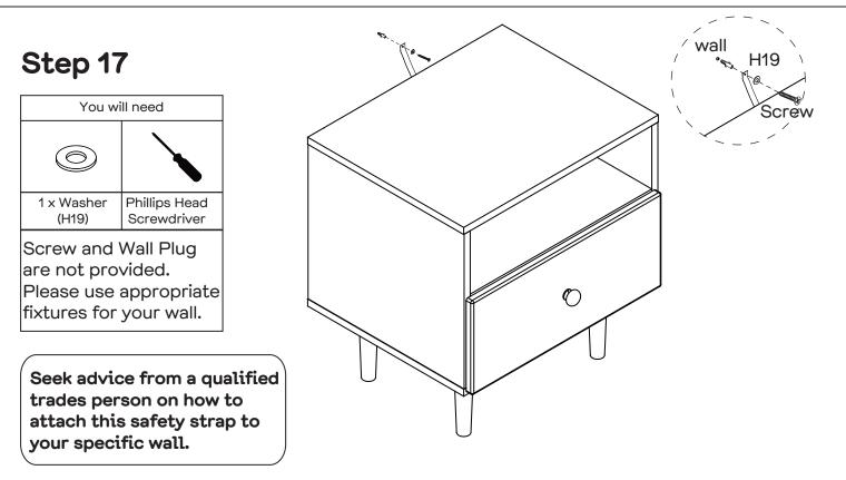
Move the unit to the final position, and attach the safety strap to the wall securely. Make sure it is firmly attached and snug fit.
