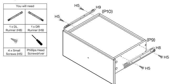
Attach 1 x DL Runner (H8) to the bottom of Left Drawer Side (P9) and 1 x DR Runner (H9) to the bottom of Right Drawer Side (P10) with  $4 \times$  Small Screws (H5) by tightening with the Phillips Head Screwdriver.
