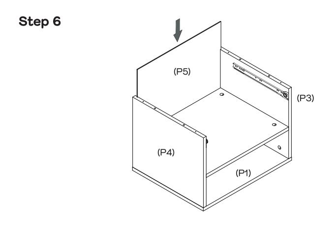
Slide Back Panel (P5) into the grooves of Left & Right Side Panel (P3 & P4) and Top panel (P1).
