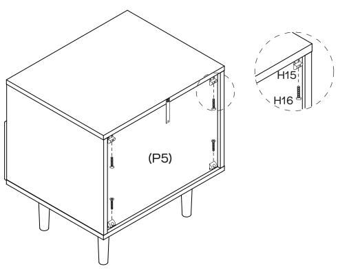
Secure Back Panel (P5) in place with  $4 \times$  Wedges (H15) using  $4 \times$  Wedge Screws (H16) by tightening with the Phillips Head Screwdriver.
