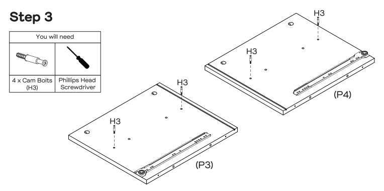
Attach 4 x Cam Bolts (H3) to Left & Right Side Panels (P3 & P4) by tightening with the Phillips Head Screwdriver.
