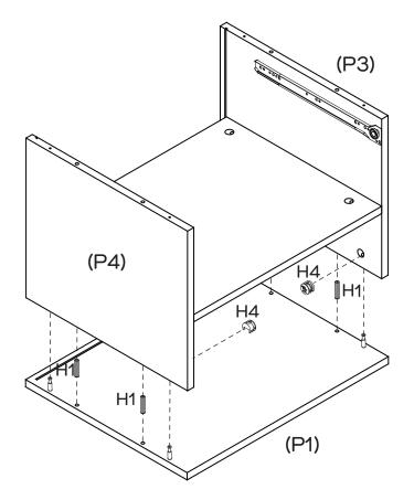
Insert 4 x Dowels (H1) into Top Panel (P1). Insert 4 x Cam Nuts (H4) into Left & Right Side Panels (P3 & P4) as shown. Rotate the cam nuts so the arrows point towards the incoming cam bolts. Attach Top Panel (P1) to Left & Right Side Panels (P3 & P4) by tightening all cam nuts with the Phillips Head Screwdriver.
