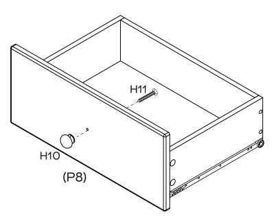
Attach 1  $\times$  Handle (H1O) to Drawer Front (P8) with 1  $\times$  Handle Screw (H11) by tightening with the Phillips Head Screwdriver.
