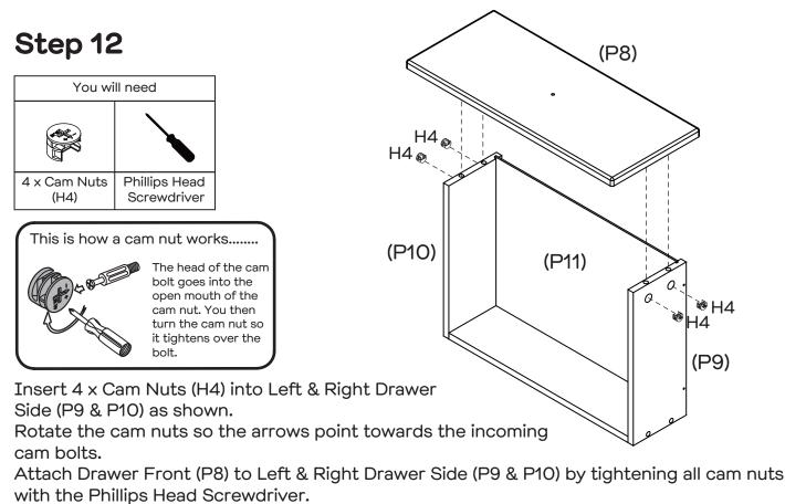
Ensure that the Drawer Base (P11) is slotted into the grooves of Drawer Front (P8).
