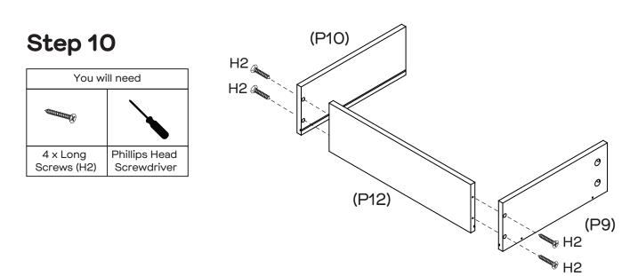
Attach Drawer Back (P12) to Left & Right Drawer Side (P9 & P10) with 4 x Long Screws (H2) by tightening with the Phillips Head Screwdriver.
