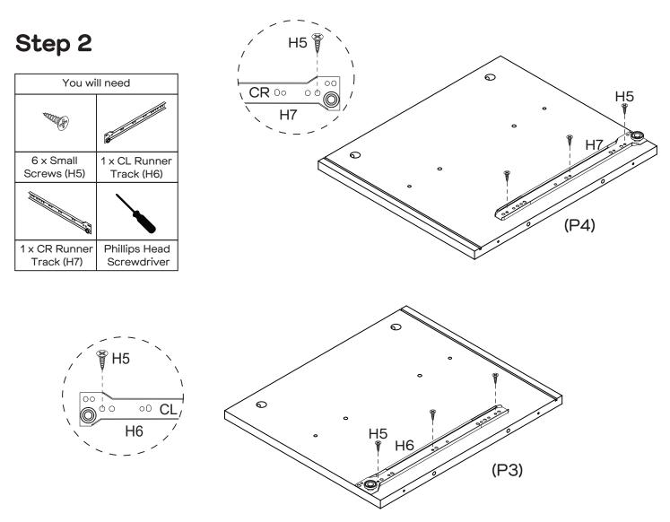
Attach 1 x CL Runner Track (H6) and 1 x CR Runner Track (H7) to Left & Right Side Panels (P3 & P4) with 6 x Small Screws (H5) by tightening with the Phillips Head Screwdriver.
