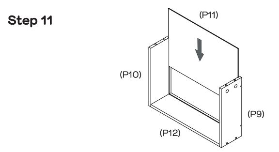
Slide the Drawer Bases (P11) into the grooves of Left & Right Drawer Sides (P9 & P10) and Drawer Back (P12) as shown.
