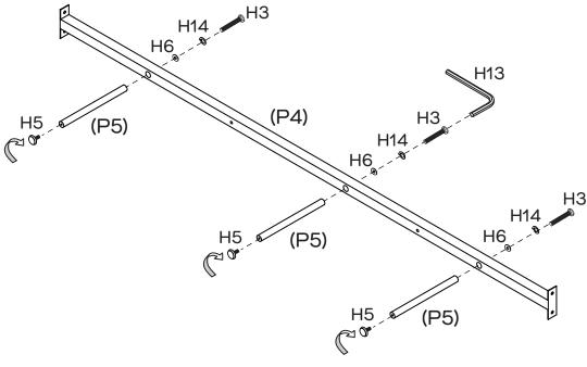
Attach 3 x support legs (P5) to centre rail (P4) using 3 x washers (H6), 3 x spring washers (H14) and 3 x long bolts (H3), tightening with the allen key (H13). Attach the 3 x adjusters (H5) to the  $3 \times 10^{-2}$  x support legs (P5) by turning clockwise.
