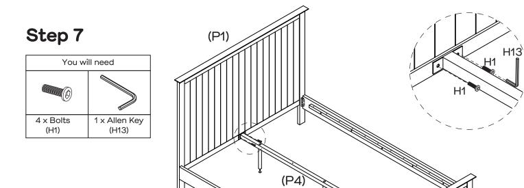
Attach centre rail (P4) to headboard (P1) and footboard (P2) using 4 x bolts (H1), tightening with the allen key (H13).
