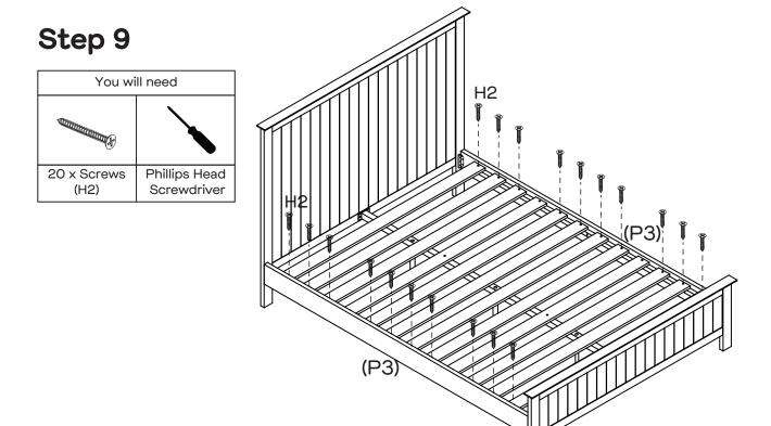
Attach the 10  $\times$  slats (P6) to the 2  $\times$  side rails (P3) using 20  $\times$  screws (H2), tightening with a phillips head screwdriver.
