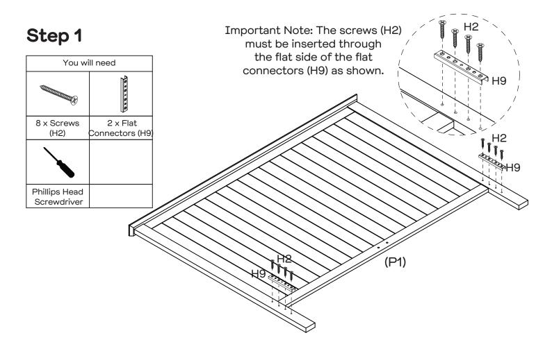
Attach 2 x flat connectors (H9) to headboard (P1) with 8 x screws (H2), tightening with a phillips head screwdriver.
