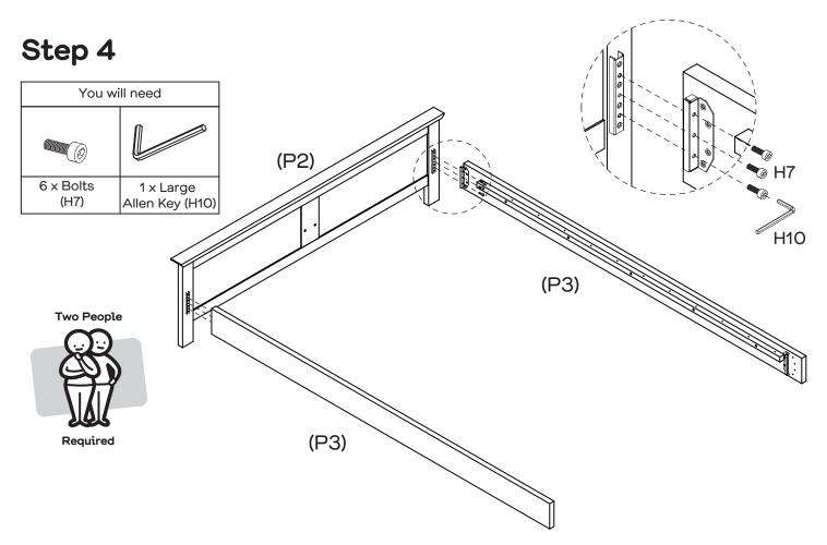
With assistance, attach the 2 x side panels (P3) to footboard (P2) with 6 x bolts (H7), tightening with the large allen key (H10).
