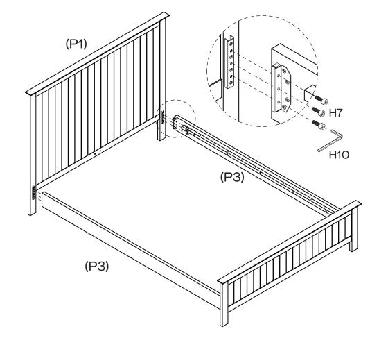
With assistance, attach the 2  $\times$  side panels (P3) to headboard (P1) using 6  $\times$  bolts (H7), tightening with the large allen key (H10).
