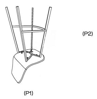
Place seat (P1) on a soft covered surface. Position frame (P2) over the seat (P1).
