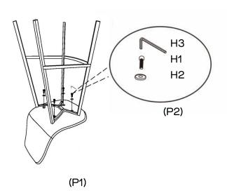
Align the holes on the frame (P2) to the holes on the seat (P1) Attach frame (P2) to seat (P1) using 4 x screws (H1) and 4 washers (H2), fully tightening using allen key (H3). Carefully turn the chair upright,
