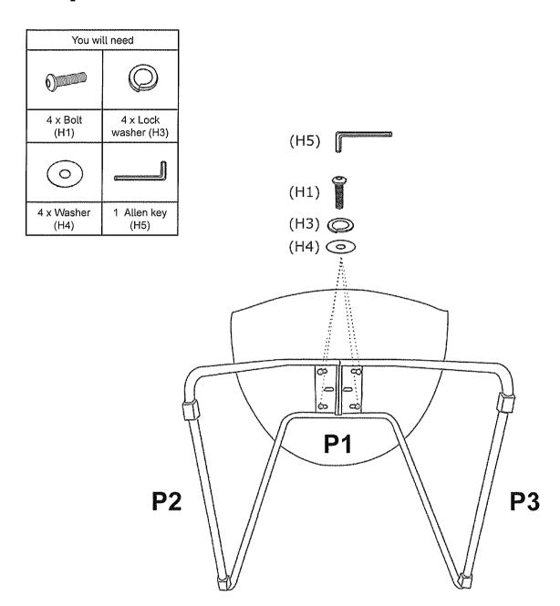
Mount the right and left legs (P2 and P3) to the chair seat (P1) as shown. Use the Allen key (H4) to mount bolts (H1), lock washers (H3) and washers (H4) into the chair seat (P1).
