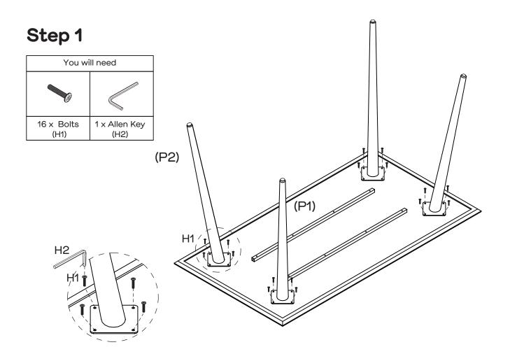
Attach 4  $\times$  Legs (P2) to Top Panel (P1) and secure with 16  $\times$  Bolts (H1). Tighten with an Allen Key (H2).
