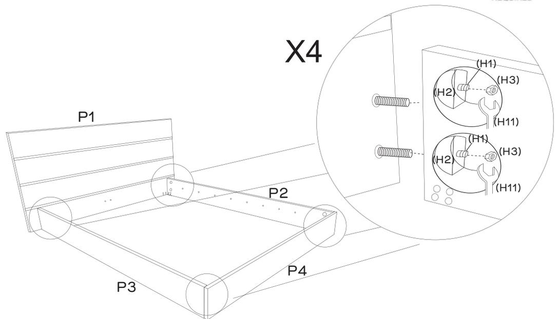
With assistance, carefully align and attach the right side panel (P2) between the headboard (P1) and footboard (P4). Secure together using 8 x half moon nuts (H2) and 8 x large nuts, tightening with the spanner (H11). Repeat this step to attach the left side panel (P3) to the headboard (P1) and footboard (P4).
