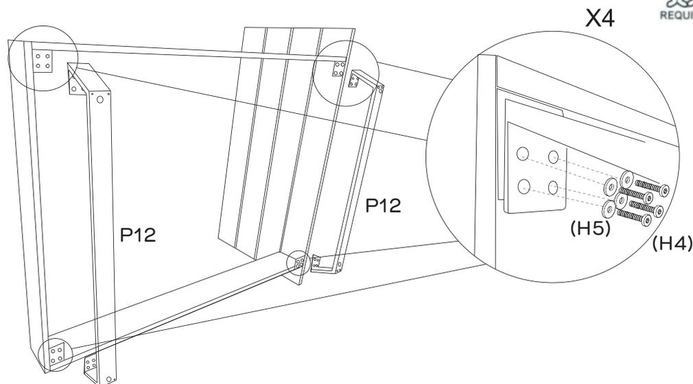
With assistance, carefully turn the bed over onto one side as pictured. Connect the 2 x legs (P12) to the connectors (H13,H14) using 16 x short bolts and 16 x washers (H5), completely tightening with the allen key (H10).
