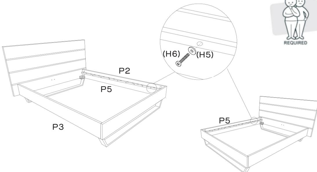
With assistance, carefully turn the bed upright again. Secure 1 x side rail (P5) to the right side panel (P2) using 8 x long bolts (H6) and 8 x washers (H5), tightening using allen key (H10). Repeat this step to secure the side rail (P5) to the left side panel (P3).
