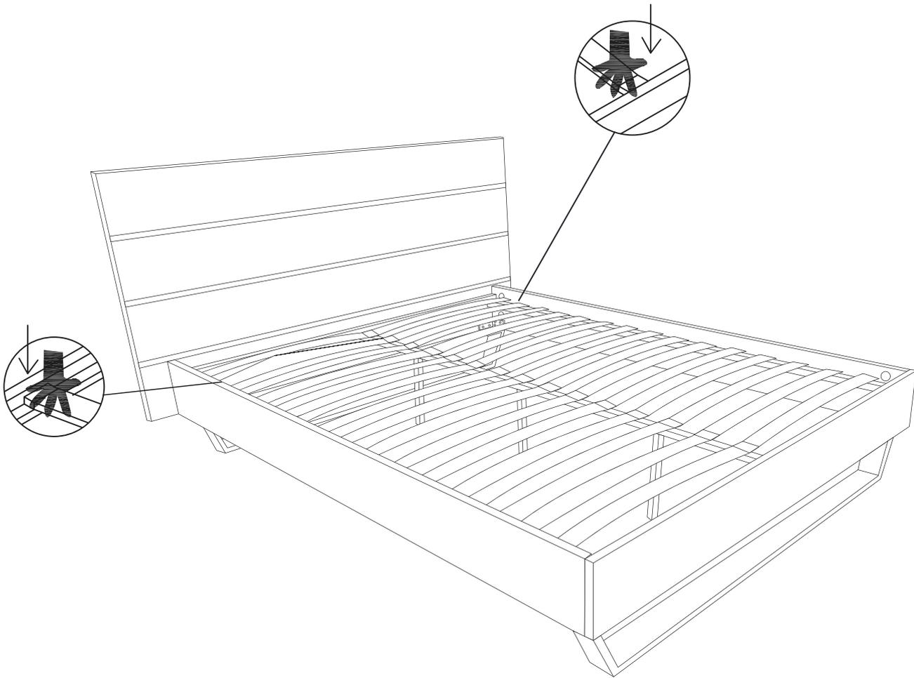
Lower onto the assembled bed frame, pushing in the plastic slat caps (P10) into the holes on the side rail, and the centre plastic slat caps (P9) into the holes on the centre rail (P8). Apply downward pressure until you feel the caps pop into place.
