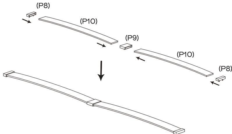
Attach 2 x plastic slat caps (P10), 2 x slats (P11) and 1 x centre plastic slat cap together as shown above.
