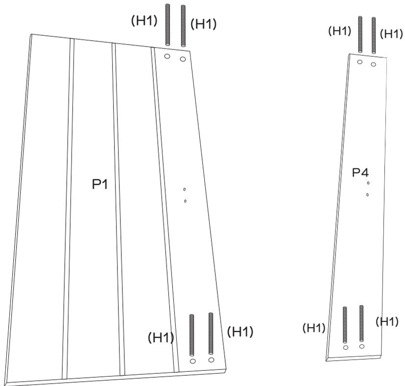
Attach 4 x threaded rods (H1) into the bottom of headboard (P1) and 4 x threaded rods (H1) into the footboard (P4) by turning clockwise until secure.
