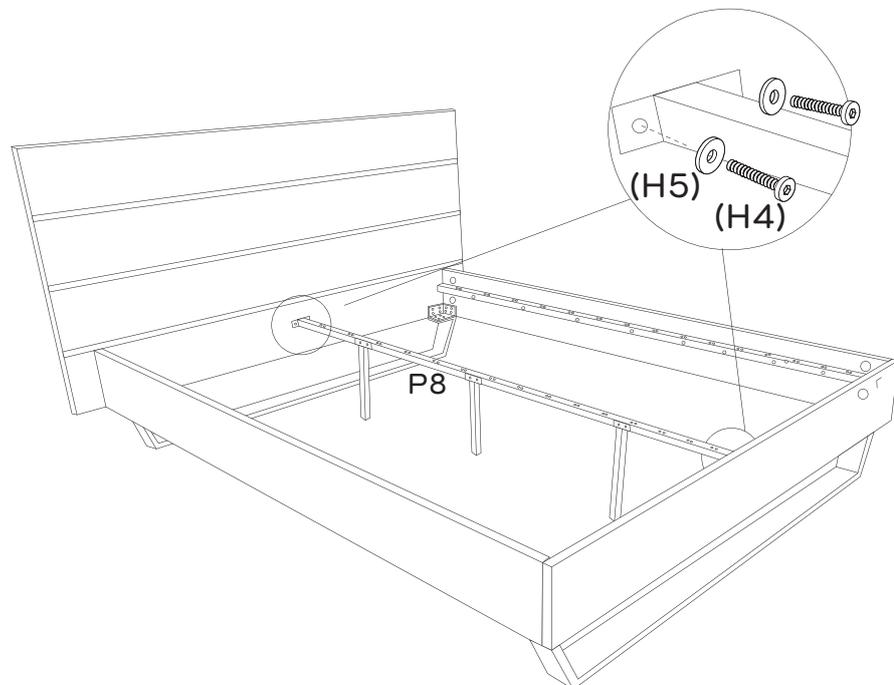
Align the centre rail (P8) between the headboard (P1) and footboard (P4) as shown. Secure the centre rail to the headboard (P1) and footboard (P4) using 4 x short bolts (H4) and 4 x washers (H5), tightening with the allen key (H10).
