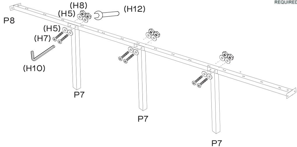
Attach the 3 x support legs (P7) to the centre rail (P8) using 6 x bolts (H7), 12 x washers (H5) and 6 x nuts (H8), tightening using the allen key (H10) and spanner (H12).
