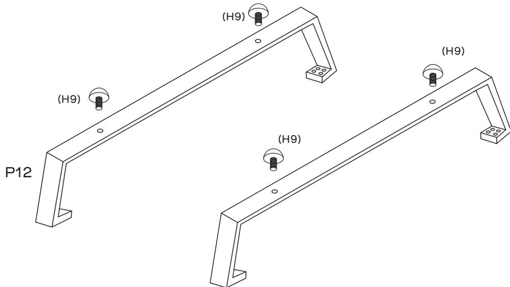
Screw in 4 x levelling feet (H9) into the 2 x legs (P12) by turning clockwise until secure. These can be adjusted as required to ensure assembled unit is level.
