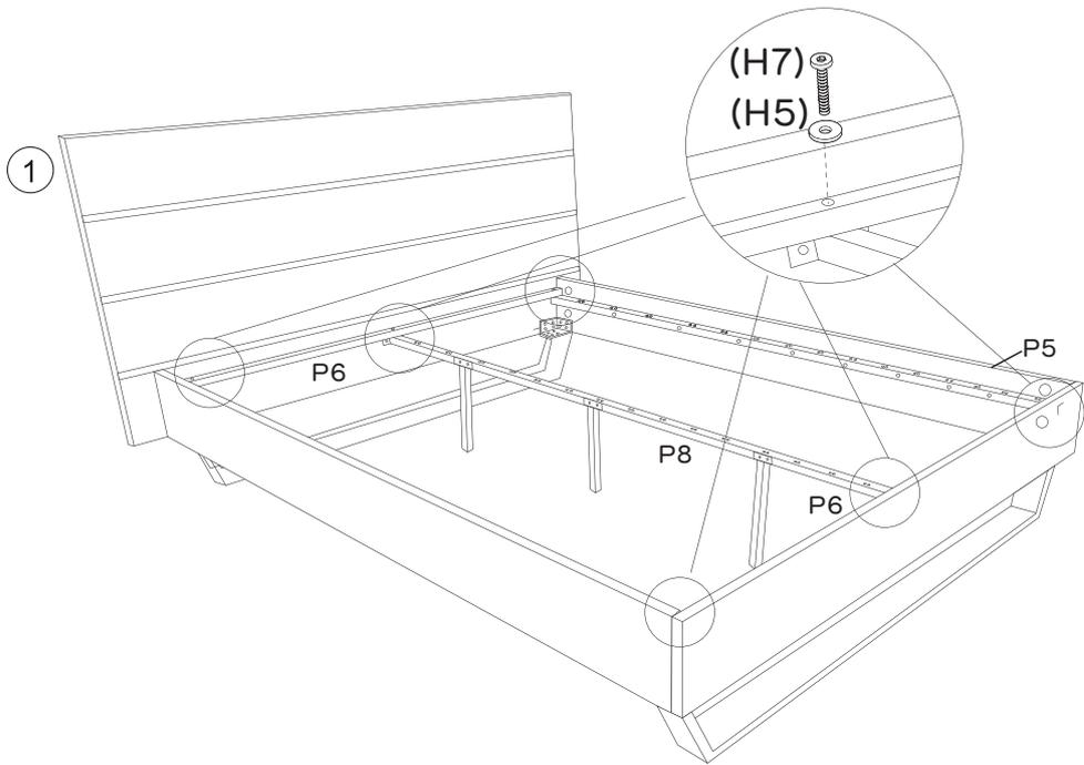
Attach the 2 x cross bars (P6) to the 2 x side rails (P5) and centre rail (P8) using 6 x bolts (H7) and 6 x washers (H5), tightening using the allen key (H10).
