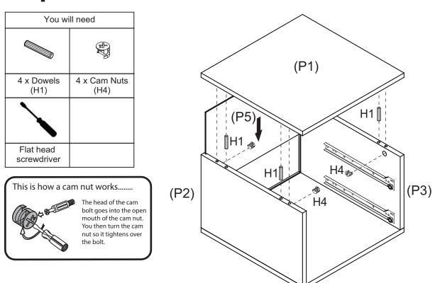
Insert Back Panel (P5) into the groove of Side Panels (P2, P3) and Bottom Panel (P4). Insert 4 x Dowels (H1) into Side Panels (P2, P3).
