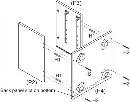
Insert 4 x Dowels (H1) into the holes of Side Panels (P2, P3).
