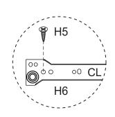
Attach 2 x CL Runner Tracks (H6) to Left Side Panel (P2) with 6 x Small Screws (H5).
