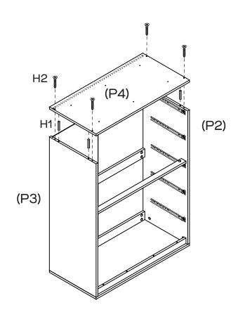
Attach Bottom Panel (P4) to Panels (P2,P3) with  $4 \times 1$  Dowels (H1), and secure with  $4 \times 1$  Long Screws (H2). Tighten with a Phillips Head Screwdriver.
