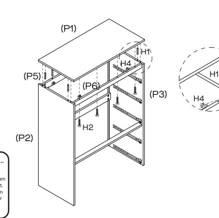
Attach Top Panel (P1) to Rails (P5,P6) and Panels (P2,P3) with 6 x Dowels (H1), and secure with 4 x Cam Nuts (H4) and 4 x Long Screws (H2). Tighten with a Phillips Head Screwdriver.
