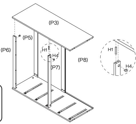
Attach Right Side Panel (P3) to Rails (P5,P6,P7,P8) with 1  $\times$  Dowel (H1), and secure with 6  $\times$  Cam Nuts (H4). Tighten with a Phillips Head Screwdriver.
