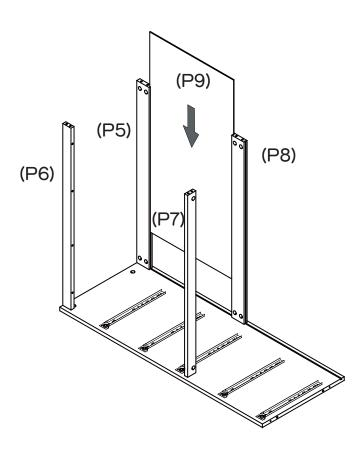
Slide remaining Back Panels (P9) into the grooves of Rails (P5,P8).
