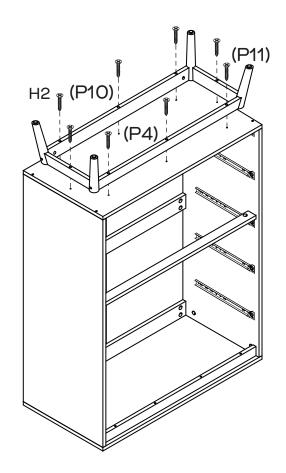
Attach Rails (P10,P11) to Bottom Panel (P4) with 8 x Long Screws (H2). Tighten with a Phillips Head Screwdriver.
