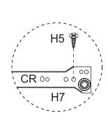
Attach 2 x CR Runner Tracks (H7) to Right Side Panel (P3) with 6 x Small Screws (H5).
