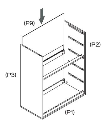
Slide Back Panel (P9) into the grooves between Panels (P2,P3) as shown.
