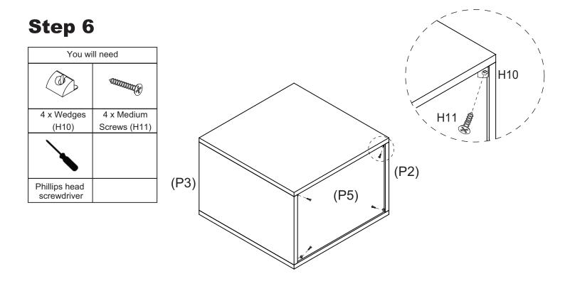
Secure Back Panel (P5) in place with 4 x Wedges (H10) using 4 x Medium Screws (H11).
