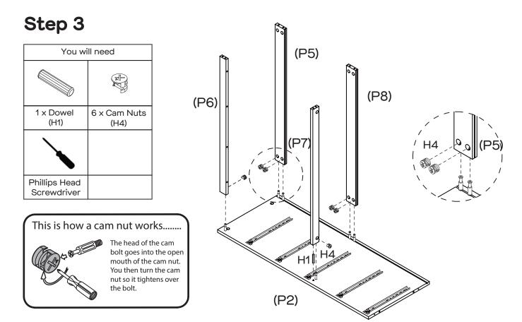
Attach Rails (P5,P6,P7,P8) to Left Side Panel (P2) with 1 x Dowel (H1), and secure with 6 x Cam Nuts (H4). Tighten with a Phillips Head Screwdriver.
