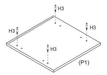
Attach 4 x Cam Bolts (H3) into Top Panel (P1) using a Phillips head screwdriver.
