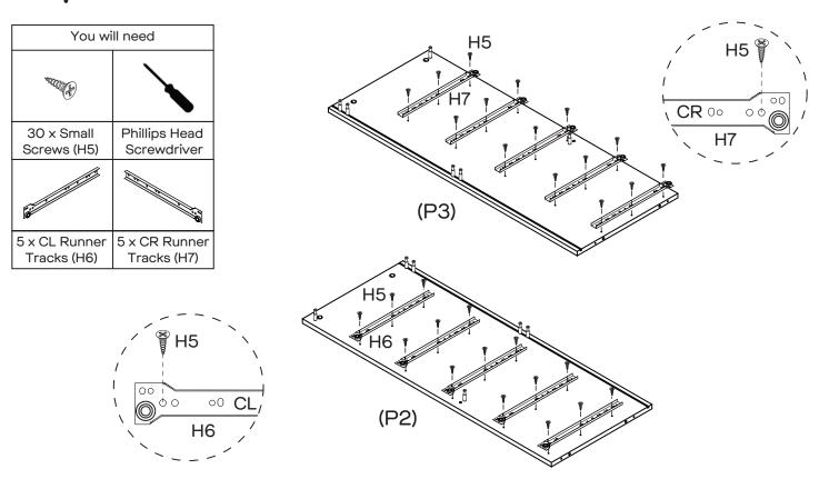
Attach  $5 \times CR$  Runner Track (H7) to Right Side Panel (P3) with  $15 \times Small$  Screws (H5). Attach  $5 \times CL$  Runner Track (H6) to Left Side Panel (P2) with  $15 \times Small$  Screws (H5). Tighten with a Phillips Head Screwdriver.
