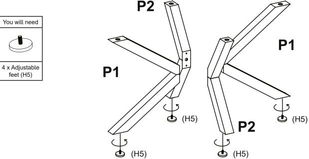
Attach adjustable feet (H5) to legs (P1 and P2).
