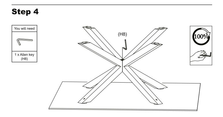
Make sure the table is level, then fully tighten all bolts (H2) by using allen key (H8).
