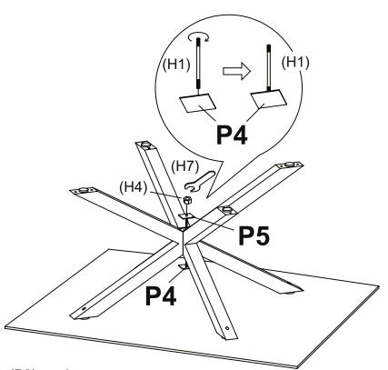
Add Metal stick (H1) to Center block (P3), and attach Caps (P4 and P5). Tighten the Caps (P4 and P5) by using nuts (H4) and Spanner (H7).
