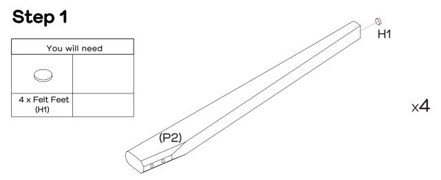
Attach 1 x felt foot (H1) onto each leg (P2) as shown.
