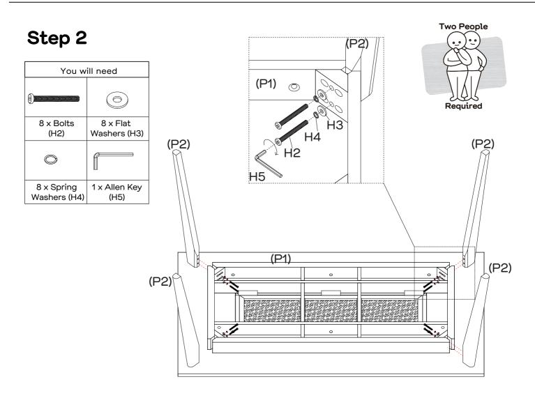
Attach 1 x leg (P2) onto top panel (P1), using 2 x bolts (H2), 2 x spring washers (H4) and 2 x flat washers (H3). Tighten the bolts with allen key (H5). Repeat this step for the other  $3 \times 10^{12}$  key (P2).
