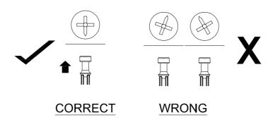
When fitting cam lock, ensure starting position is correct before you insert connecting quickfit.
