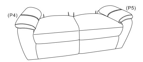
Zip the left arm (P4) to the left side of the seat (P1). Then peel the velcro cover off and stick the arm down to fix it into position. Repeat this step for the right arm (P5) to the right side of the seat (P1).
