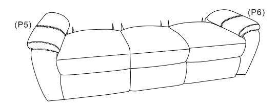
Zip the left arm (P5) to the left side of the seat (P1). Then peel the velcro cover off and stick the arm down to fix it into position. Repeat this step for the right arm (P6) to the right side of the seat (P1).
