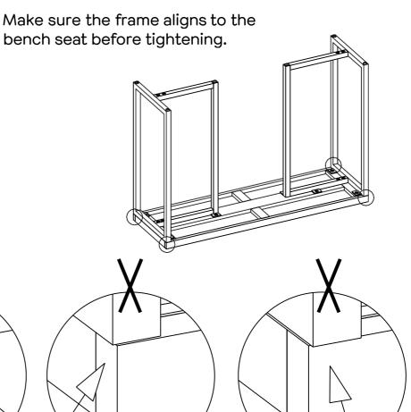
Align the leg frames to bench seat (P1) as shown. Tighten the bolts using Allen key (H3).
