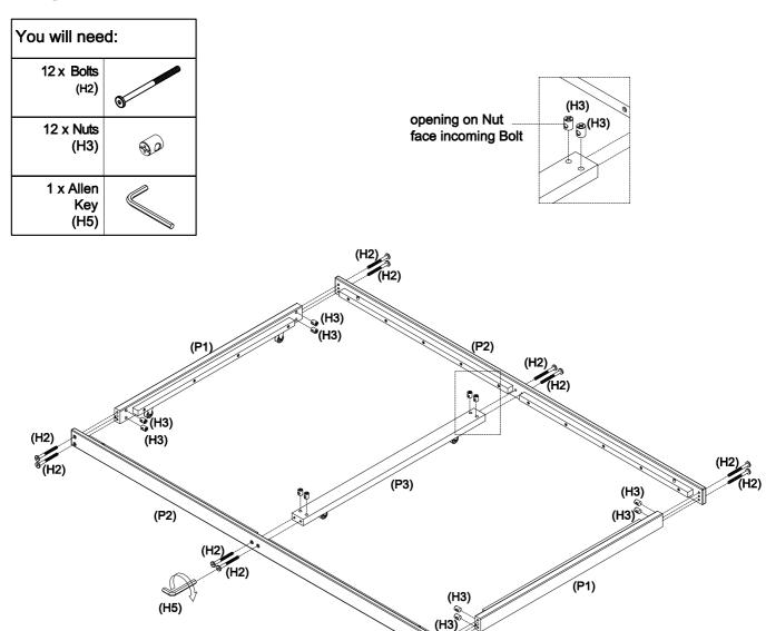
Attach 2 x side rails (P2) to the 2 x end rails (P1) and centre rail (P3). Insert 12 x nuts (H3) into the 2 x end rails (P1) and centre rail (P3) and make sure the opening on the nut is facing incoming bolts. Insert 12 x bolts (H2) and use an allen key (H5) and turn clockwise to tighten.
