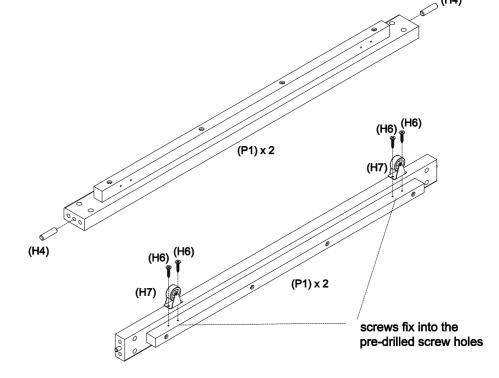
Insert 4 x wooden dowels (H4) into the 2 x end rails (P1). Fix 4 x wheels (H7) to the 2 x end rails (P1) by using 8 x small wood screws (H6), tightening with a phillips head screwdriver.
