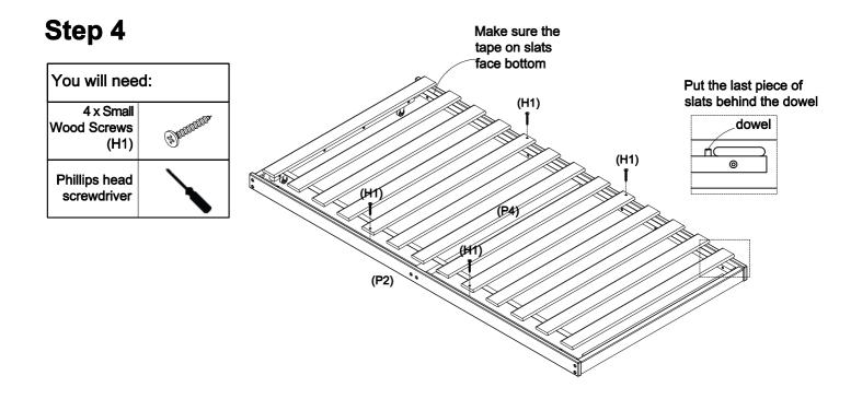
Put the slats (P4) on the bed and slot the end slats next to the dowels. Fix the slats on to the 2 x side rails (P2) by using 4 x large wood screws (H1) and a phillips head screwdriver.
