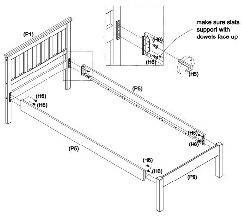
Connect the 2 x side rails (P5) to the headboard (P1) and footboard (P6), using an allen key (H5), turn 8 x small bolts (H6) clockwise to fix.
