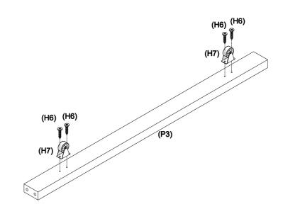
Fix 2 x wheels (H7) to the centre rail (P3) by using 4 x small wood screws (H6), tightening with a phillips head screwdriver.
