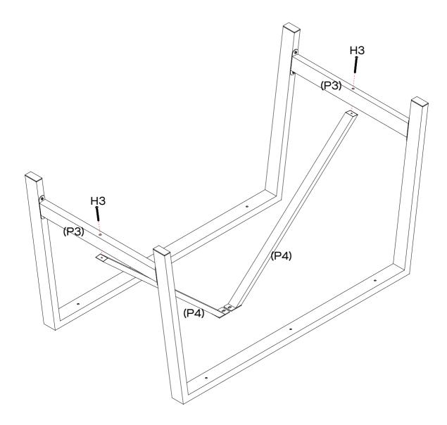
Attach support braces (P4) to bottom rails (P3) with  $2 \times bolts$  (H3), tighten the bolts with Allen key (H5).
