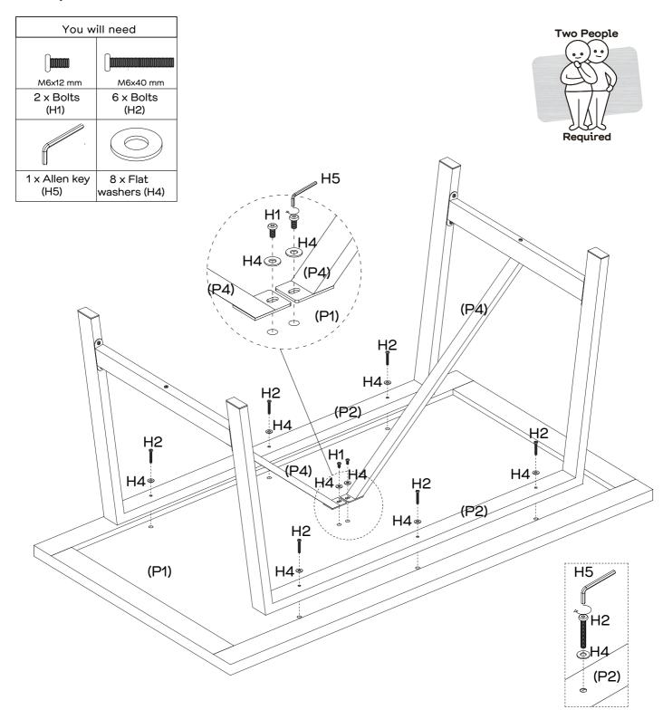
Position the assembled frame onto top panel (P1).
