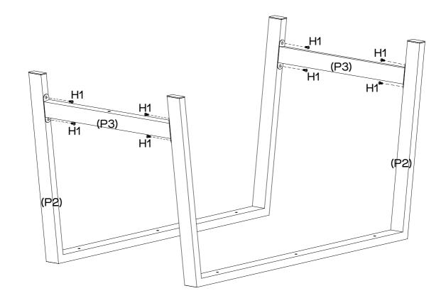
Fasten bottom rails (P3) to leg frames (P2) with  $8 \times 10^{-2}$  with  $8 \times 10^{-2}$  using Allen key (H5) as shown.
