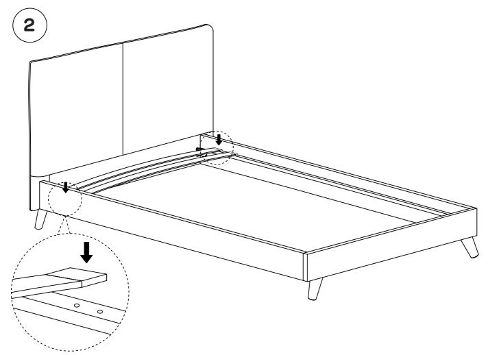
Attach the assembled slats by pressing down the connectors (P7) into the holes on  $2 \times 3$  side rails (P6) until they lock.
