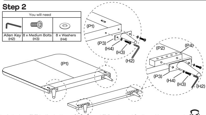
Attach 4 x legs (P3) to the bottom of headboard (P1) and wood footboard legs supports (P4) with 8 x medium bolts (H3) and 8 x washers (H4) by using allen key (H2).
