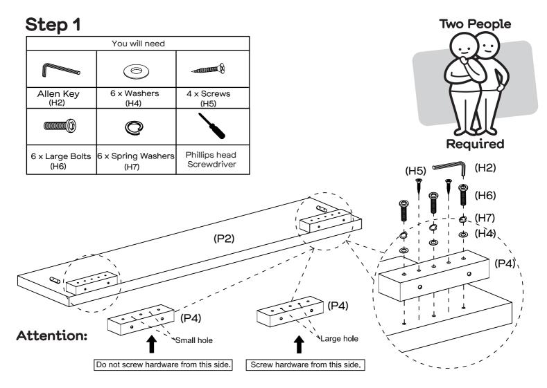
Attach 2 x wood footboard legs supports (P4) to the footboard (P2) with 6 x large bolts (H7), 6 x washers (H4) and 6 x spring washers (H8) by using allen key (H2). Then screw the 4 x screws (H5) by using a phillips head screwdriver (not provided).
