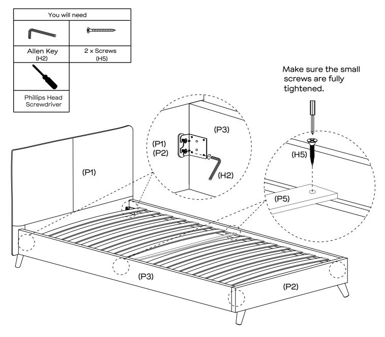
Attach the timber cross rail (P5) to the side rails (P3) with  $2 \times$  screws (H5), fully tighten using a phillips head screwdriver. You may now fully tighten all the bolts on the headboard (P1) and footboard (P2) to  $2 \times$  side rails (P3).
