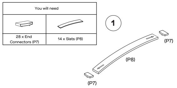
Attach 2 x end connectors (P7) to 1 x slat (P8) together as shown.
