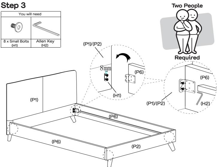
Install the bolts (H1) to the brackets by using allen key (H2) as shown, do not tighten the bolts and keep them 8mm loose. Then attach 2 x side rails (P6) to headboard (P1) and footboard (P2) by slotting the bracket on the side rails (P6) over the bolt as shown. Please do not tighten bolts until step 5.
