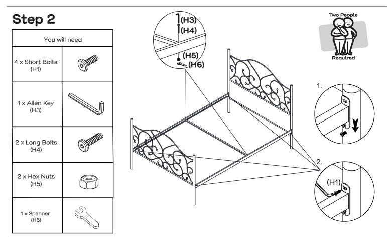
Attach the 2 x side rails (P4) to the headboard (P1) and footboard (P2). Slot the side rails onto the bolts as shown and insert 4 x short bolts (H1) into the top holes with the allen key (H3).
