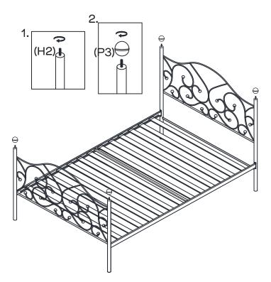
Screw 4 x headless bolts (H2) into the posts of the headboard (P1) and footboard (P2). Then attach the 4 x finials (P3) by rotating clockwise as shown.
