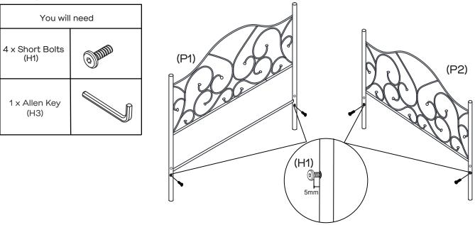
Insert 4  $\times$  short bolts (H1) into the bottom holes of the headboard (P1) and footboard (P2) using the allen key (H3). Do not fully tighten the bolts and leave a gap of 5mm as shown.
