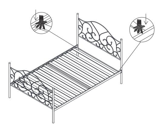
Lower the slat (P7) with the end connectors (P6) to the side rails (P4). Ensure the plastic slat caps are in place over the side rail holes and apply downward pressure until the plastic slat caps are fully inserted into the rails. Repeat for every bed slat until finished.
