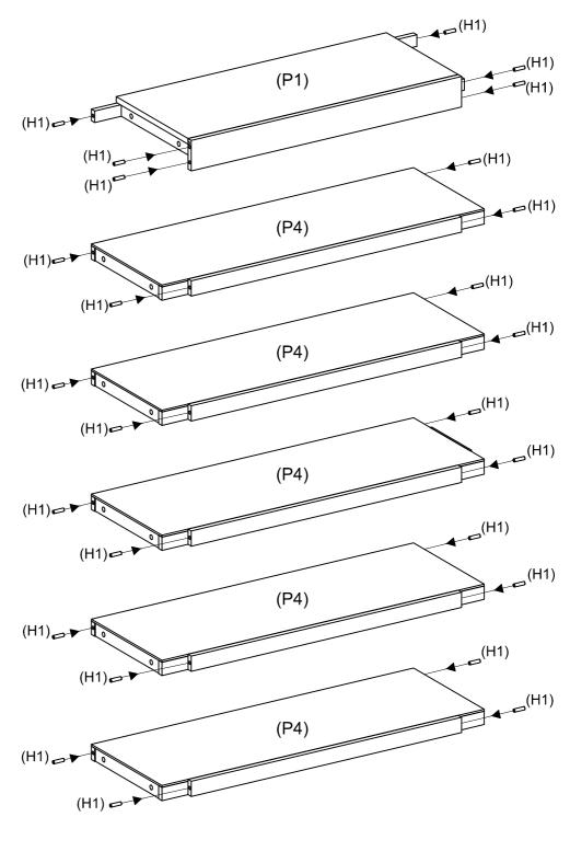
Insert 26 x Wooden Dowels (H1) into Top panel (P1) and Shelf panels (P4x5) as shown. Use the mallet to gently tap the end of the Wooden Dowels into place.
