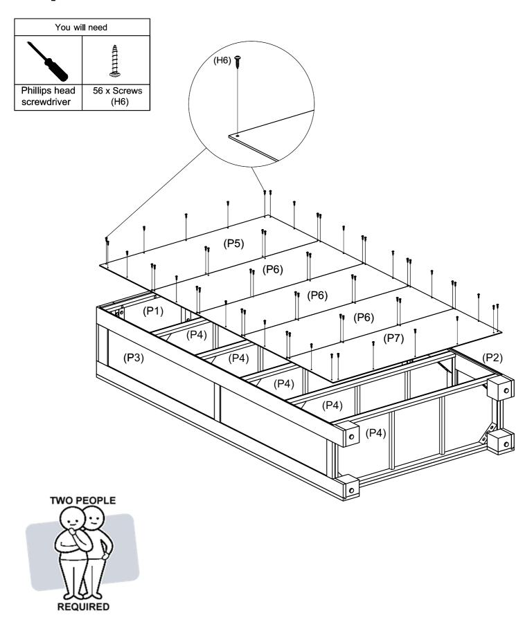
Fix Top Back panel (P5), Back panels (P6x3) and Bottom Back panel (P7) to Left & Right Side frames (P2) &(P3) and Top panel (P1) & Bottom Shelf panel (P4) with 56 x Screws (H6) by tightening with the Phillips Head Screwdriver as show. Ensure all back panels fit into the frame and are aligned before securing.
