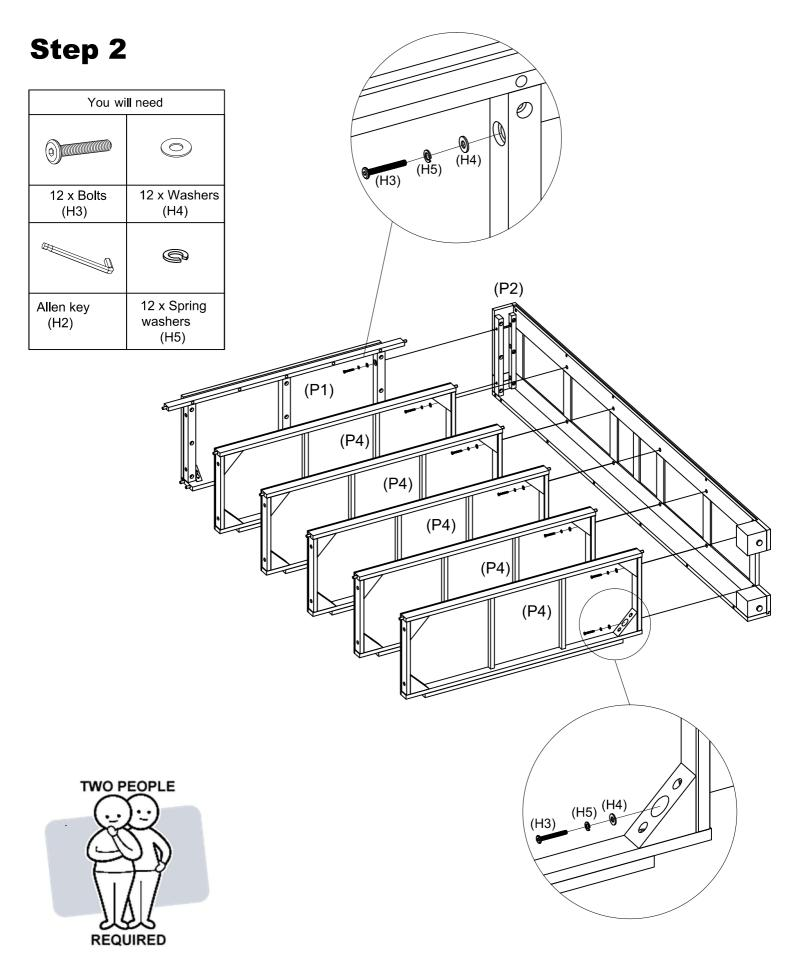
Secure Top panel (P1) and Shelf panels (P4x5) to Left Side frame (P2) with 12 x Bolts (H3), 12 x Washers (H4) and 12 x Spring Washers (H5) and tighten with the Allen Key (H2) as shown.
