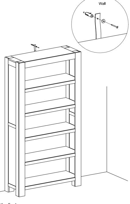
Move the bookcase to the final position and attach the safety strap to the wall securely
