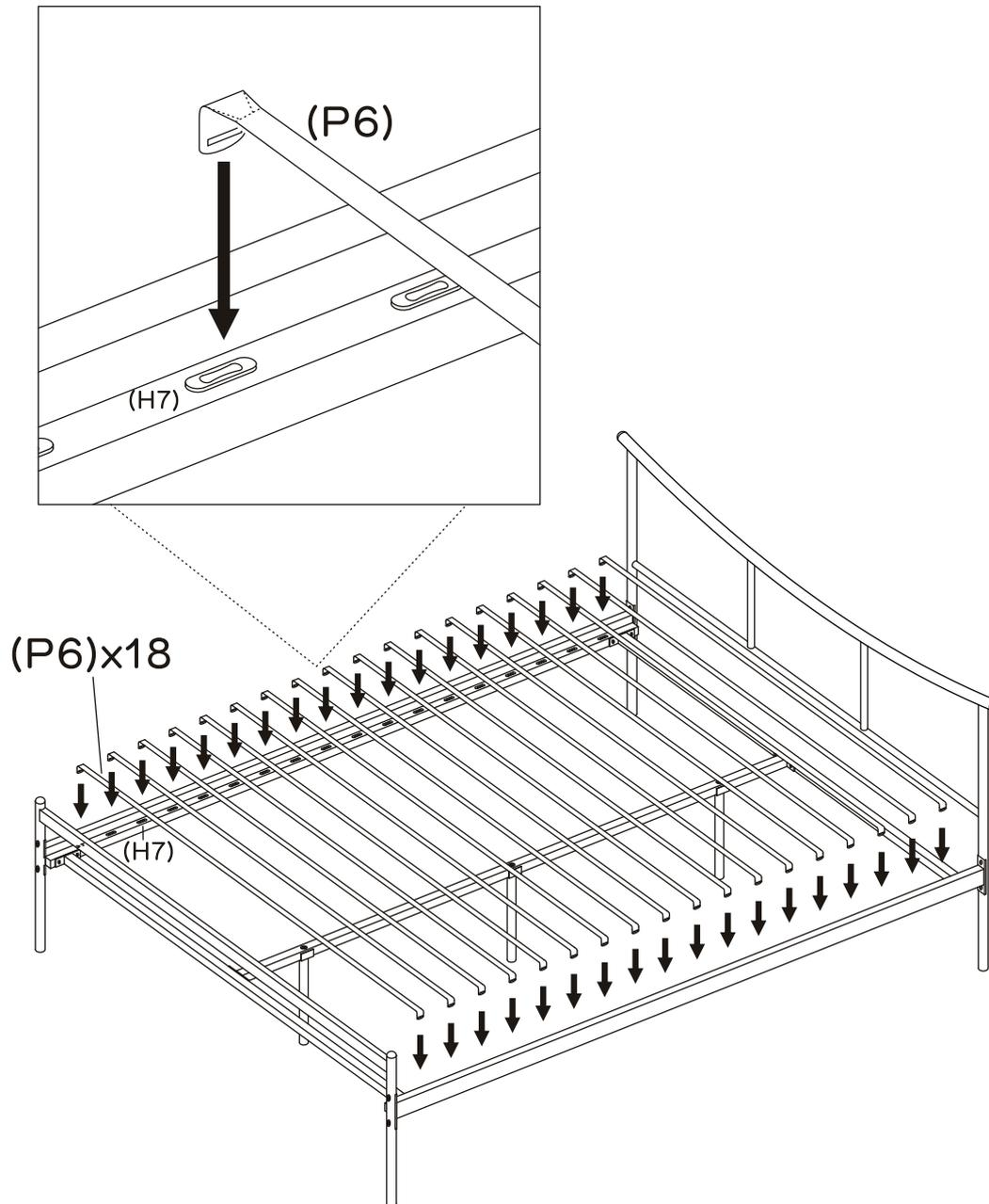
Insert the 18 x slats (P6) into the holes on the plastic connectors (H7) in the side rails (P3).
