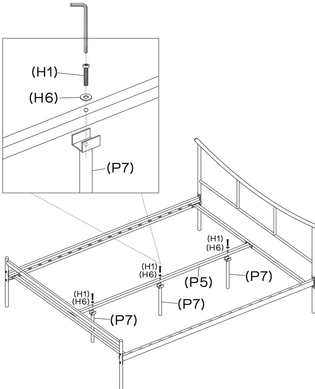
Attach the 3 x support legs (P7) to the centre rail (P5) with 3 x flat washers (H6) and 3 x bolts (H1), tightening with an allen key (H8).
