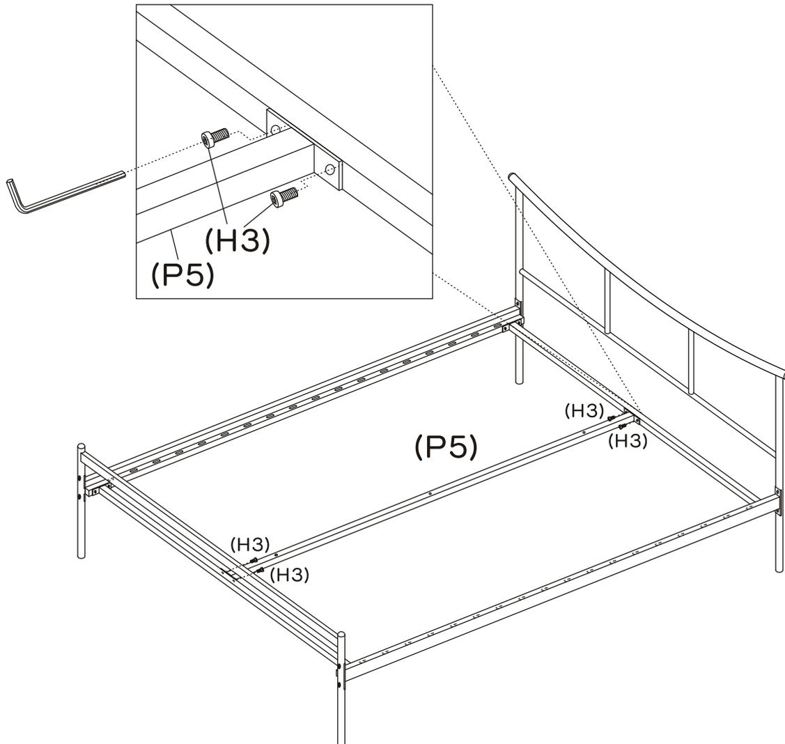
Attach the centre rail (P5) to the 2 x head/foot rails (P4) with 4 x bolts (H3) using an allen key (H8).
