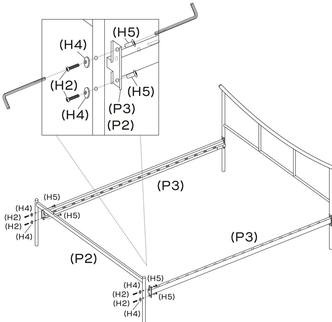
Attach 1 x side rail (P3) to the footboard (P2) with 2 x sleeve nuts (H5), 2 x bolts (H2) and 2 x washers (H4) using 2 x allen keys (H8).
