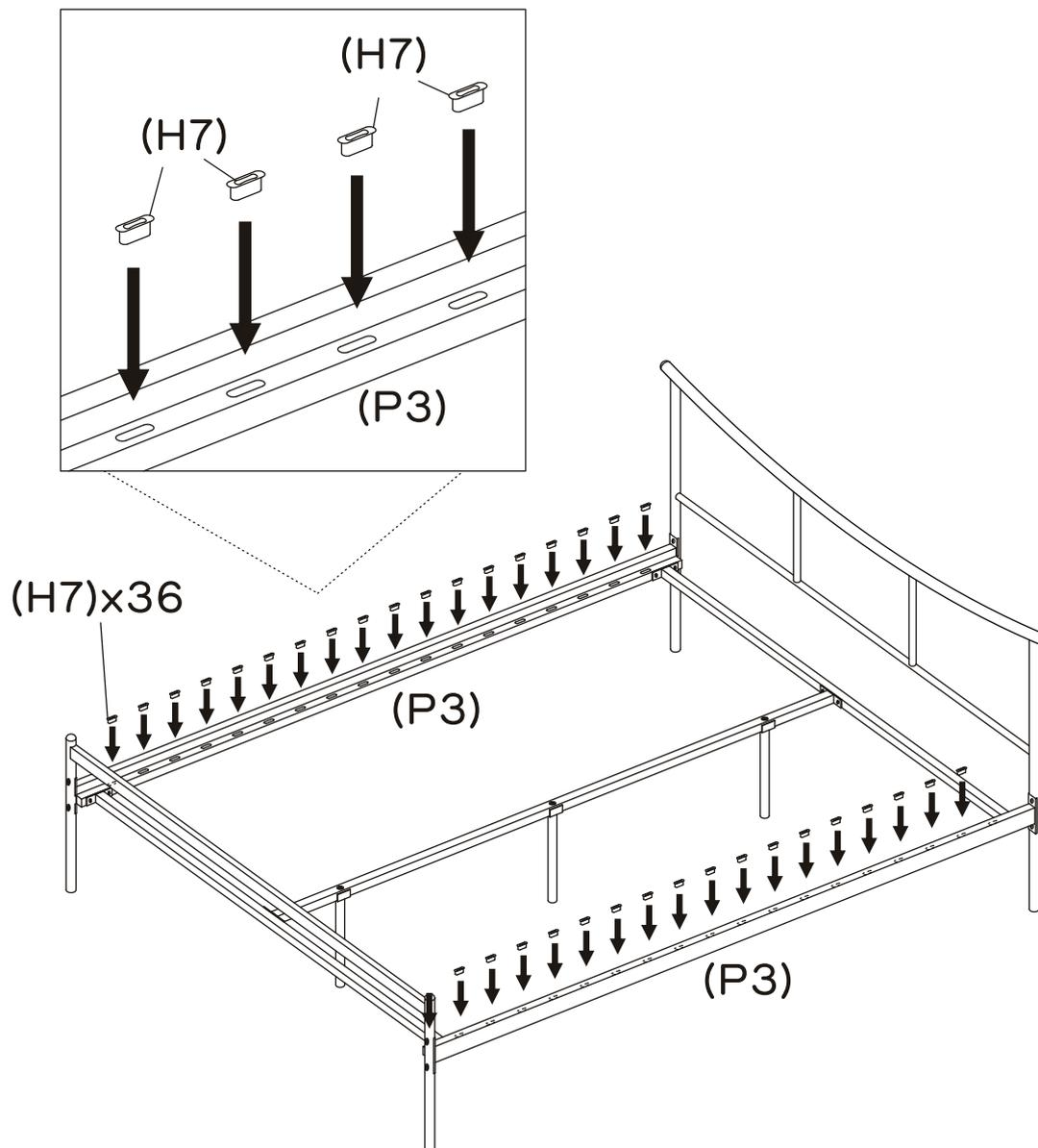
Insert 36 x plastic connectors (H7) into the holes on the 2 x side rails (P3).
