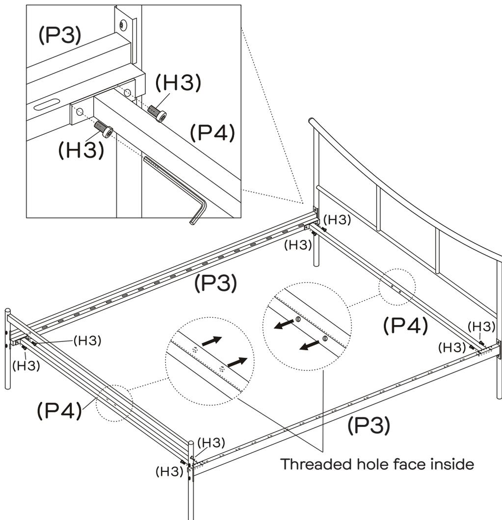
Attach 2 x head/foot rails (P4) to the side rails (P3) with 8 x bolts (H3) using an allen key (H8).
