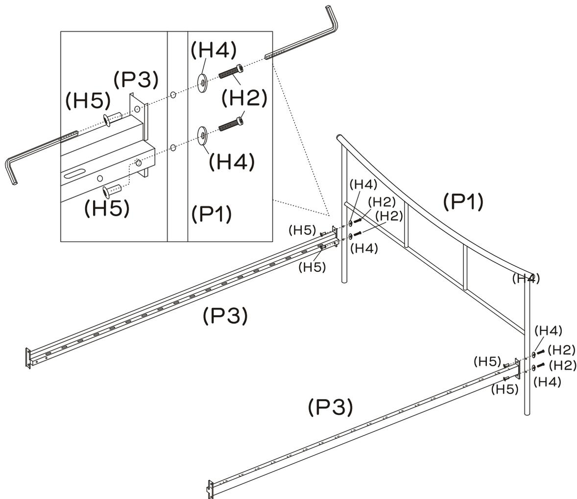
Attach 1 x side rail (P3) to headboard (P1) with 2 x sleeve nuts (H5), 2 x bolts (H2) and 2 x washers (H4) using 2 x allen keys (H8).
