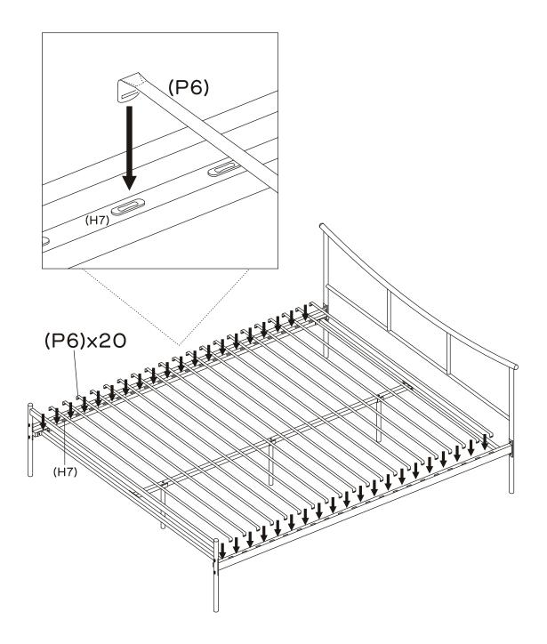
Insert the 20 x slats (P6) into the holes on the plastic connectors (H7) in the side rails (P3).
