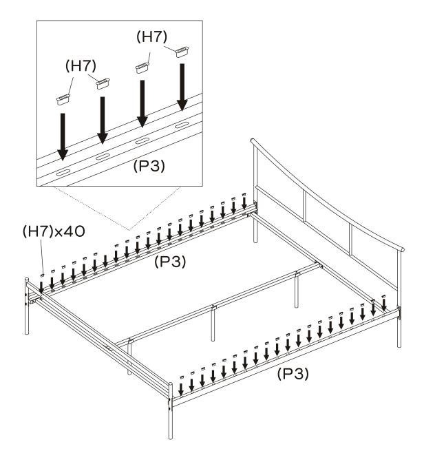
Insert 40 x plastic connectors (H7) into the holes on the  $2 \times side$  rails (P3).
