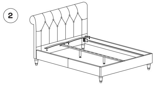
Insert the full slat into the side rail and centre rail one by one.
