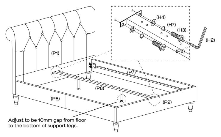
Slot the centre rail (P8) into the headboard (P1) and footboard (P2). Rotate  $4 \times$  bolts (H3),  $4 \times$  washers (H4) and  $4 \times$  spring washers (H7) to the headboard (P1) and footboard (P2) by using alley key (H2). No need to tighten bolts until step 7.
