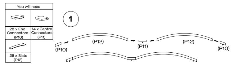
Push 2 end connectors (P10), 2 pcs slats (P12) and a centre connector (P11) together.
