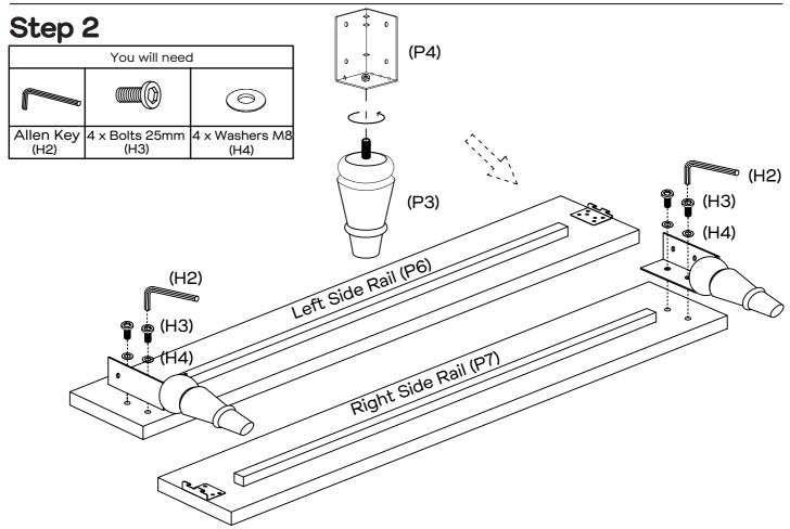
Attach footboard legs (P3) to the bottom of the bracket (P4) and rotate as shown. Then, attach brackets (P4) to the left side rail (P6) with  $2 \times bolts$  (H3) and  $2 \times bolts$  (H4) by using the allen key (H2). Repeat for the right side rail (P7). Do not fully tighten the bolts (H3) until step 7.
