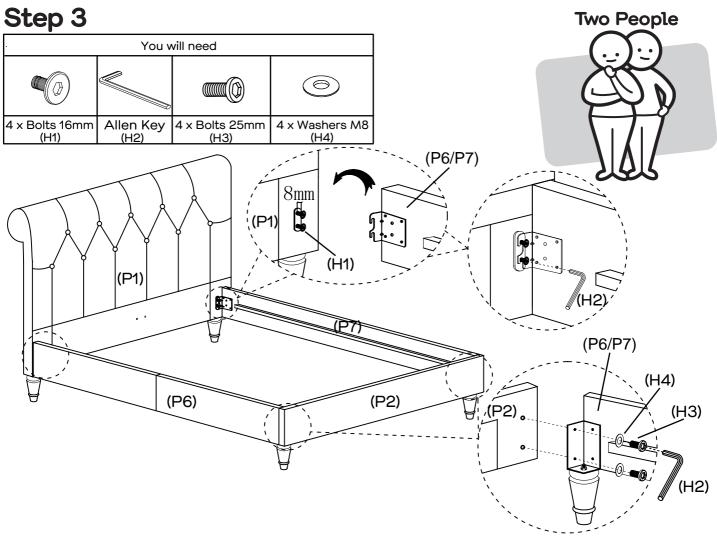
Install 4 x bolts (H1) to the brackets of headboard (P1) by using allen key (H2) as shown, do not tighten the bolts and keep them 8mm loose. Then attach the side rails (P6/P7) to the headboard (P1) over the bolts (H1) as shown. Finally, attach the side rails (P6/P7) to the footboard (P2) with 4 x bolts (H3) and 4 x washers (H4) by using the allen key (H2). Do not fully tighten the bolts (H3) until step 7.
