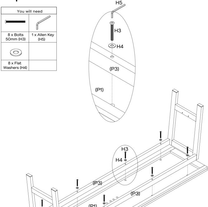
Position the assembled frame onto top panel (P1).
