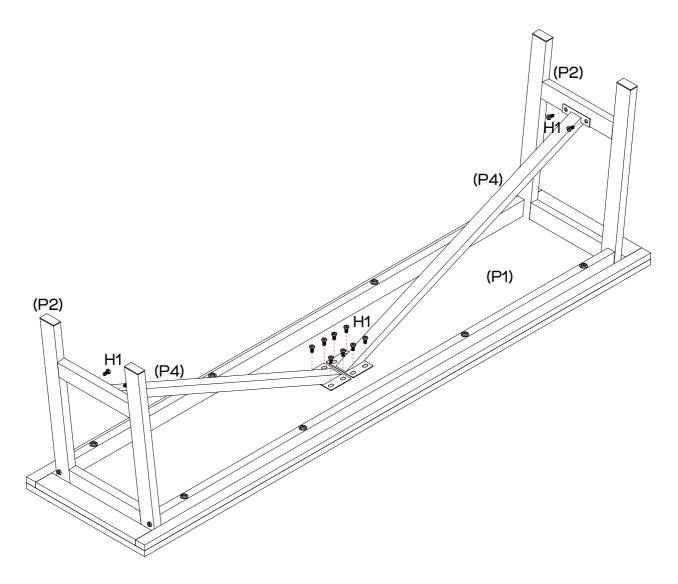
Attach 2  $\times$  support rails (P4) onto leg frames (P2) and top panel (P1) with 6  $\times$  bolts (H1) as shown, tighten with allen key (H5). With help, turn over the bench.
