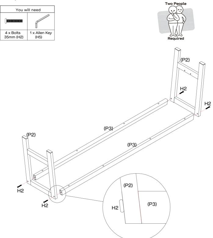
Attach 2 x top rails (P3) to 2 x leg frames (P2) with 4 x bolts (H2) using allen key (H5) as shown.
