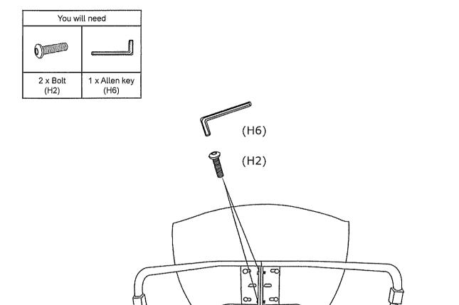
Tighten the right and left legs (P2 and P3) together using bolt (H2) and Allen Key (H6).
