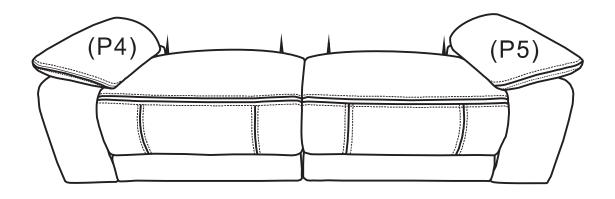
Zip the left arm (P4) to the left side of the seat (P1). Then peel the velcro cover off and stick the arm down to fix it into position. Repeat this step for the right arm (P5) to the right side of the seat (P1).
