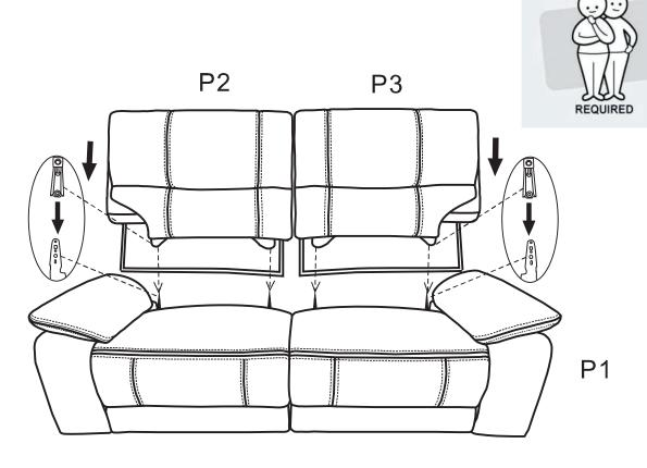
Attach the left back (P2) and right back (P3) to the seat base (P1) as shown. Make sure the clips are well aligned before inserting the back. Ensure the backs (P2 & P3) are fully slotted on the brackets before use.
