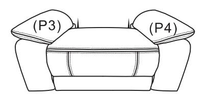
Zip the left arm (P3) to the left side of the seat (P1). Then peel the velcro cover off and stick the arm down to fix it into position. Repeat this step for the right arm (P4) to the right side of the seat (P1).
