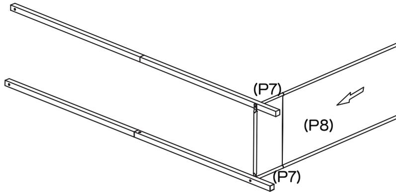
Slide the Fabric Base (P8) over Base Supports (P7x2) as shown.
