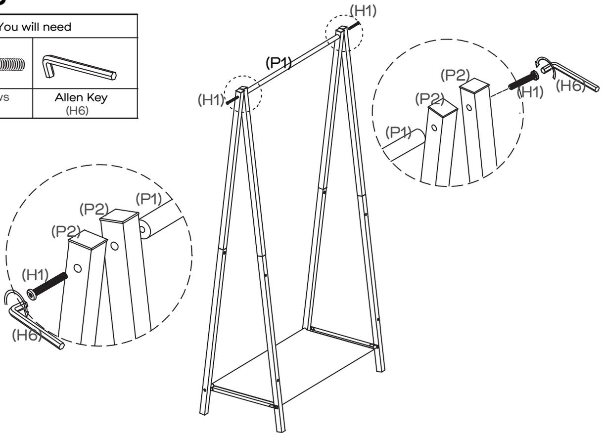
Secure Hanging Rail (P1) to Top Frames (P2) with 2 x Screws (H1) by tightening with the Allen Key (H6).
