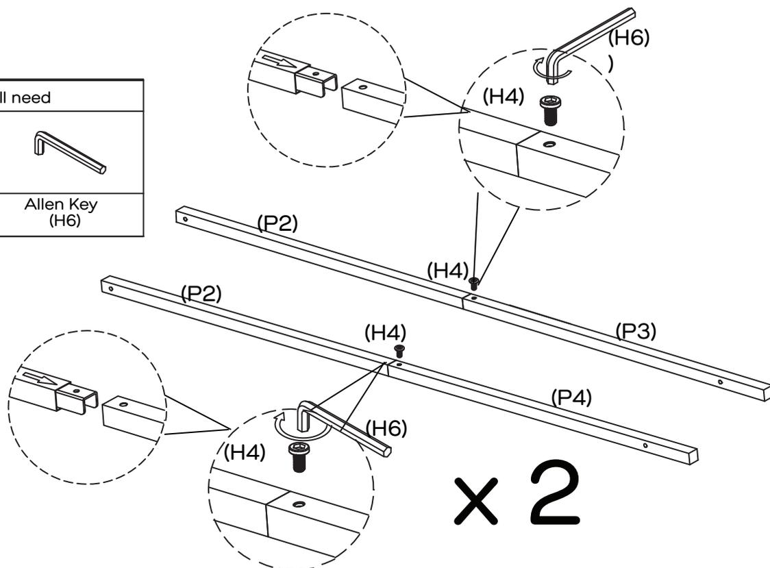
Attach Top Frames (P2x2) to Lower Back & Front Frames (P3&P4) with 2 x Screws (H4) by tightening with the Allen Key (H6).
