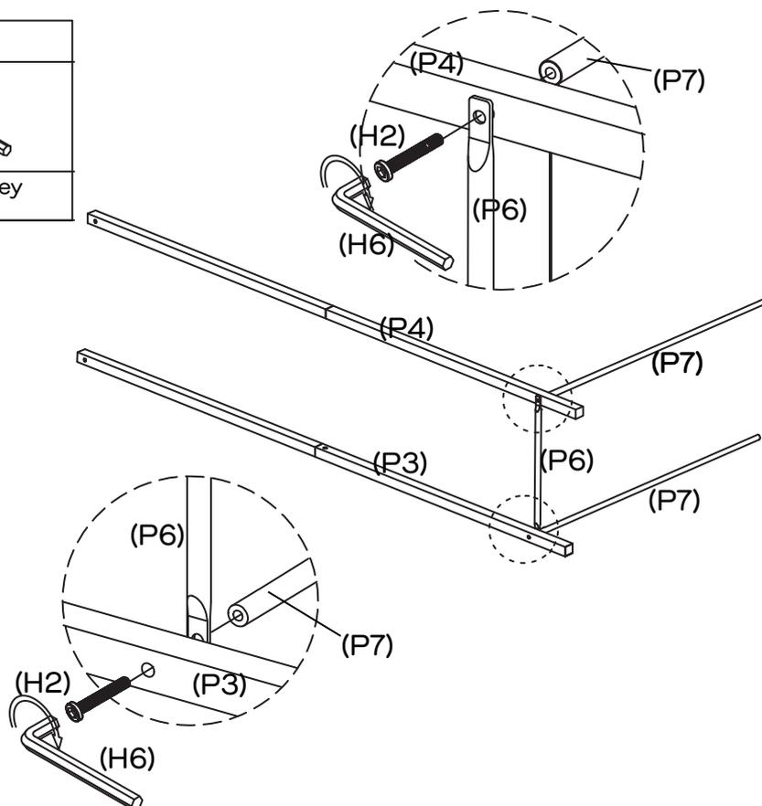
Secure Side Support (P6) and Base Supports (P7x2) to Lower Back & Front Frames (P3&P4) with 2 x Screws (H2) by tightening with the Allen Key (H6).
