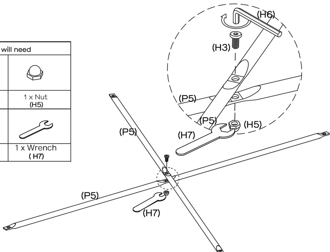
Secure Back Supports (P5x2) together as shown with 1 x Nut (H5) and 1 x Screw (H3) by tightening with the Allen Key (H6) and Wrench (H7).
