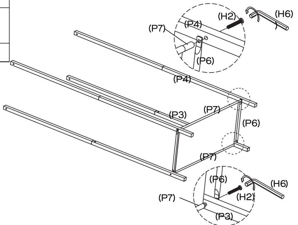
Secure Side Support (P6) and Lower Back & Front Frames (P3&P4) to Base Supports (P7x2) to with 2 x Screws (H2) by tightening with the Allen Key (H6).
