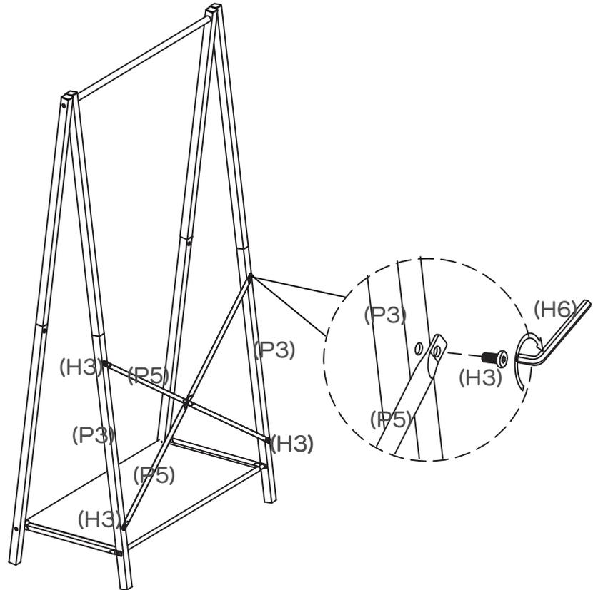
Secure Back Supports (P5x2) to Lower Back Frames (P3x2) with 4 x Screws (H3) by tightening with the Allen Key (H6).
