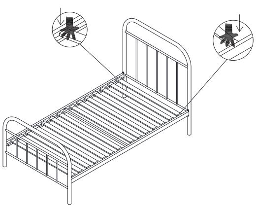
Lower the slat (P6) with the end connectors (P5) to the side rails (P3). Ensure the plastic slat caps are in place over the side rail holes and apply downward pressure until the plastic slat caps are fully inserted into the rails. Repeat for every bed slat until finished.
