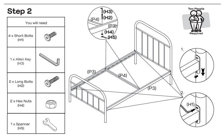
Attach the 2 x side rails (P3) to the headboard (P1) and footboard (P2). Slot the side rails onto the bolts as shown and insert 4 x short bolts (H1) into the top holes with the allen key (H3).
