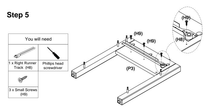
Fix the right runner track (H8) to the right side panel (P3) with 3 x small screws (H9) by tightening with a phillips head screwdriver.
