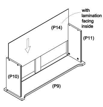
Slide the drawer base (P14) into the grooves of the drawer sides (P10 & P11) and the drawer front (P9).
