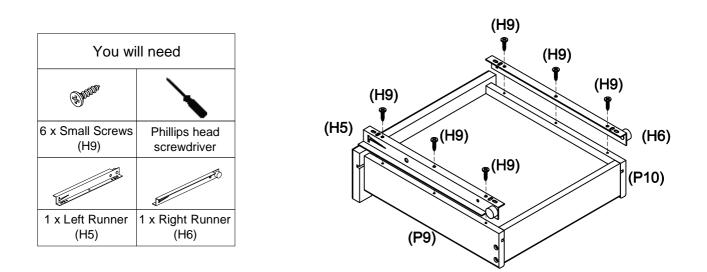
Fix the left runner (H5) to the left drawer side (P9) and right runner (H6) to the right drawer side (P10) with 6 x small screws (H9) by tightening with the phillips head screwdriver.
