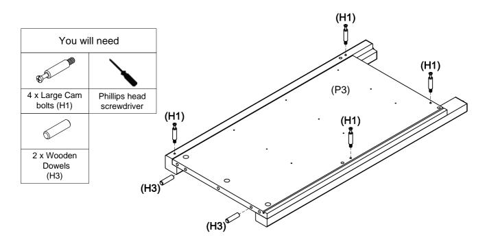
Fix 4 x large cam bolts (H1) to the right side panel (P3) by tightening with a phillips head screwdriver.
