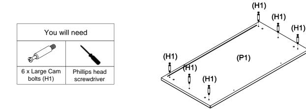
Fix 6 x large cam bolts (H1) to the top panel (P1) by tightening with a phillips head screwdriver.
