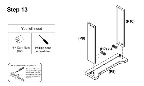
Insert 4 x cam nuts (H2) into the left and right drawer sides (P9, P10), rotate the cam nuts (H2) so the arrow is pointing towards the incoming cam bolt (H1).
