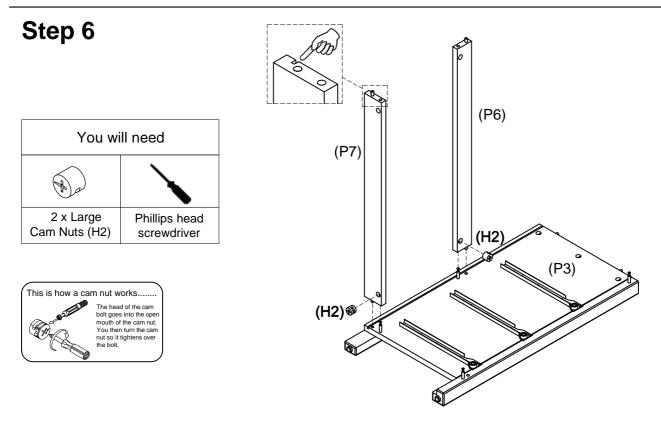
Insert large cam nuts (H2) into the back support rails (P6, P7). Rotate the cam nuts (H2) so the arrow is pointing towards the incoming cam bolt (H1).
