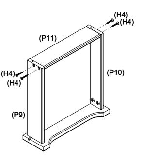
Use 4 x large screws (H4) to fix the drawer back (P11) to the drawer sides (P9, P10), by tightening with the phillips head screwdriver.
