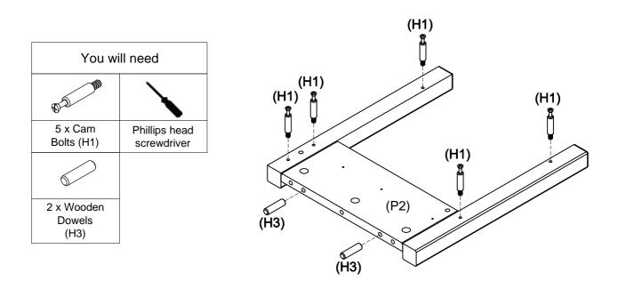
Fix 5 x cam bolts (H1) to the left side panel (P2) by tightening with a phillips head screwdriver.
