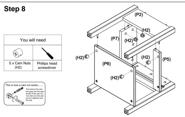
Insert cam nuts (H2) into front rail (P5), shelf (P6) and back panel (P7). Rotate the cam nuts (H2) so the arrow is pointing towards the incoming cam bolt (H1).
