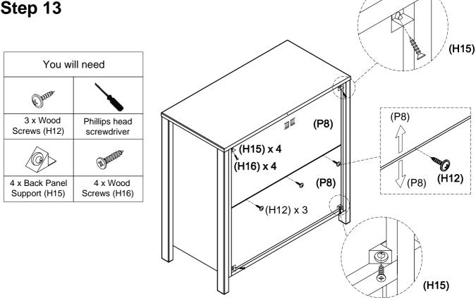
Fix the back panels (P8) to back support rail (P6) with 3 x wood screws (H12) by tightening with a phillips head screwdriver.
