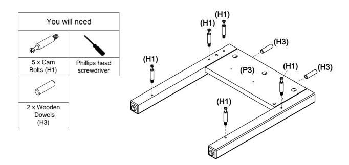
Fix 5 x cam bolts (H1) to the right side panel (P3) by tightening with a phillips head screwdriver.
