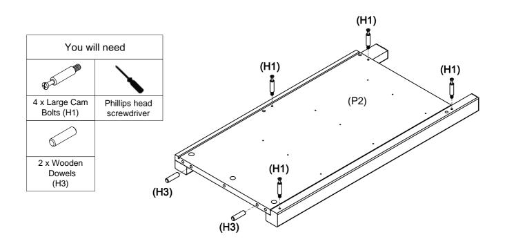
Fix 4 x large cam bolts (H1) to the left side panel (P2) by tightening with a phillips head screwdriver.
