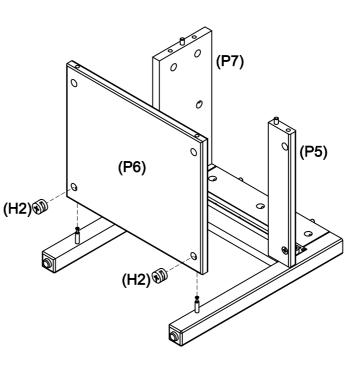
Insert 2 x cam nuts (H2) into the shelf (P6). Rotate the cam nuts (H2) so the arrow is pointing towards the incoming cam bolt (H1).
