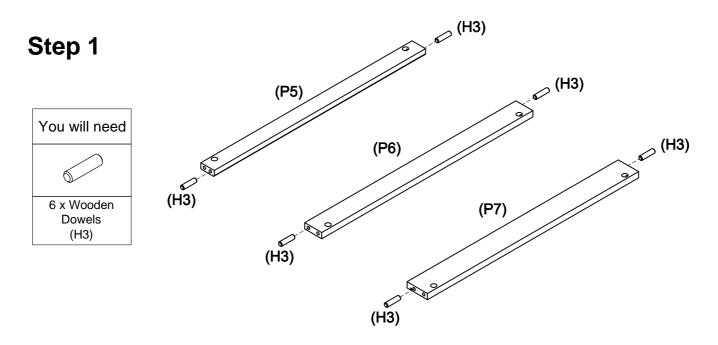
Insert 2 x wooden dowels (H3) into the front rail (P5). Insert 2 x wooden dowels (H3) into the middle back support rail (P6). Insert 2 x wooden dowels (H3) into the bottom back support rail (P7).
