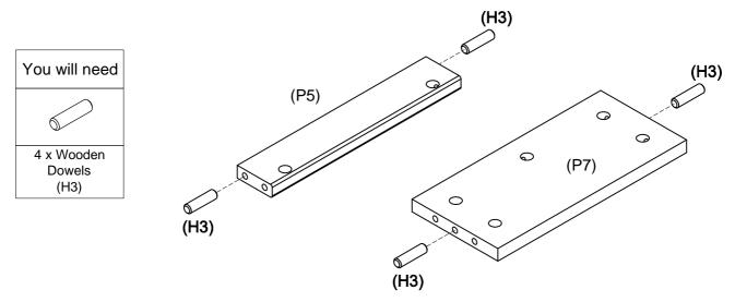
Insert 2 x wooden dowels (H3) into the front rail (P5). Insert 2 x wooden dowels (H3) into the back panel (P7).
