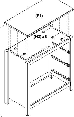
Insert large cam nuts (H2) into the left side panel (P2) and right side panel (P3). Rotate the cam nuts (H2) so the arrow is pointing towards the incoming cam bolt (H1). To fix the left side panel (P2) and right side panel (P3) to the top panel (P1), use the phillips head screwdriver to tighten the cam nuts (H2).
