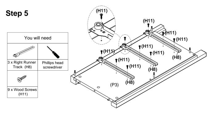
Fix 3 x right runner tracks (H8) to the right side panel (P3) with 9 x woodscrews (H11) into the pre-drilled holes by tightening with a phillips head screwdriver.
