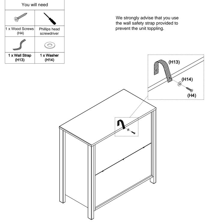
Fix the wall strap (H13) to the back of the top panel (P1) with a wood screw (H4) and sasher (H14) by tightening with the phillips head screwdriver. Seek professional advice for how to attach the other end of the wall strap to your wall.
