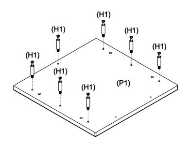
Fix 7 x cam bolts (H1) to the top panel (P1) by tightening with a phillips head screwdriver.
