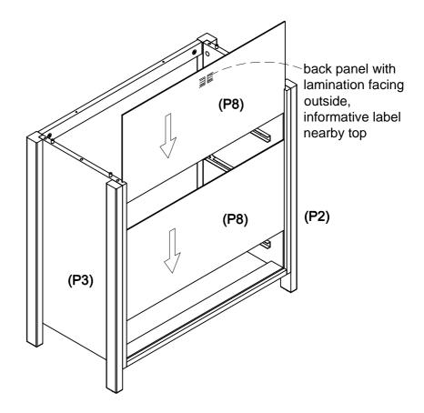
Turn the unit upright carefully, slip 2 x back panels (P8) into the grooves on the side panels (P2) & (P3).
