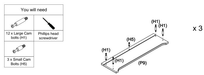
Fix 4 x large cam bolts (H1) and 1 x small cam bolts (H5) to the drawer front panel (P9) by tightening with a phillips head screwdriver.
