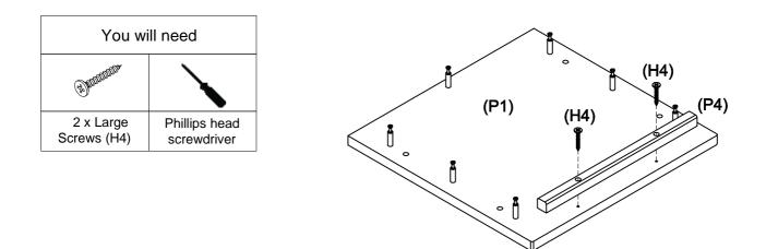
Fix the top panel rail (P4) to the top panel (P1) with 2 x large screws (H4) by tightening with a phillips head screwdriver.
