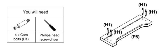
Fix 4 x cam bolts (H1) to the drawer front panel (P8) by tightening with a phillips head screwdriver.
