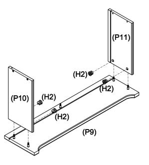
Insert large cam nuts (H2) into the left and right drawer sides (P10 & P11), rotate the large cam nuts (H2) so the arrow is pointing towards the incoming cam bolt (H1).
