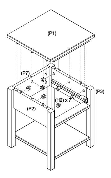
Insert cam nuts (H2) into the left side panel (P2), the right side panel (P3) and the back panel (P7). Rotate the cam nuts (H2) so the arrow is pointing towards the incoming cam bolt (H1). To fix the left side panel (P2), the right side panel (P3) and the back panel (P7) to the top panel (P1), use the phillips head screwdriver to tighten the cam nuts (H2).
