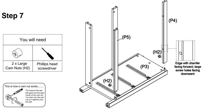
Insert large cam nuts (H2) into the top panel rail (P4) and the front rail (P5). Rotate the cam nuts (H2) so the arrow is pointing towards the incoming cam bolt (H1). To fix the top panel rail (P4) and front rail (P5) to the right side panel (P3), use the phillips head screwdriver to tighten the cam nuts (H2).
