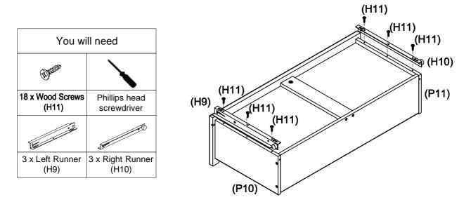
Fix the left runner (H9) to the left drawer side (P10) and the right runner (H10) to the right drawer side (P11) with wood screws (H11) by tightening with the phillips head screwdriver. Repeat steps for the other two drawers.
