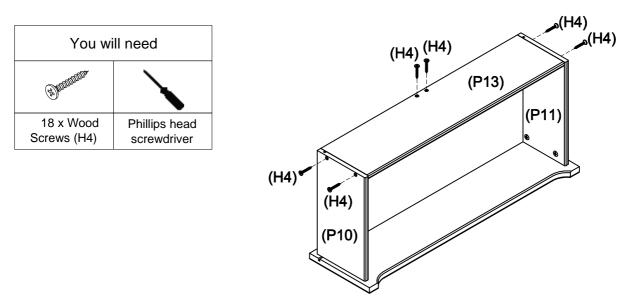
Use wood screws (H4) to fix the drawer back (P13) to drawer sides (P10 & P11) and the drawer support rail (P12) , by tightening with the phillips head screwdriver. Repeat steps for the other two drawers.
