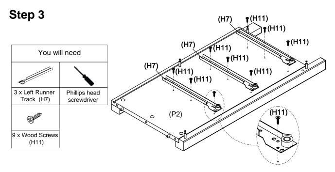
Fix 3 x left runner tracks (H7) to the left side panel (P2) with 9 x wood screws (H11) into the pre-drilled holes by tightening with a phillips head screwdriver.
