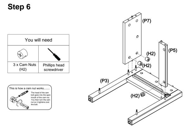
Insert cam nuts (H2) into the front rail (P5) and back panel (P7). Rotate the cam nuts (H2) so the arrow is pointing towards the incoming cam bolt (H1).
