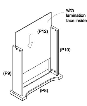
Slide the drawer base (P12) into the grooves of the left and right drawer sides (P9, P10) and the drawer front (P8).
