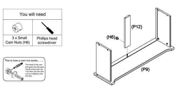
Insert small cam nuts (H6) into the drawer support rail (P12), rotate the small cam nuts (H6) so the arrow is pointing towards the incoming cam bolt (H5). To secure the drawer support rail (P12) to the drawer front (P9), use the phillips head screwdriver to tighten the small cam nuts (H6). Repeat steps for the other two drawers.
