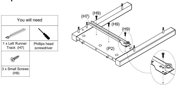
Fix the left runner track (H7) to the left side panel (P2) with 3 x small screws (H9) by tightening with a phillips head screwdriver.
