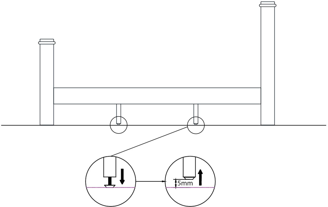
The rest position of adjustable support is 5mm above the floor .
