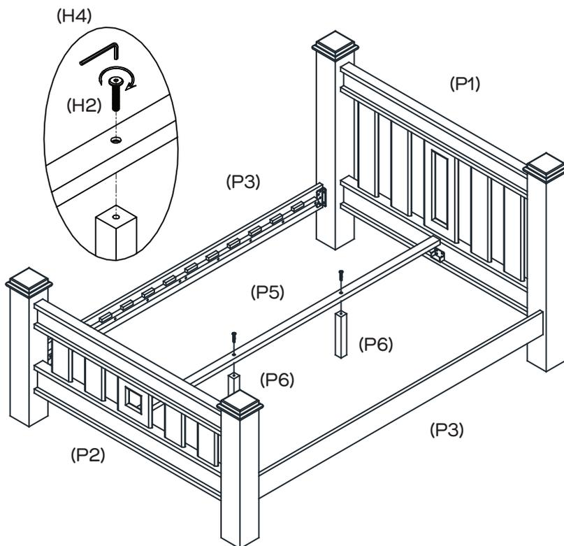
Attach Supports (P6) to Crossbar (P5) with 2 x Long Bolts (H2).
