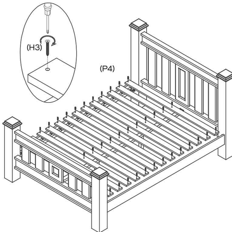
Attach Slats (P4) to Assembled Bed with 39 x Long Screws (H3).
