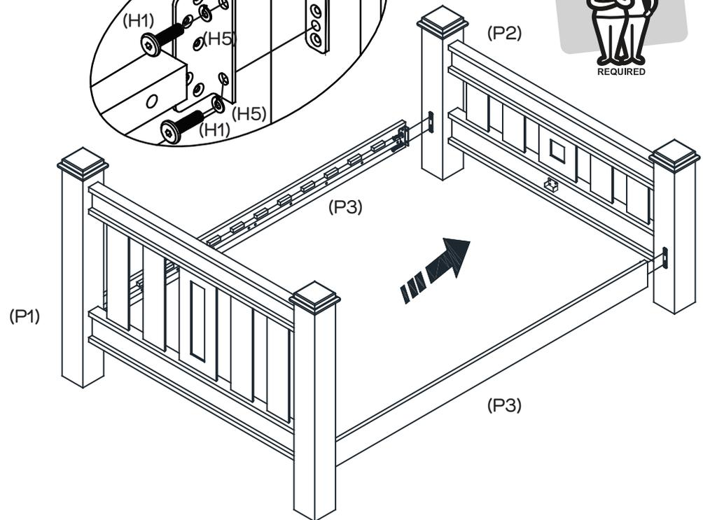
Attach Side Rails (P3) to Footboard (P2) with 4 x Short Bolts (H1) And 4 x Spring Washers (H5) . Tighten Bolts loosely with an Allen Key (H4). Now check and tighten all (H1) Bolts firmly.
