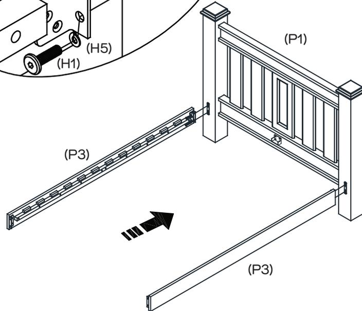
Attach Side Rails (P3) to Headboard (P1) with 4 x Short Bolts (H1) And 4 x Spring Washers (H5). Tighten Bolts loosely with an Allen Key (H4) .
