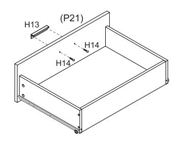
Attach 1 x Handle (H13) to Larger Drawer Front (P21) with 2 x Round Head Bolts (H14). Tighten Round Head Bolts using a Phillips head screwdriver.
