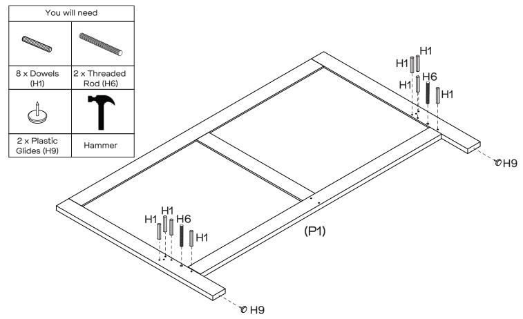
Insert 8 x Dowels (H1) into Bedhead (P1). Attach 2 x Threaded Rod (H6) into Bedhead (P1). Hammer 2 x Plastic Glides (H9) onto the bottom of Bedhead (P1).
