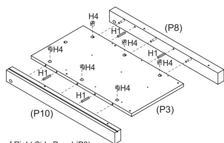
Insert 4 x Dowels (H1) into the holes of Right Side Panel (P3).
