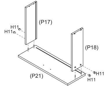
Insert 4 x Small Cam Nuts (H11) into the holes of Drawer Sides (P17, P18). Rotate the cam nuts so the arrows point towards the incoming cam bolts. Attach Drawer Sides (P17, P18) with Larger Drawer Front (P21), and then tighten the cam nuts.
