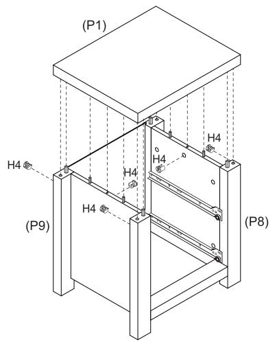
Insert 6 x Cam Nuts (H4) into the holes of Side Panels (P2, P3) and Legs (P7, P8, P9, P10). Rotate the cam nuts so the arrows point towards the incoming cam bolts. Attach Top Panel (P1) to the frame and tighten the cam nuts using a Flat head screwdriver.
