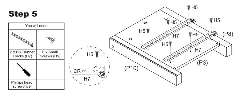
Attach 2 x CR Runner Tracks (H7) to Right Side Panel (P3) with 6 x Small Screws (H5).
