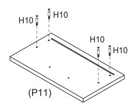
Screw 4 x Small Cam Bolts (H10) into Drawer Front (P11) with a Phillips head screwdriver.
