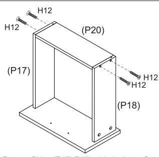
Attach Smaller Drawer Back (P20) to Drawer Sides (P17, P19) with 4 x Long Screws (H12), make sure that the grooves line up the whole way around the drawer. Tighten Screws using a Phillips head screwdriver.
