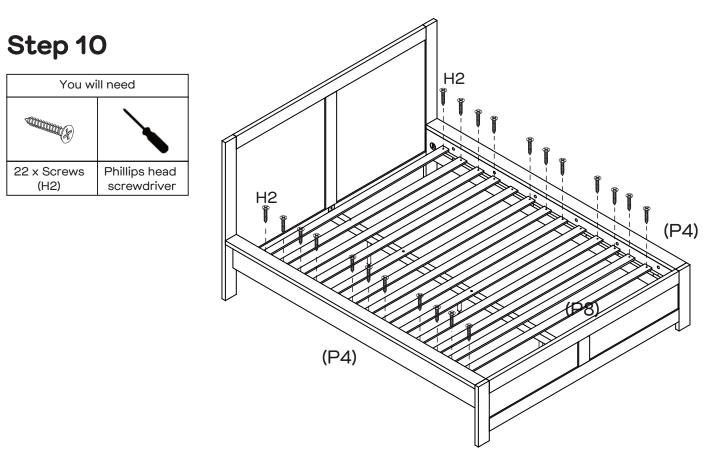
Attach Article bed boards (P8x11) to Side Rails (P4) with 22 x Screws (H2). Tighten with a Phillips head screwdriver.
