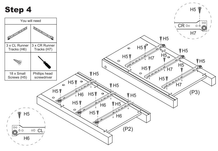
Attach 3 x CL Runner Tracks (H6) to Left Side Panel (P2) with 9 x Small Screws (H5). Attach 3 x CR Runner Tracks (H7) to Right Side Panel (P3) with 9 x Small Screws (H5).
