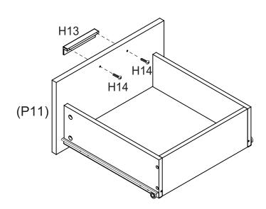
Attach 1 x Handle (H13) to Drawer Front (P11) with 2 x Round Head Bolts (H14). Tighten round head bolts using a Phillips head screwdriver. Repeat Step 14 to Step 19 to assemble the other drawer.
