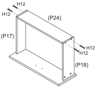
Attach Larger Drawer Back (P24) to Drawer Sides (P17, P18) with 4 x Long Screws (H12), make sure that the grooves line up the whole way around the drawer. Tighten Screws using a Phillips head screwdriver.
