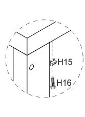
Secure Back Panel (P6) in place with 4 x Wedges (H15) using 4 x Screws (H16). www.fantasticfurniture.com.au
