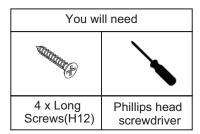
Attach Drawer Back (P15) to Drawer Sides (P12, P13) with 4 x Long Screws (H12), make sure that the groove lines up the whole way around the drawer. Tighten Screws using a Phillips head screwdriver.
