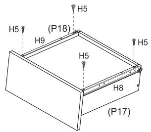
Attach 1 x DL Runner (H8) to the bottom of Left Drawer Side (P17) and 1 x DR Runner (H9) to the bottom of Right Drawer Side (P18) with 4 x Small Screws (H5). Tighten Screws using a Phillips head screwdriver.
