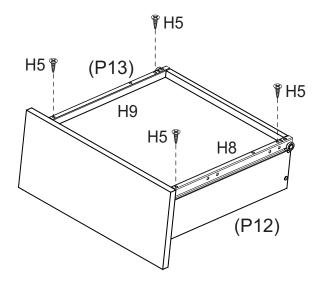
Attach 1 x DL Runner (H8) to the bottom of Left Drawer Side (P12) and 1 x DR Runner (H9) to the bottom of Right Drawer Side (P13) with 4 x Small Screws (H5). Tighten Screws using a Phillips head screwdriver.
