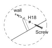
Move the dresser to the final position, and attach the safety strap to the wall securely. Make sure it is firmly attached and snug fit.
