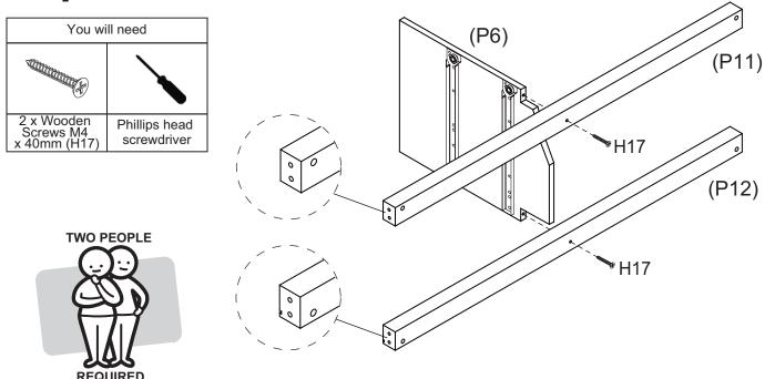
Attach Rails (P11, P12) to Divider (P6) with 2 x Wooden Screws (H17) using a Phillips head screwdriver.
