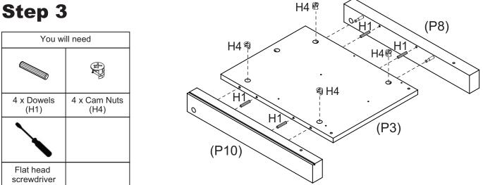
Insert 4 x Dowels (H1) into the holes of Right Side Panel (P3). Insert 4 x Cam Nuts (H4) into the holes of Right Side Panel (P3). Rotate the cam nuts so the arrows point towards the incoming cam bolts. Attach Legs (P8, P10) to Right Side Panel (P3), then tighten the cam nuts. www.fantasticfurniture.com.au
