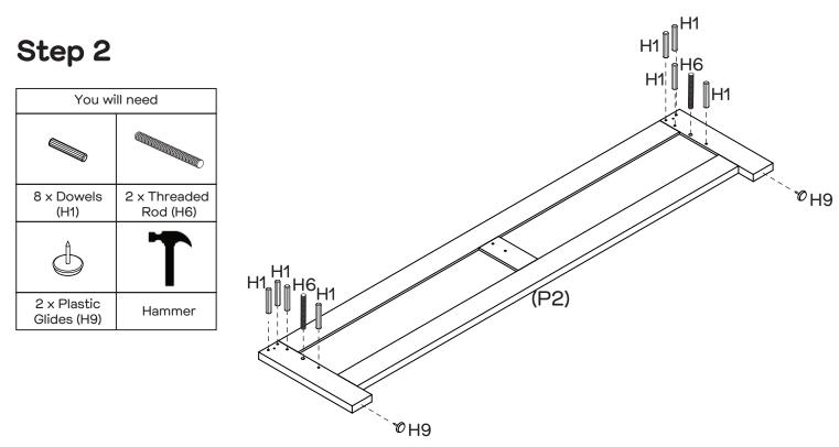
Insert 8 x Dowels (H1) into Bedfoot (P2). Attach 2 x Threaded Rod (H6) into Bedfoot (P2). Hammer 2 x Plastic Glides (H9) onto the bottom of Bedfoot (P2).
