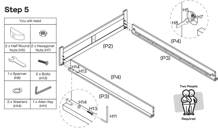
Attach Bedfoot (P2) to Side Covers (P3) and Side Rails (P4) with 2 x Half Round Nuts (H5), and 2 x Hexagonal Nuts (H7) using a Spanner (H8). Connect the brackets to Bedfoot (P2) with 2 x Bolts (H13) and 2 x Washers (H14) using an Allen Key (H11). Do not fully tighten the bolts until Step 6.
