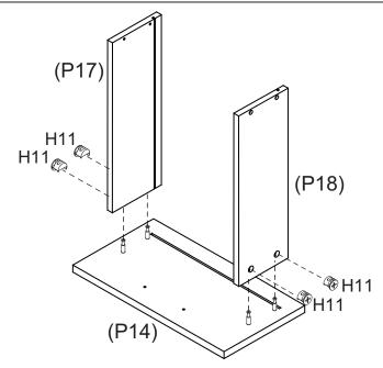
Insert 4 x Small Cam Nuts (H11) into the holes of Drawer Sides (P17, P18). Rotate the cam nuts so the arrows point towards the incoming cam bolts. Attach Drawer Sides (P17, P18) with Smaller Dawer Front (P14), and then tighten the cam nuts.
