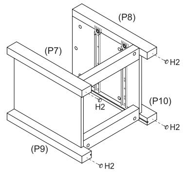
Attach 4 x Plastic Glides (H2) to the bottom of Legs (P7, P8, P9, P10) with a Hammer.
