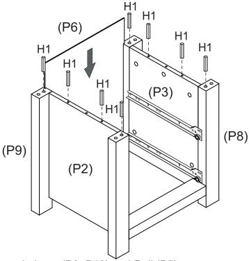
Slide Back Panel (P6) into the groove in Legs (P9, P10) and Rail (P5). Insert 8 x Dowels (H1) into Side Panels (P2, P3) and Legs (P7, P8, P9, P10).
