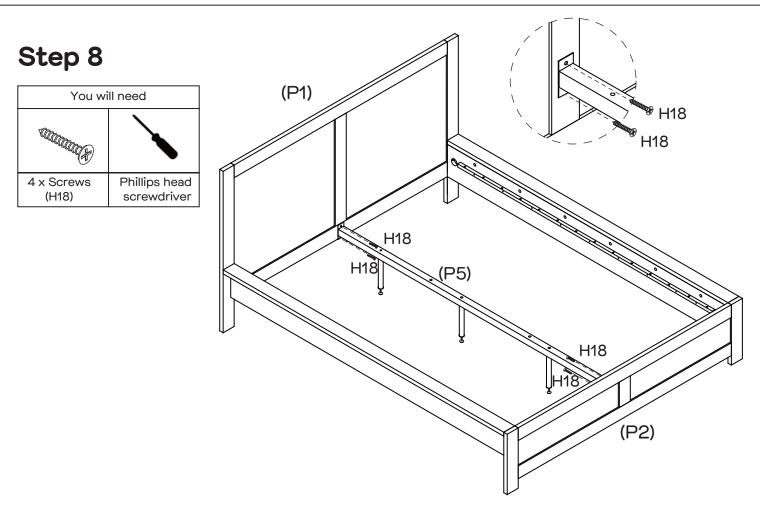
Attach Centre Rail (P5) to Bedhead (P1) and Bedfoot (P2) screw with  $4\times$  Screws (H18). Tighten with a Phillips Head Screwdriver.
