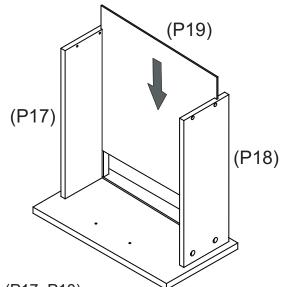
Slide Smaller Drawer Base (P19) in through the grooves of Drawer Sides (P17, P18).
