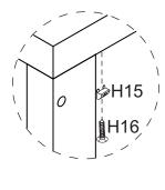
Secure Back Panel (P13) in place with 4 x Wedges (H15) using 4 x Screws (H16).
