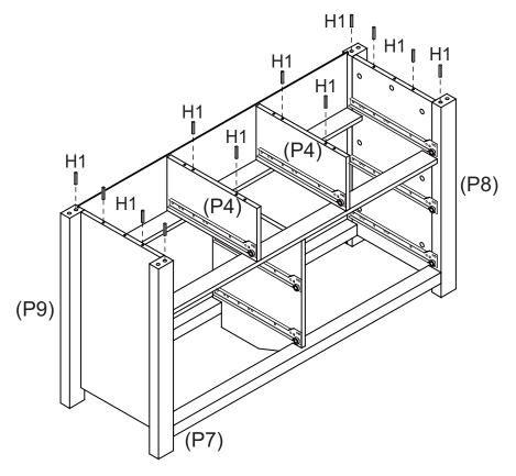
Insert 12 x Dowels (H1) into Side Panels (P2, P3), Dividers (P4) and Legs (P7, P8, P9, P10) as shown.
