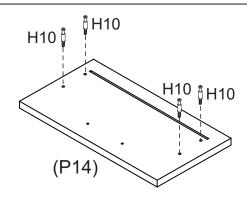
Screw 4 x Small Cam Bolts (H10) into Smaller Drawer Front (P14) with a Phillips head screwdriver.
