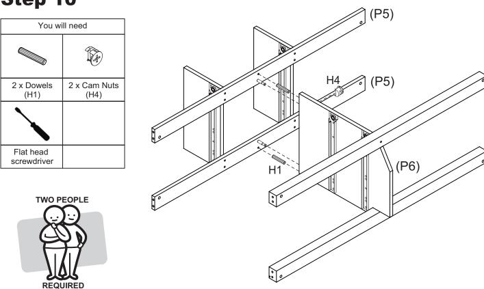
Insert 2 x Dowels (H1) into the holes of Rails (P5).
