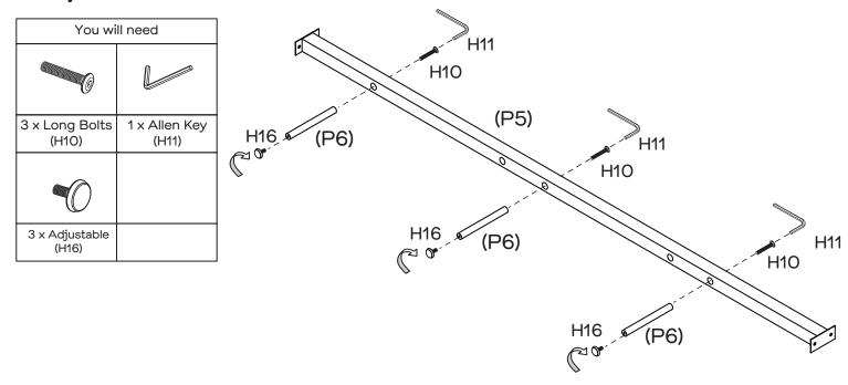
Attach 3 x Support Legs (P6) to Centre Rail (P5) with 3 x Long Bolts (H10) using Allen Key (H11). Insert the  $3 \times Adjustable$  (H16) into the Support Legs (P6).
