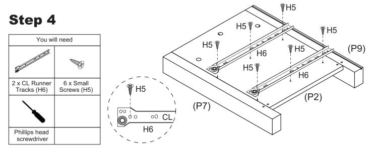
Attach 2 x CL Runner Tracks (H6) to Left Side Panel (P2) with 6 x Small Screws (H5).
