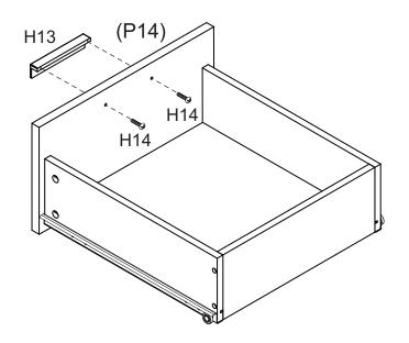
Attach 1 x Handle (H13) to Smaller Drawer Front (P14) with 2 x Round Head Bolts (H14). Tighten Round Head Bolts using a Phillips head screwdriver.
