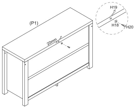
Use Screw (H20) and Washer (H18) to attach Safety Strap (H19) securely on Top Panel (P1) as shown. www.fantasticfurniture.com.au
