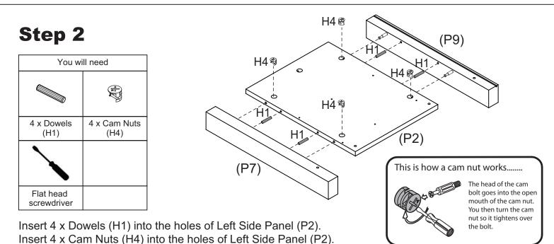
Attach Legs (P7, P9) to Left Side Panel (P2), then tighten the cam nuts.
