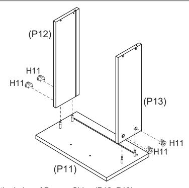
Insert 4 x Small Cam Nuts (H11) into the holes of Drawer Sides (P12, P13). Rotate the cam nuts so the arrows point towards the incoming cam bolts. Align the holes together, secure Drawer Sides (P12, P13) into place and tighten the cam nuts using a Flat head screwdriver.
