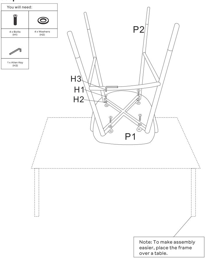
Align holes on seat (P1) with holes on metal frame (P2). Attach seat (P1) to metal frame (P2) using 4 x bolts (H1) and 4 x washers (H2). Apply downward pressure on the metal frame (P2) to secure the bolts (H1) into the pre-drilled holes and hand-tighten by turning the bolts (H1) clockwise. Once the bolts (H1) are secure, use the allen key (H3) to firmly tighten the bolts (H1).
