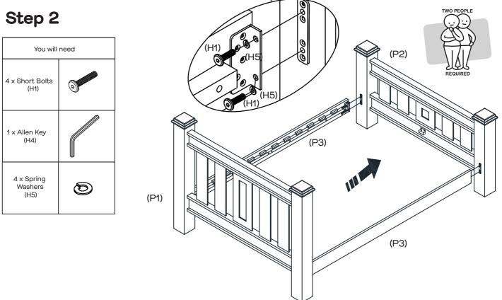
Attach Side Rails (P3) to Footboard (P2) with 4 x Short Bolts (H1) And 4 x Spring Washers (H5) . Tighten Bolts loosely with an Allen Key (H4).
