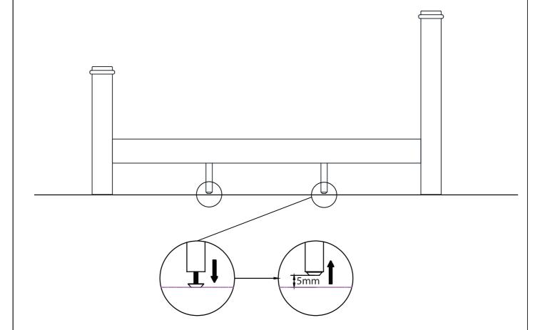
The rest position of adjustable support is 5mm above the
