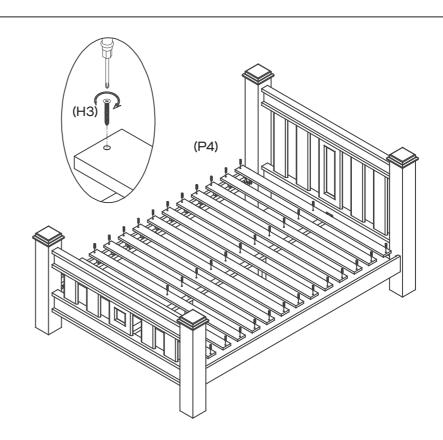
Attach Slats (P4) to Assembled Bed with  $39 \times Long$  Screws (H3). Tighten Long Screws using a Phillips Head Screwdriver .
