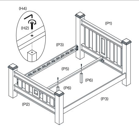
Attach Supports (P6) to Crossbar (P5) with 2 x Long Bolts (H2). Tighten Bolts with an Allen key (H4). Insert Crossbar (P5) into Assembled Bed.
