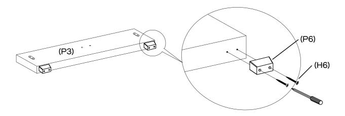
Attach 2 x footboard legs (P6) to the bottom of footboard (P3) with  $4 \times 1$  large screw 51mm (H6) by using phillips head screwdriver (not provided).
