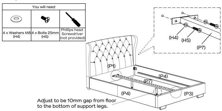
Slot the centre rail (P7) into the headboard (P1) and footboard (P3). Rotate bolts (H5) by using phillips head screwdriver (not provided) to the headboard (P1) and footboard (P3). No need to tighten bolts until step 8.
