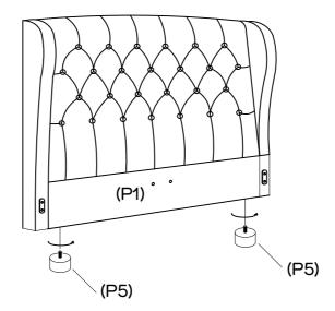
Attach 2 x headboard legs (P5) to the bottom of headboard (P1) as shown.
