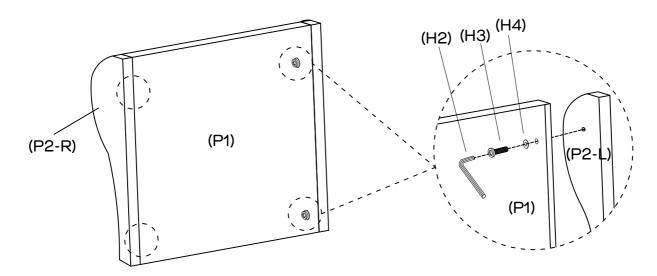
Attach wings (P2-L; P2-R) to the headboard (P1) with 4 x washers (H4) and 4 x bolts 45mm (H3) by using allen key (H2) as shown.
