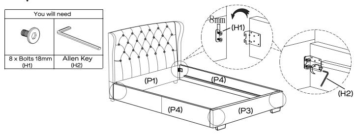
Install the bolts (H1) to the brackets by using allen key (H2) as shown, do not tighten the bolts and keep them 8mm loose. Then attach 2 x side rails (P4) to headboard (P1) and footboard (P3) by slotting the bracket on the side rails (P4) over the bolt as shown. No need to tighten bolts until step 8.
