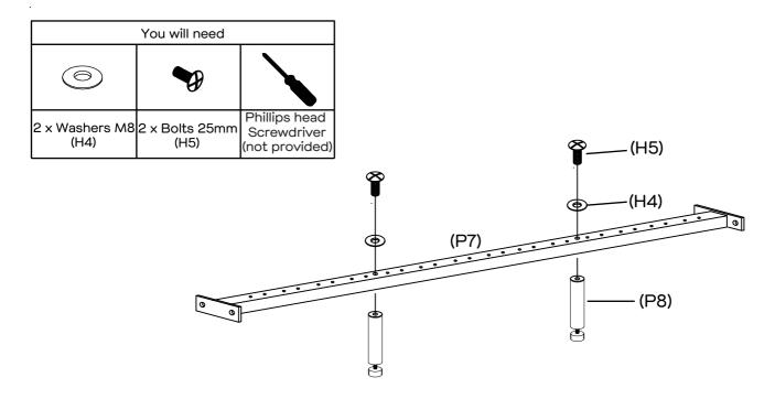
Attach 2 x support legs (P8) to the centre rail (P7) using  $2 \times 10^{-2}$  x bolts (H5) and  $2 \times 10^{-2}$  as shown.
