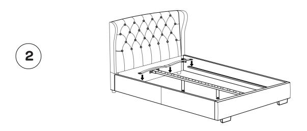
Insert the full slat into the side rail and centre rail one by one.
