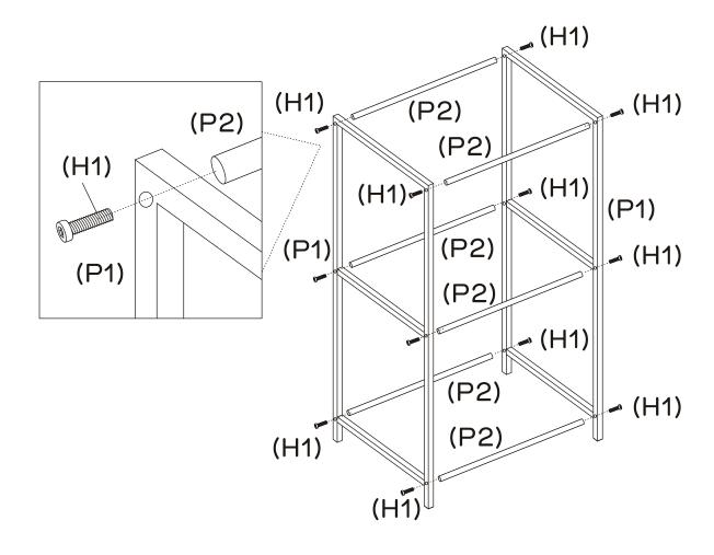
Attach Frame Bars (P2x6) to Frame (P1x1) with 6 x Bolts (H1) by tightening with the Allen Key (H2).
