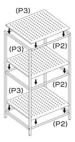
Attach Shelves (P3x3) to Frame Bars (P2x3) by firmly pushing down. Ensuring Shelves (P3x3) are clipped in correctly and firmly attached.
