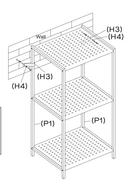
Attach 2x Wall Straps (H3) to the top of Frame (P1x2), as shown. Connect the 2 x Wall Straps (H3) to the wall. Make sure it is firmly attached and a snug fit.
