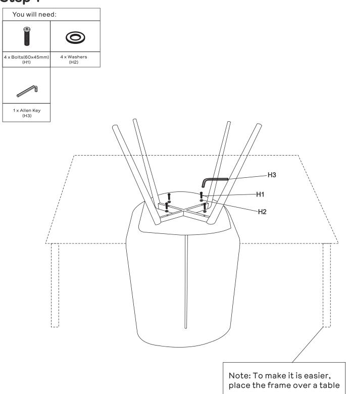
Align seat (P2) with holes in Metal Frame (P1). Attach seat(P2) to Metal Frame(P1) with 4xBolts(H1) and 4xWashers(H2). You may need to apply downward pressure to get the bolts to catch. Once all bolts are hand-tightened, use Allen Key(H3) to tighten firmly.
